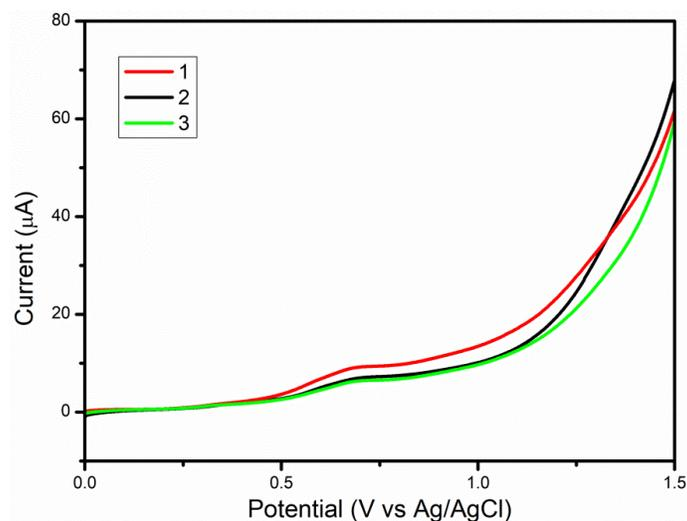
Figure S13: LSV of the rGO-CM coated on different GCEs
