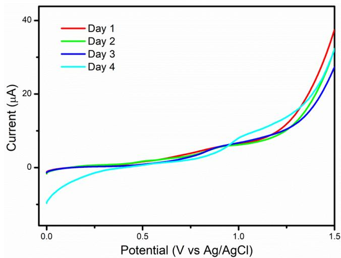
Figure S12: Stability of the rGO-CM/GCE sensor performance towards dioxane detection on different days
