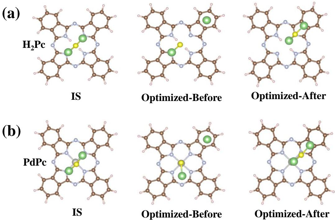
Fig. S3. The stable structures (IS), decomposed  $\text{Li}_2\text{S}$  adsorption structures before and after optimization of the (a)  $\text{H}_2\text{Pc}$ - $\text{Li}_2\text{S}$  and (b)  $\text{PdPc}$ - $\text{Li}_2\text{S}$  systems.
