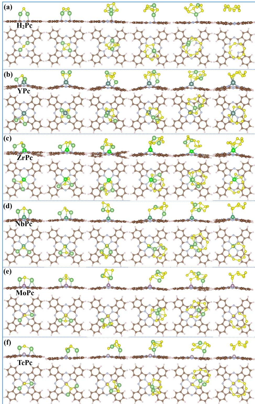
Fig. S1. (a)-(f) are the fully relaxed lowest-energy binding configurations of  $S_8/Li_2S_x$  ( $x = 1, 2, 4, 6, 8$ ) adsorbed on  $H_2Pc/TMPc$  (TM = Y, Zr, Nb, Mo, Tc) substrates. Here, the top view and side view are given, respectively.
