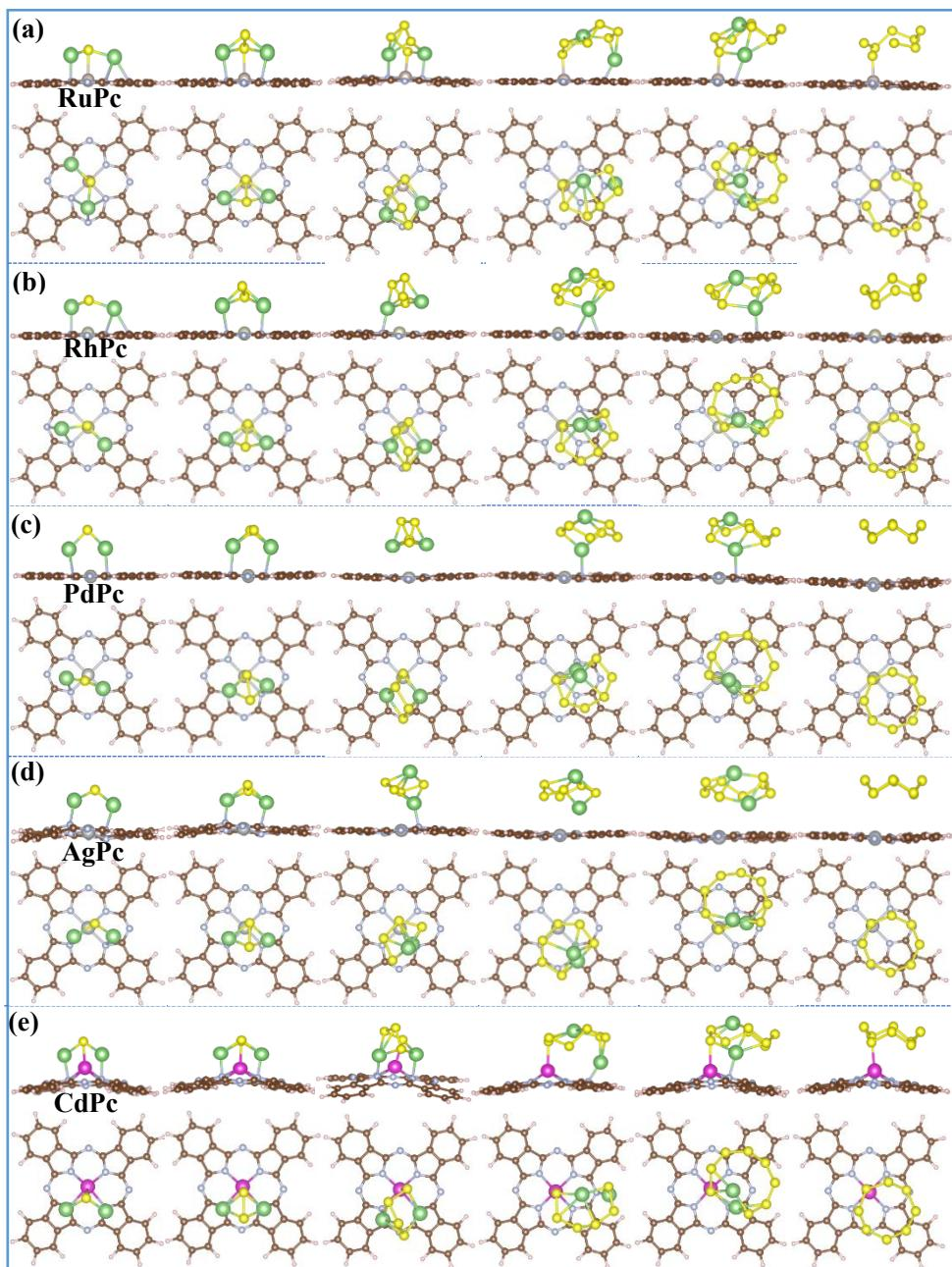
Fig. S2. (a)-(e) are the fully relaxed lowest-energy binding configurations of  $S_8/Li_2S_x$  ( $x = 1, 2, 4, 6, 8$ ) adsorbed on  $H_2Pc/TMPc$  ( $TM = Tc, Ru, Pd, Ag, Cd$ ) substrates. Here, the top view and side view are given, respectively.
