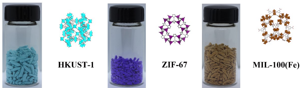
Fig. S1. Digital images of HKUST-1/RWR composite, ZIF-67/RWR composite and MIL-100(Fe)/RWR composite
