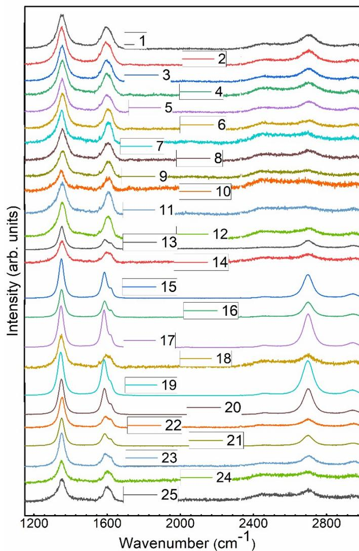
Fig. S1. Typical Raman spectra of the all studied samples. Samples' synthesis conditions can be found in Table 1.
