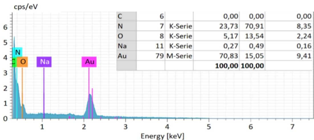
**Fig. S6** EDS data of  $g\text{-C}_3\text{N}_4\text{-}^t\text{BuONa}$ .
