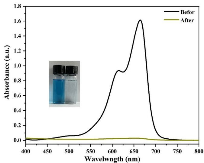
**Fig. S5** UV-Vis absorption spectra of MB dye for PAN/g-C<sub>3</sub>N<sub>4</sub>-*t*BuONa photocatalytic degradation (inset: the visual pictures of MB solution under illumination at 0 min and 180 min).
