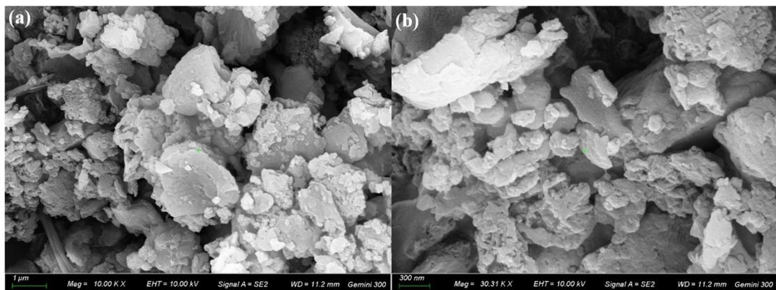
**Fig. S3** SEM image of  $g\text{-C}_3\text{N}_4\text{-EtONa}$
