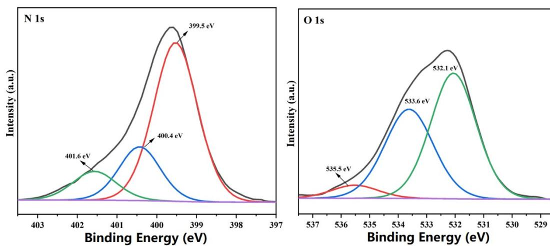
**Fig. S4** N 1s and O 1s core-level spectra of PAN/g-C<sub>3</sub>N<sub>4</sub>-*t*BuONa.
