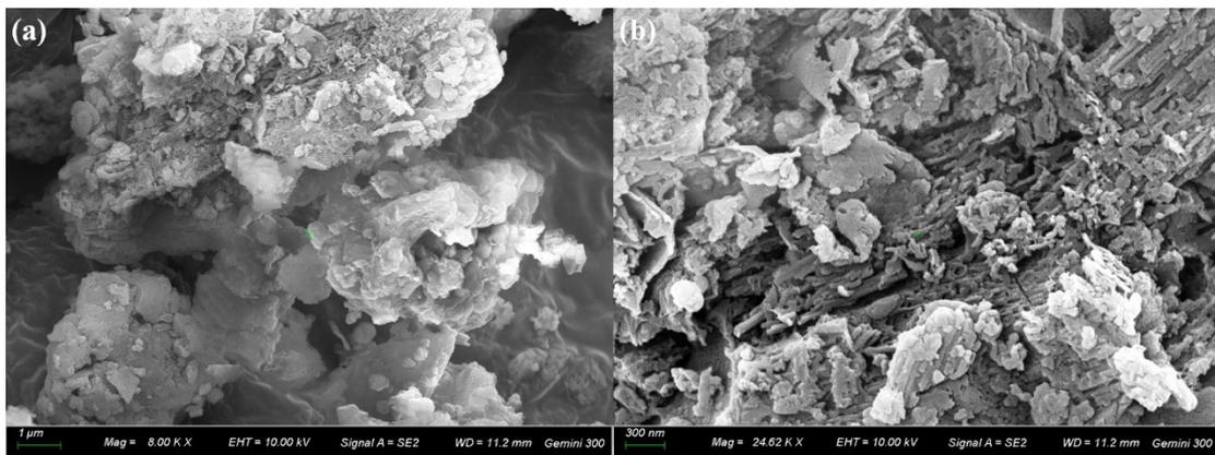
**Fig. S2** SEM image of  $g\text{-C}_3\text{N}_4\text{-MeONa}$
