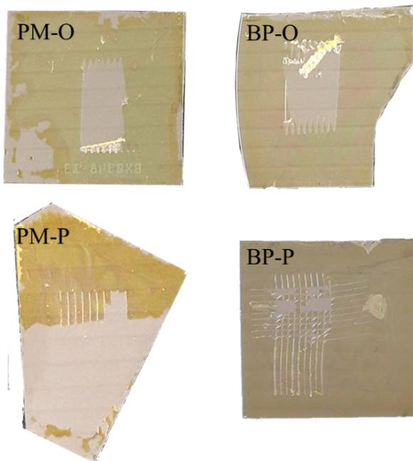
Fig. S1 Photos of a series of PI coatings on SiC after cross-cut adhesion tests.
