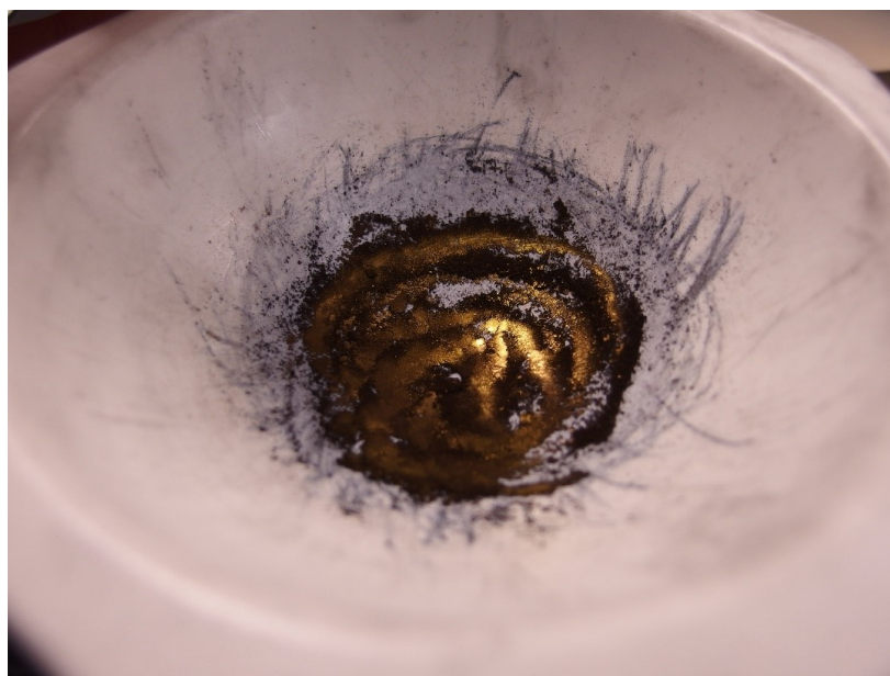
Fig. S1. Photographic image showing the development of a gold tone upon the grinding of a blackish brown 3-methoxythiophene oligomer powder in a mortar.
