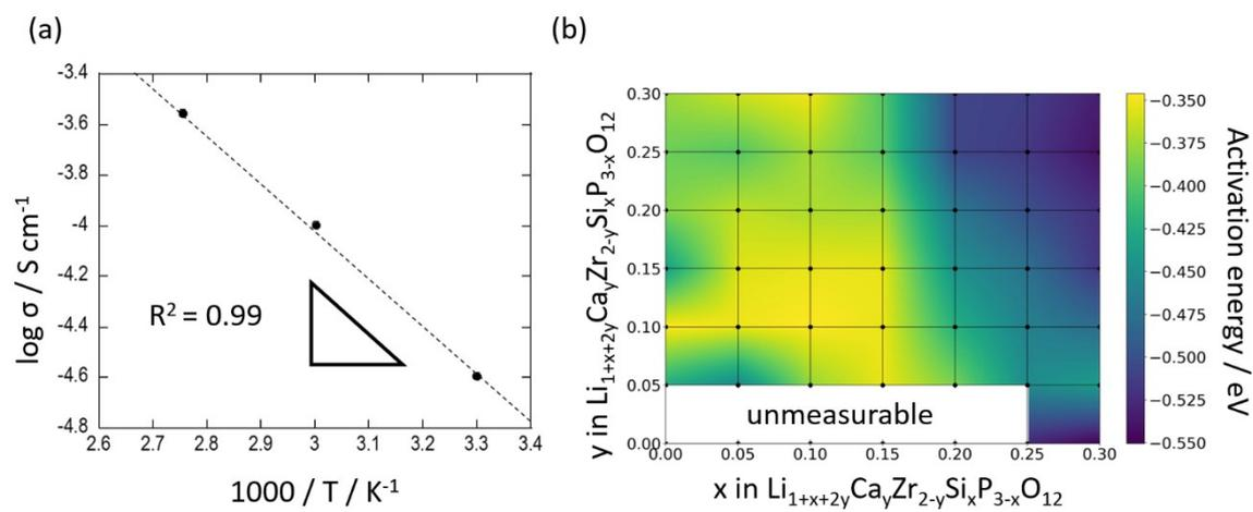
**Fig. S2** (a) Arrhenius plot of the Li-ion conductivity of  $\text{Si}_{0.1}/\text{Ca}_{0.05}$ . (b) Composition dependence of the activation energy for the as-synthesised  $\text{Si}_x/\text{Ca}_y$  pellets.
