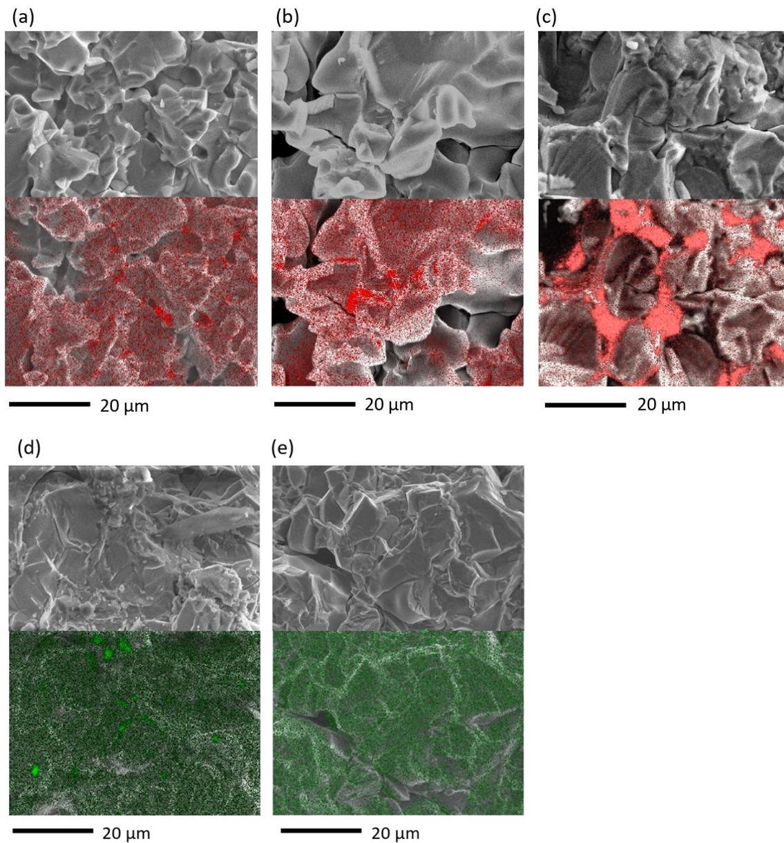
**Fig. S1** EDX elemental maps of calcium (red) and silicon (green) in the fracture surfaces of (a)  $\text{Si}_{0.1}/\text{Ca}_{0.05}$ , (b)  $\text{Si}_{0.1}/\text{Ca}_{0.1}$ , (c)  $\text{Si}_{0.1}/\text{Ca}_{0.3}$ , (d)  $\text{Si}_{0.2}/\text{Ca}_{0.1}$ , and (e)  $\text{Si}_{0.3}/\text{Ca}_{0.1}$ .
