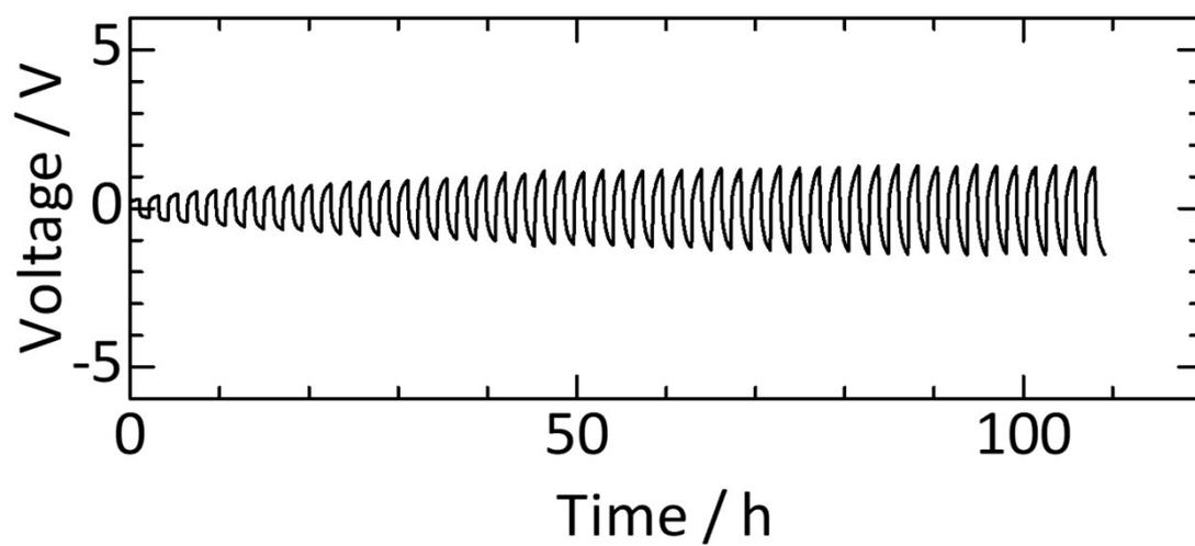
**Fig. S3** Galvanostatic cycle measurement of the Li | Li<sub>1.2</sub>Ca<sub>0.05</sub>Zr<sub>1.95</sub>Si<sub>0.1</sub>P<sub>2.9</sub>O<sub>12</sub> | Li symmetric cell over a period of 110 h at a current density of 50  $\mu\text{A cm}^{-2}$ .
