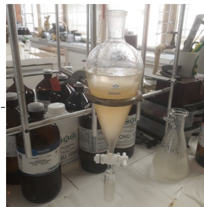
Neutralization with \text{Na}_2\text{CO}_3 (pH around 7-8) followed by the extraction with AcOEt
