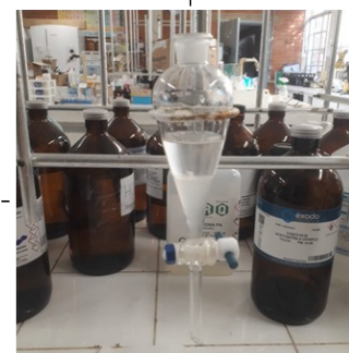
Liquid/liquid extraction followed by solvent removal under reduced pressure
