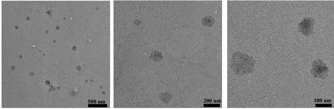
Fig. S5 The TEM images and f NOD-NP at different resolutions
