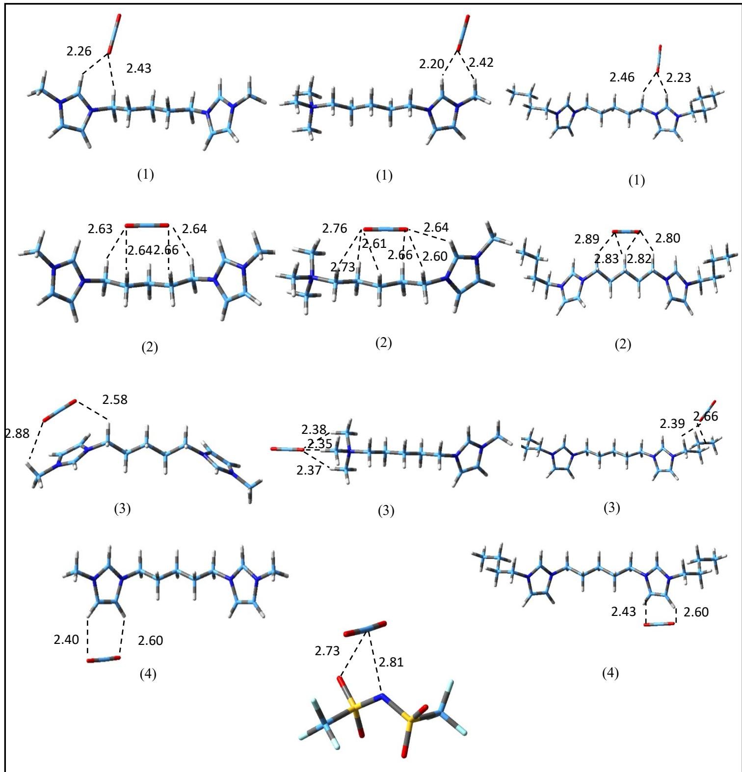
**Fig. S3.** Optimized structures of isolated ion- $\text{CO}_2$  complexes at the M06-2x/cc-pVDZ level of theory. The broken lines show the most important intermolecular interactions between  $\text{CO}_2$  molecule and isolated ions (distances are in  $\text{\AA}$ ).
