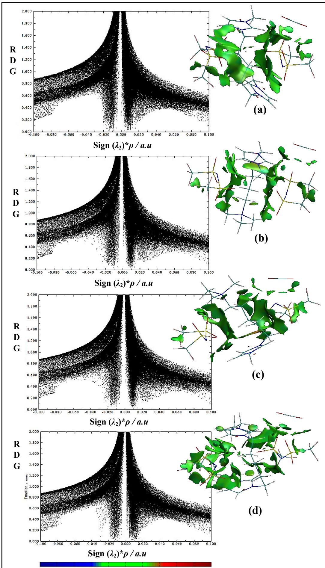
**Fig. S6.** Color-filled RDG isosurfaces and scatter graphs of RDG for DIL-CO<sub>2</sub> complexes. Green and red colors denote vdW interactions and steric contributions, respectively.
