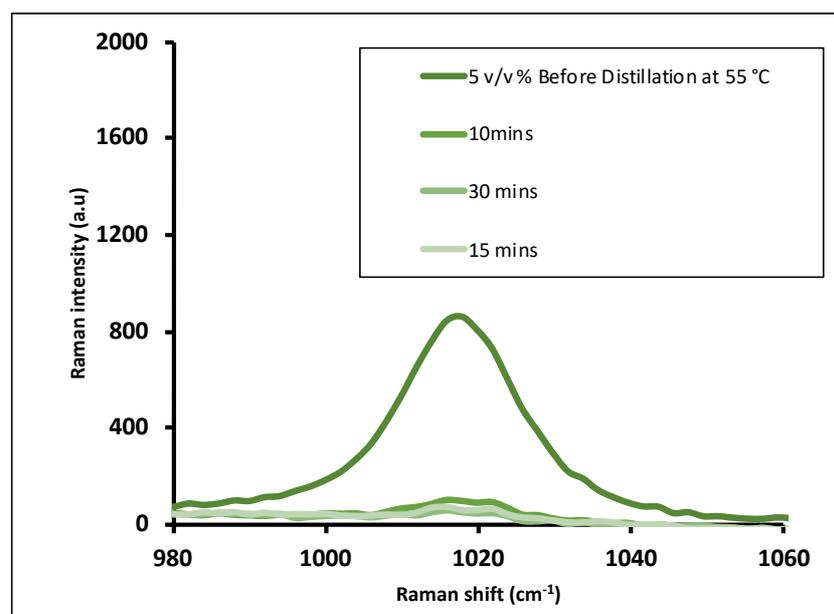
**Figure 3:** Raman spectra of 5 (v/v)% TMOS before distillation demonstrating concentration of methanol before and after distillation by rotary evaporation at 25 mbar and 55 °C for 10, 15 and 30 minutes.
