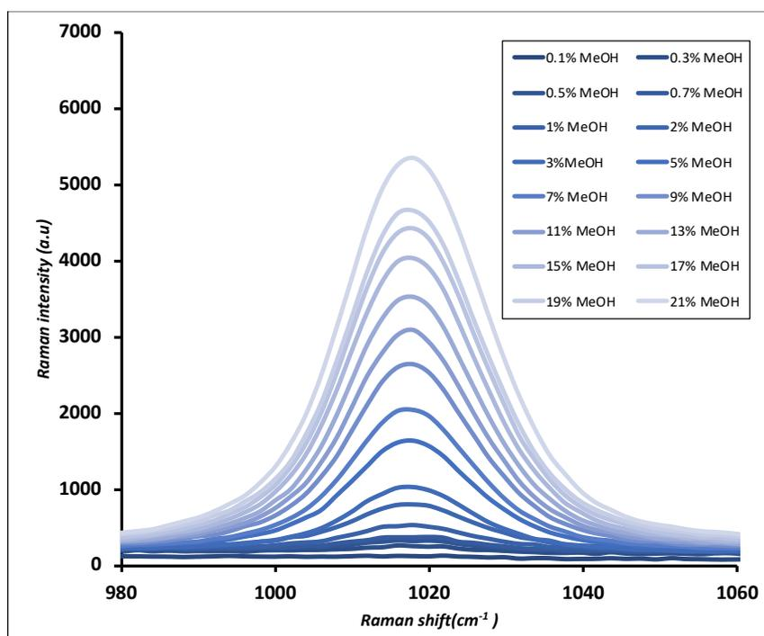
**Figure 1:** Calibration curve of Raman peak intensity vs aqueous methanol concentration (v/v %) (top) based on Raman spectra (bottom) at methanol concentrations from 0.1% to 21%.
