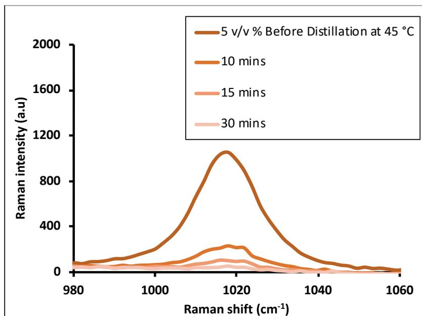
**Figure 2:** Raman spectra of 5 (v/v)% TMOS before distillation demonstrating concentration of methanol before and after distillation by rotary evaporation at 25 mbar and 45 °C for 10, 15 and 30 minutes.
