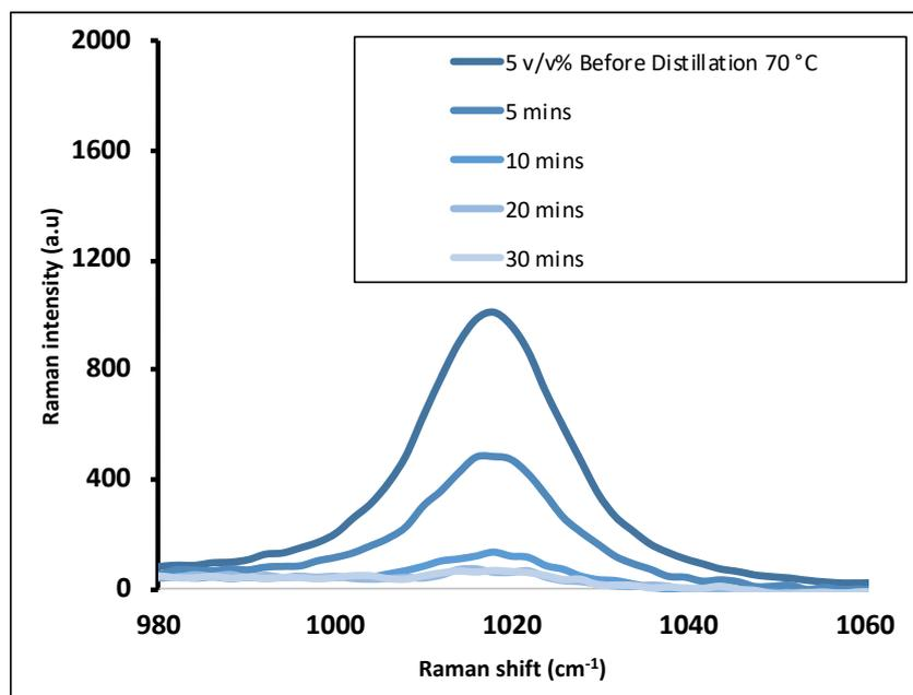
**Figure 4:** Raman spectra of 5 (v/v)% TMOS before distillation demonstrating concentration of methanol before and after distillation by rotary evaporation at 25 mbar and 70 °C after 10, 15 and 30 minutes.
