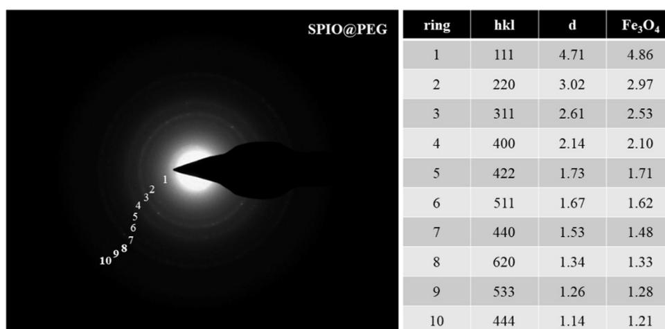
Figure S1. SAED patter of SPIO@PEG nanoparticles and Measured Lattice Spacing
