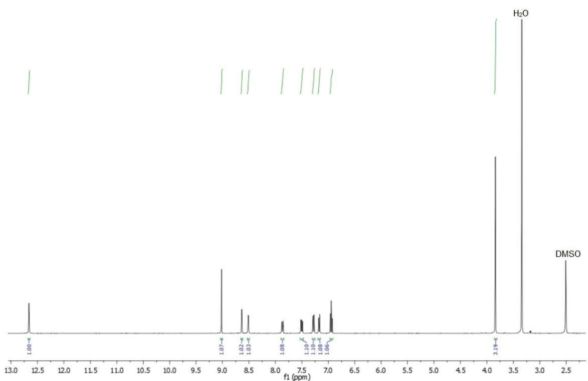
**Figure 7S.** <sup>1</sup>H NMR of **HL2** at room temperature in DMSO-d6
