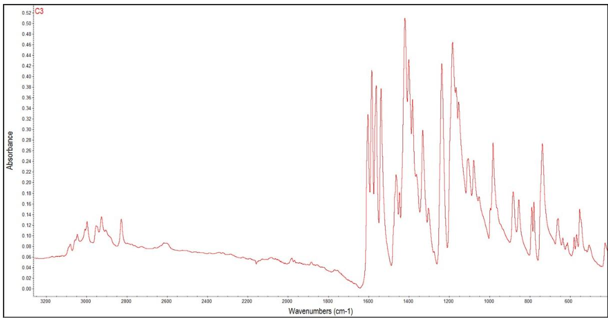
Figure 16S. FT-IR spectrum of C3
