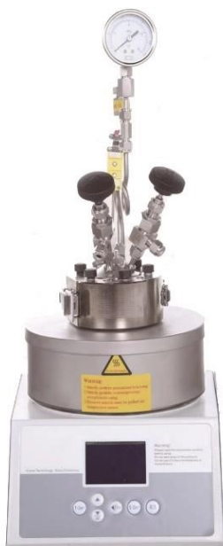
Fig.S1 High-pressure hydrothermal reactor.
