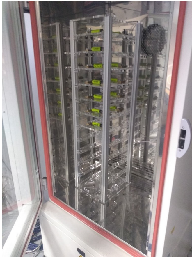
Figure S4: Thermal chamber including racks for cell testing
