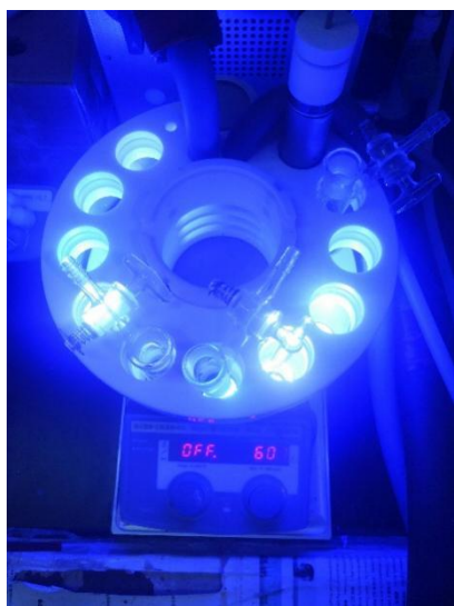
Watecs Parallel Light Reactor equipped with a coolant circulating pump (Blue LED Light source, 445-450 nm, 10 W every position)
