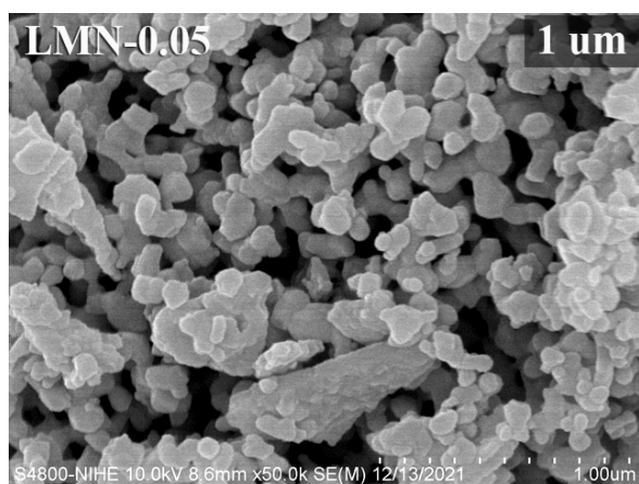
Fig. S4. FE-SEM image (left) and particle size distribution histogram (right) of \text{LaMn}_{0.95}\text{Ni}_{0.05}\text{O}_3 .
