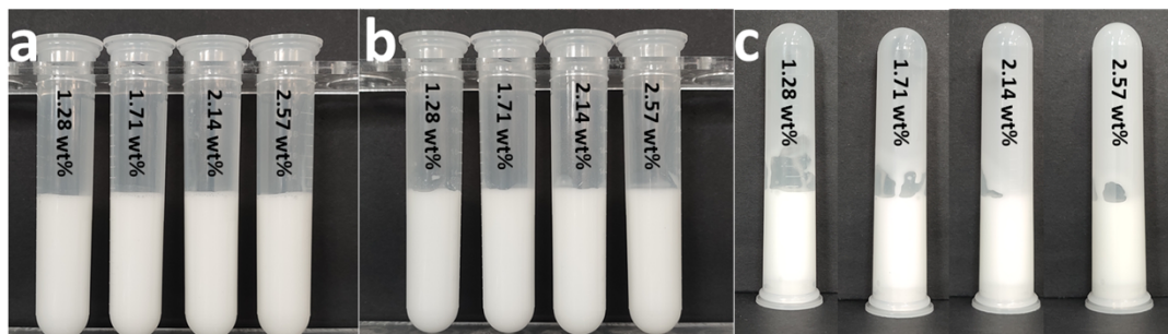
Figure S4. The stability test of the Pickering emulsion with different PEI-g-PNIPAm microgel content where the PMHS/water mass ratio was 3/7. a) the fresh prepared Pickering emulsion with different microgel content. b) the Pickering emulsion after centrifuge processing at the speed of 3000 rpm for 15 min. c) the inverted moment of the Figure b.
