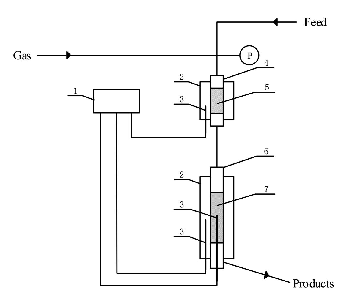
1.PID temperature controller, 2.Electrical heating, 3.Thermocouple, 4.Feed preheater, 5.Packing, 6.Fixed-bed reactor, 7.Catalyst
