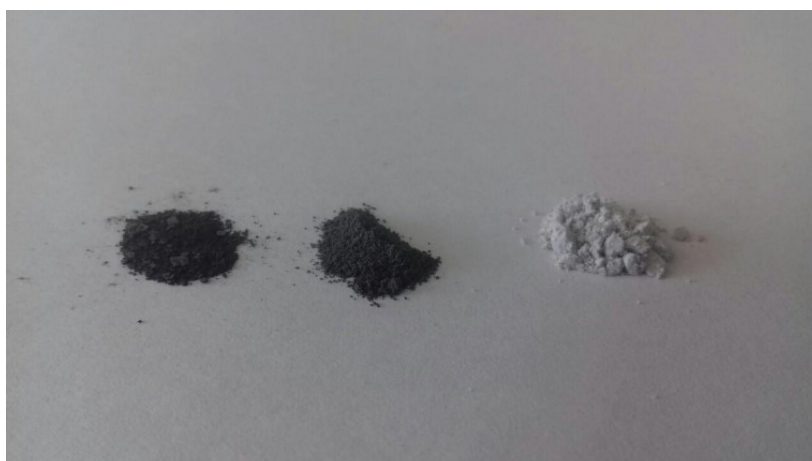
Figure S1. Three types of catalysts in terms of ZnS content. Respectively from right to left RGO-ZnS1%, RGO5%-ZnS, and RGO10%-ZnS.
