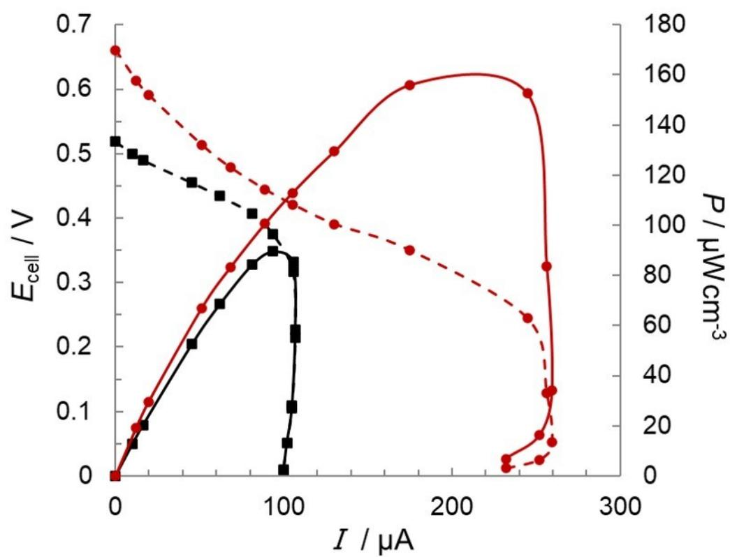
**Figure S5** The polarization curves (dotted lines) and power curves (solid lines) of the EBFCs with a Nafion membrane (red) and without membrane (black).
