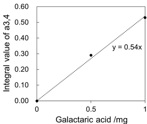
**Figure S8** Calibration curve of galactaric acid generated using NMR. The measurement solution was prepared by dissolving galactaric acid (0.29 mg, 0.53 mg) in 500  $\mu$ L of a deuterated buffer and adding DSS (0.5 mg/5  $\mu$ L). The integrated intensity of the 3.95 ppm peak of galactaric acid (a3,4) was calculated using an integrated intensity of 1 for the 0 ppm peak of DSS.
