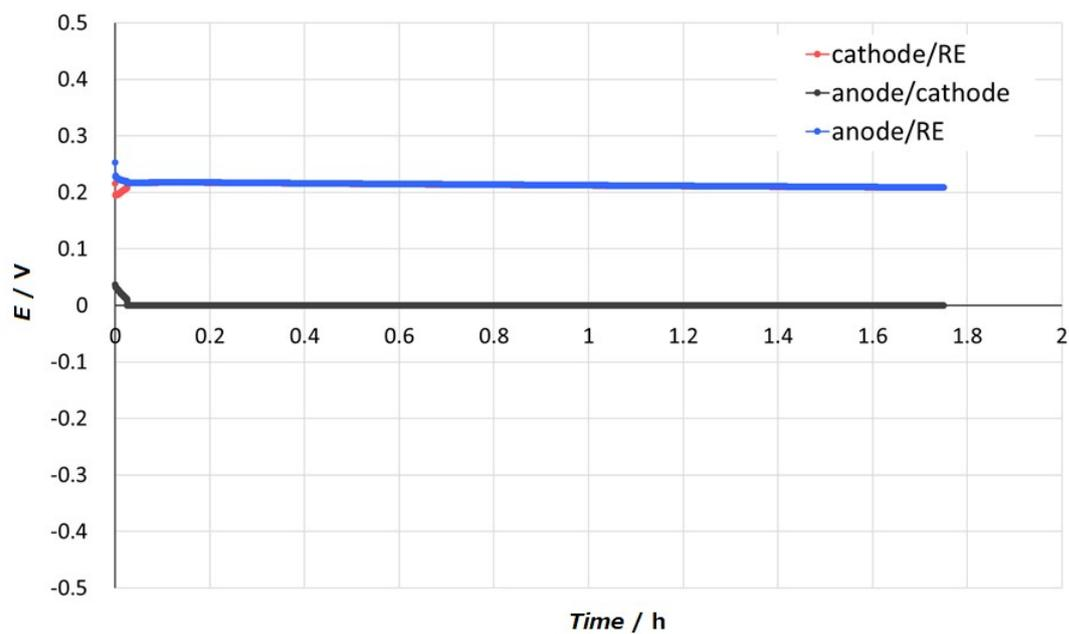
**Figure S7** V-t curve of the cathode (red) without BOD, anode without PQQ-GDH (blue), and cell (black). All conditions are the same as in Fig. 5 except for the absence of enzyme on both electrodes.
