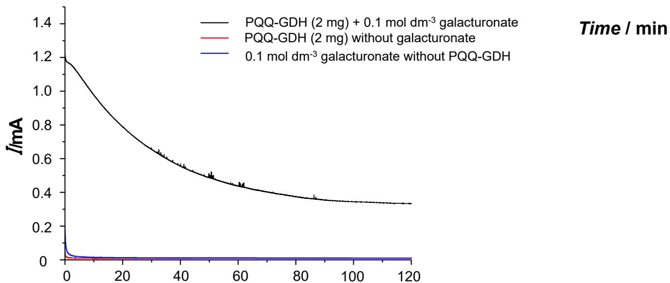
**Figure S1** Amperometric I-t curves for a PMG modified CF electrode. Measurements under conditions with enzyme and substrate (black), substrate and no enzyme (red), and enzyme and no substrate (blue).
