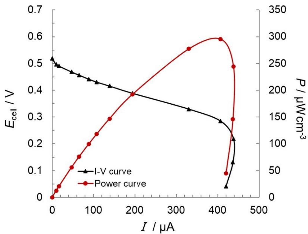
**Figure S4** The polarization curve (black) and power curve (red) of the EBFC using glucose as a substrate.
