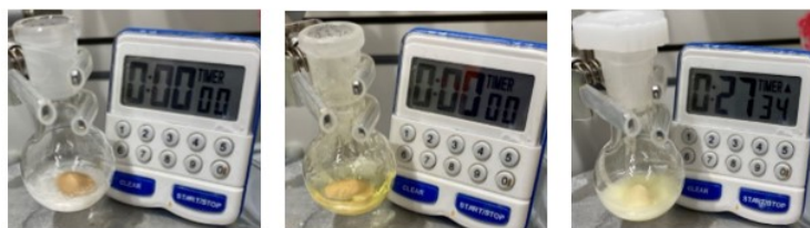
Fig. S5. Chlorosulfonylation of diphenyl disulfide ( 4 ) in MeCN with 10% water. Left: before the addition of DCH, center: after adding DCH, right: 27 minutes reaction time.
