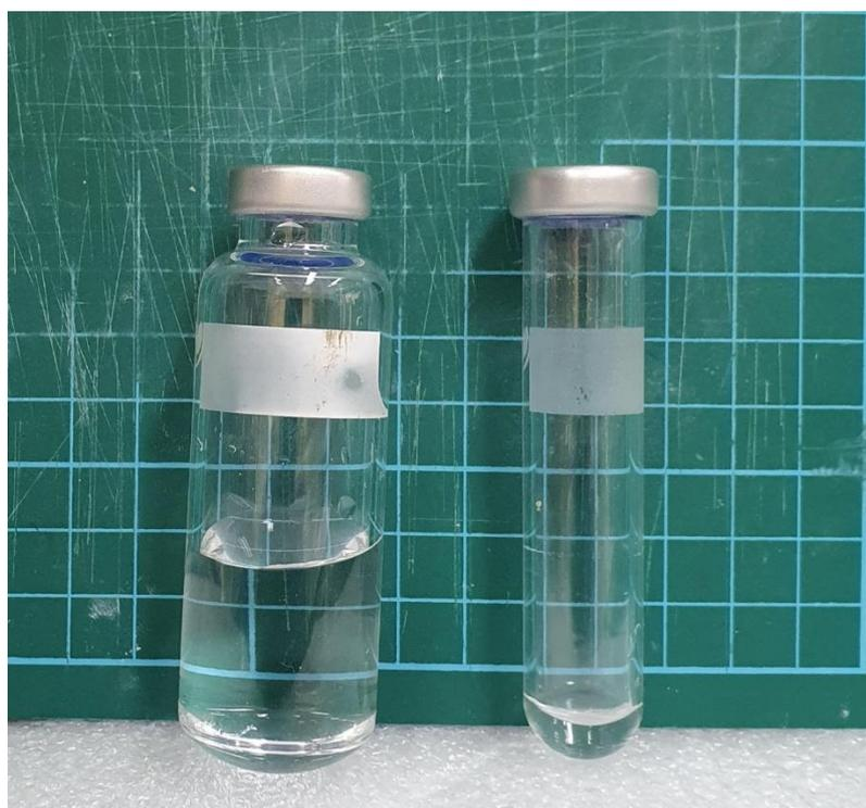
Reactor vessels used in this study. 30 mL (left) and 10 mL (right) microwave reactor vessel with crimp-seal cap. Solvent volumes for the 20 mg and 500 mg scale reactions are illustrated by water.
