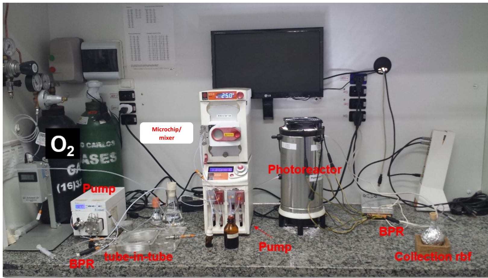
Figure S7 – Flow setup 2 for the synthesis of pinocarvones (2a-b)
