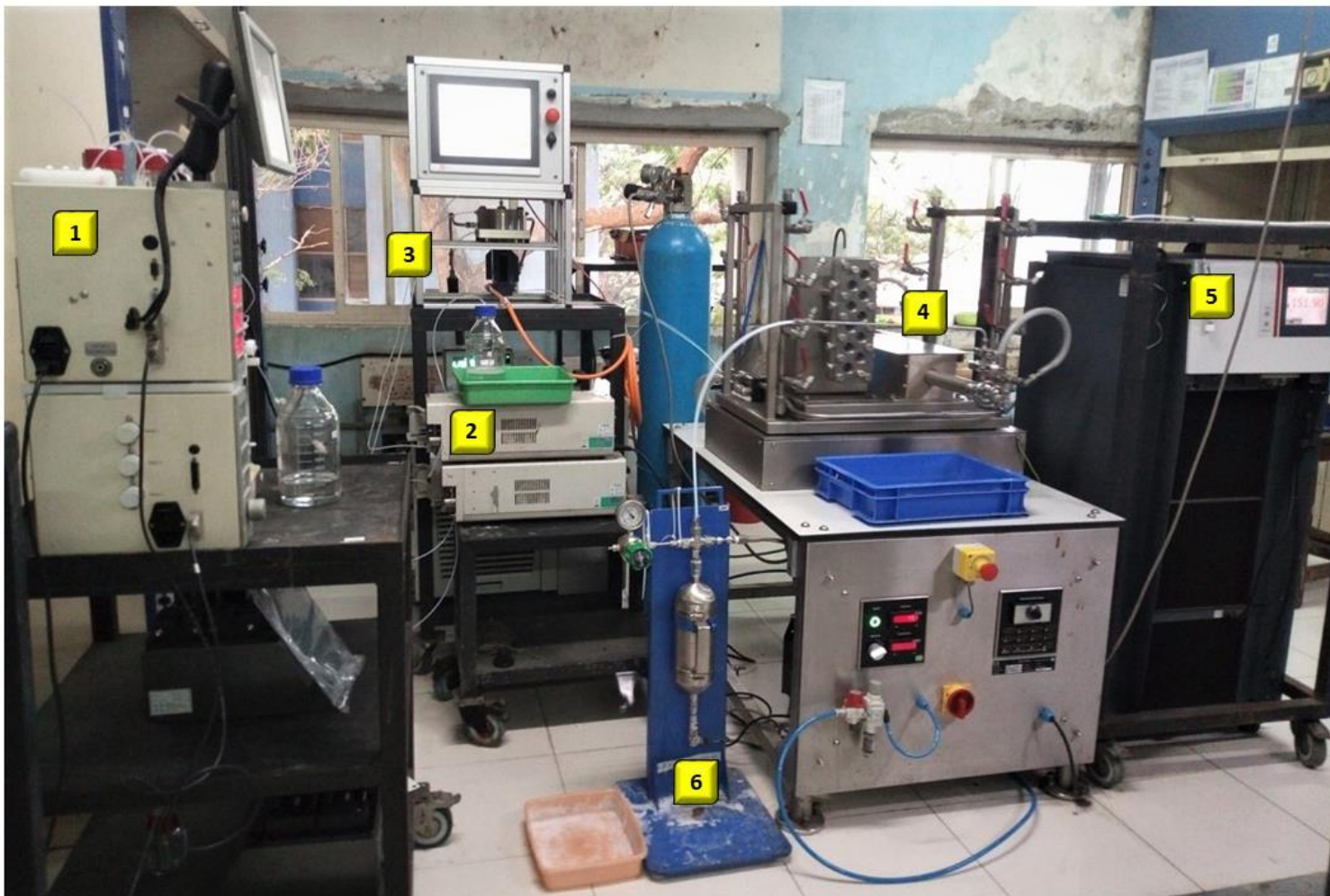
Figure S5: The continuous flow setup used for process intensified continuous flow synthesis of DFNS; (1) and (2) Pumps for organic and aqueous solutions; (3) Spinning Disk Reactor for in situ emulsification; (4) Agitated Cell Reactor for scalable performance; (5) Chiller for maintaining reaction temperature; (6) Back Pressure Regulator-cum-collector
