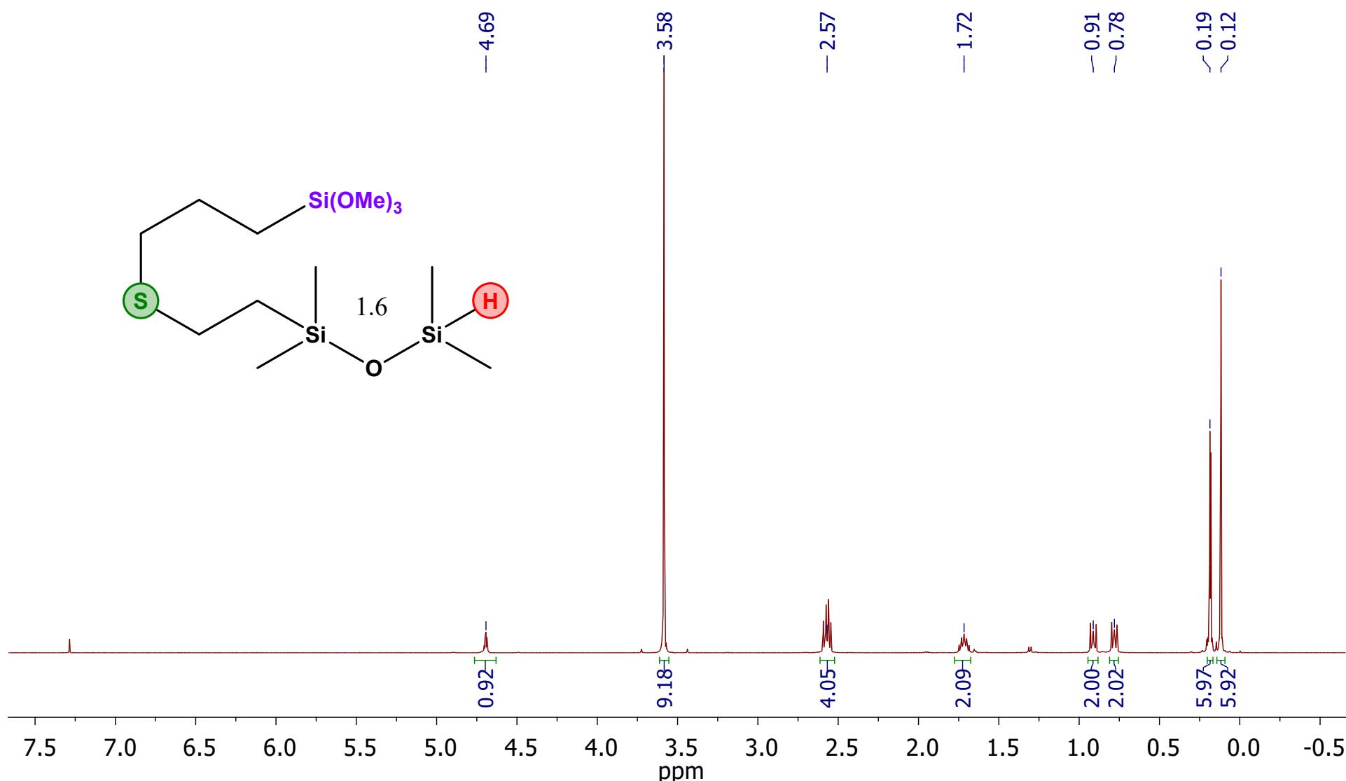
**Figure 65s.**  $^1\text{H}$  NMR spectrum of compound **1.6** (500 MHz, solvent –  $\text{CDCl}_3$ ).
