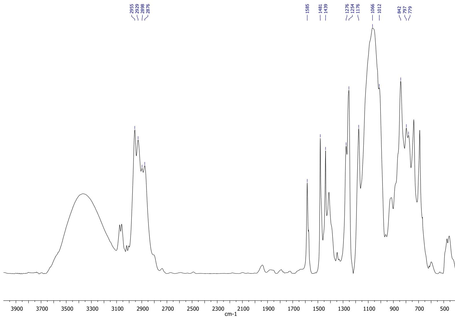
**Figure 164s.** IR-spectrum of compound 3.1.1. (the presence of an OH group is associated with the presence of moisture in potassium bromine, which leads to the partial hydrolysis during the analysis)
