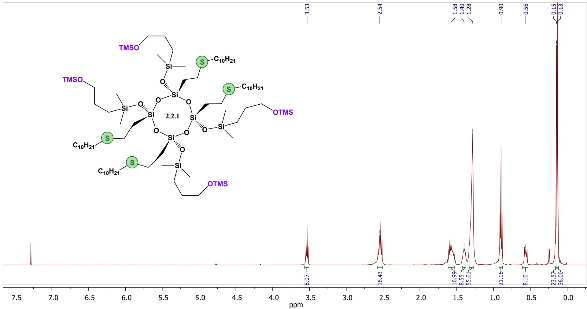
**Figure 135s.**  $^1\text{H}$  NMR spectrum of compound 2.2.1 (500 MHz, solvent –  $\text{CDCl}_3$ ).
