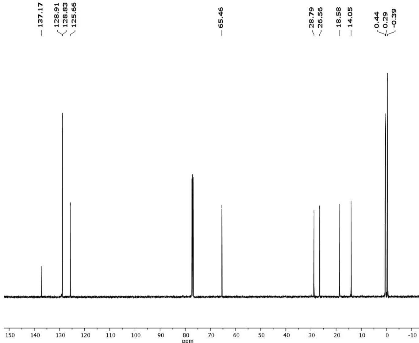
**Figure 102s.**  $^{13}\text{C}$  NMR spectrum of compound 1.1.1 (100 MHz, solvent –  $\text{CDCl}_3$ ).
