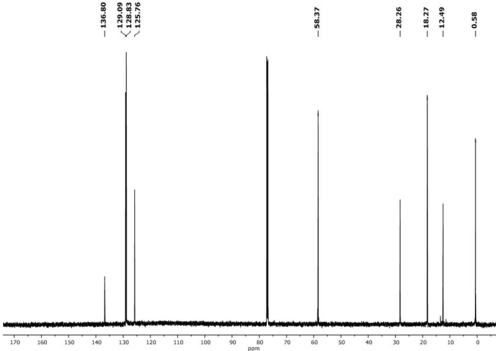
**Figure 76s.**  $^{13}\text{C}$  NMR spectrum of compound 3.1 (100 MHz, solvent –  $\text{CDCl}_3$ ).
