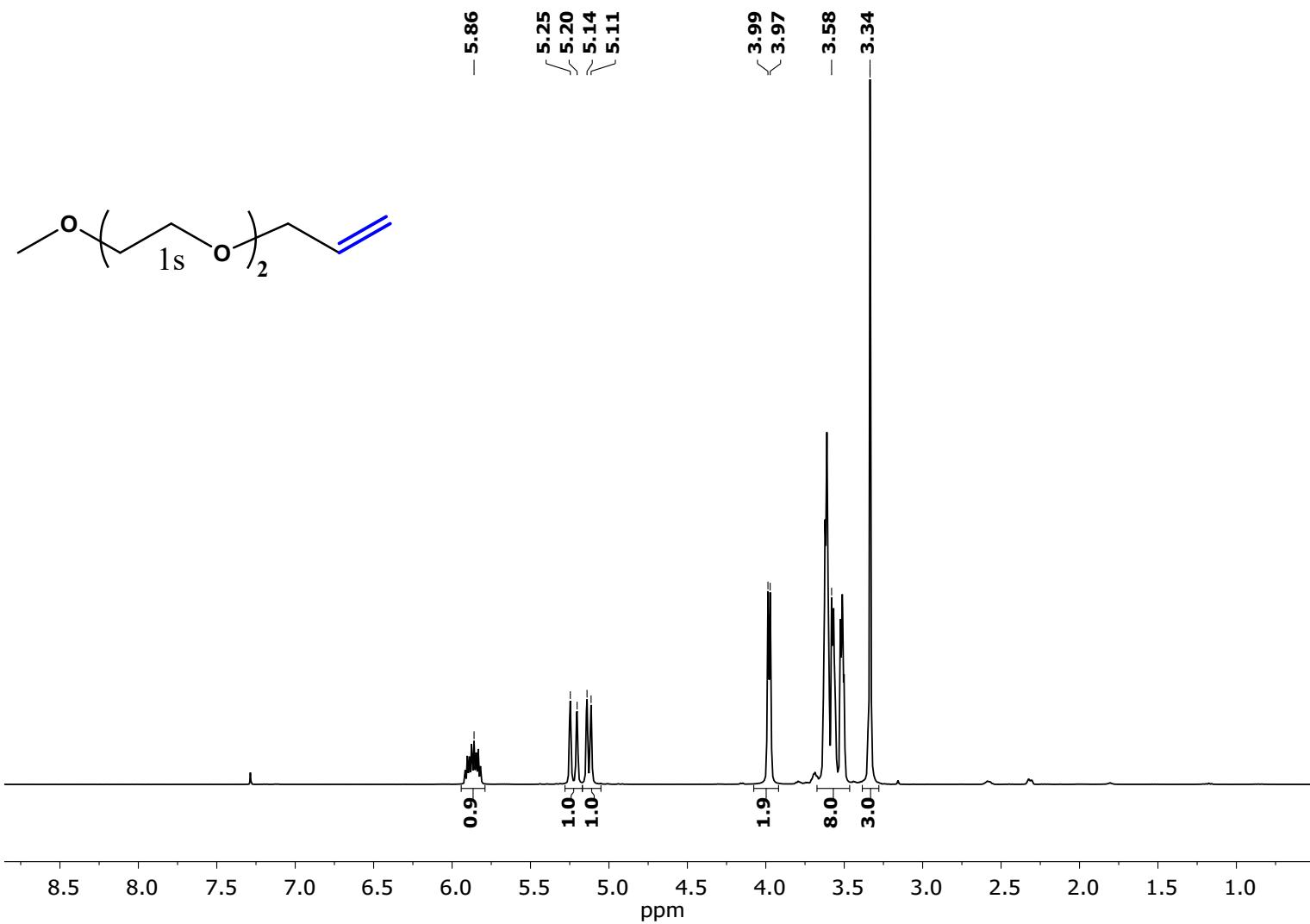
**Figure 21s.**  $^1\text{H}$  NMR spectrum of compound **1'** (400 MHz, solvent –  $\text{CDCl}_3$ ).
