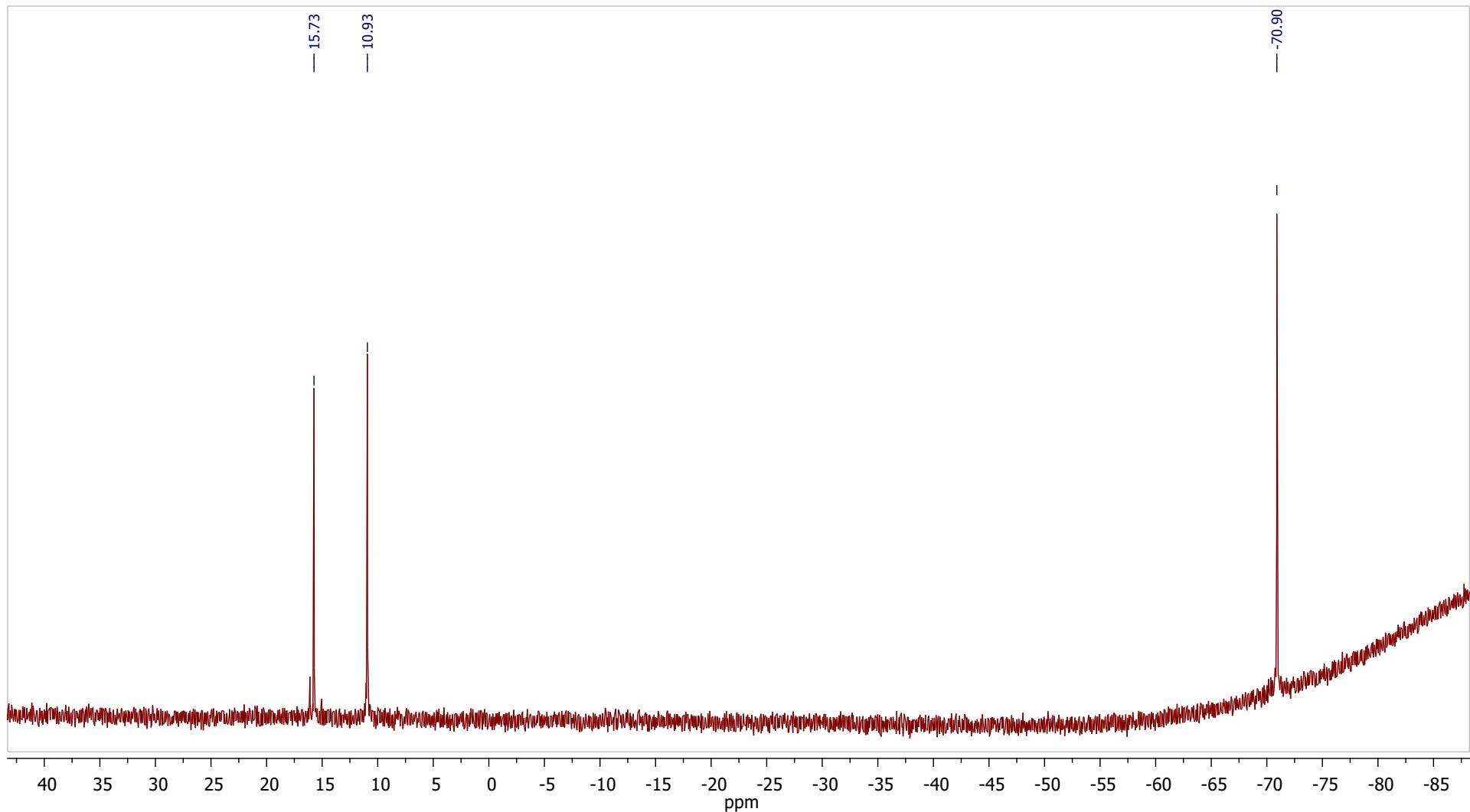
**Figure 133s.**  $^{29}\text{Si}$  NMR spectrum of compound **2.1.1** (500 MHz, solvent –  $\text{CDCl}_3$ ).
