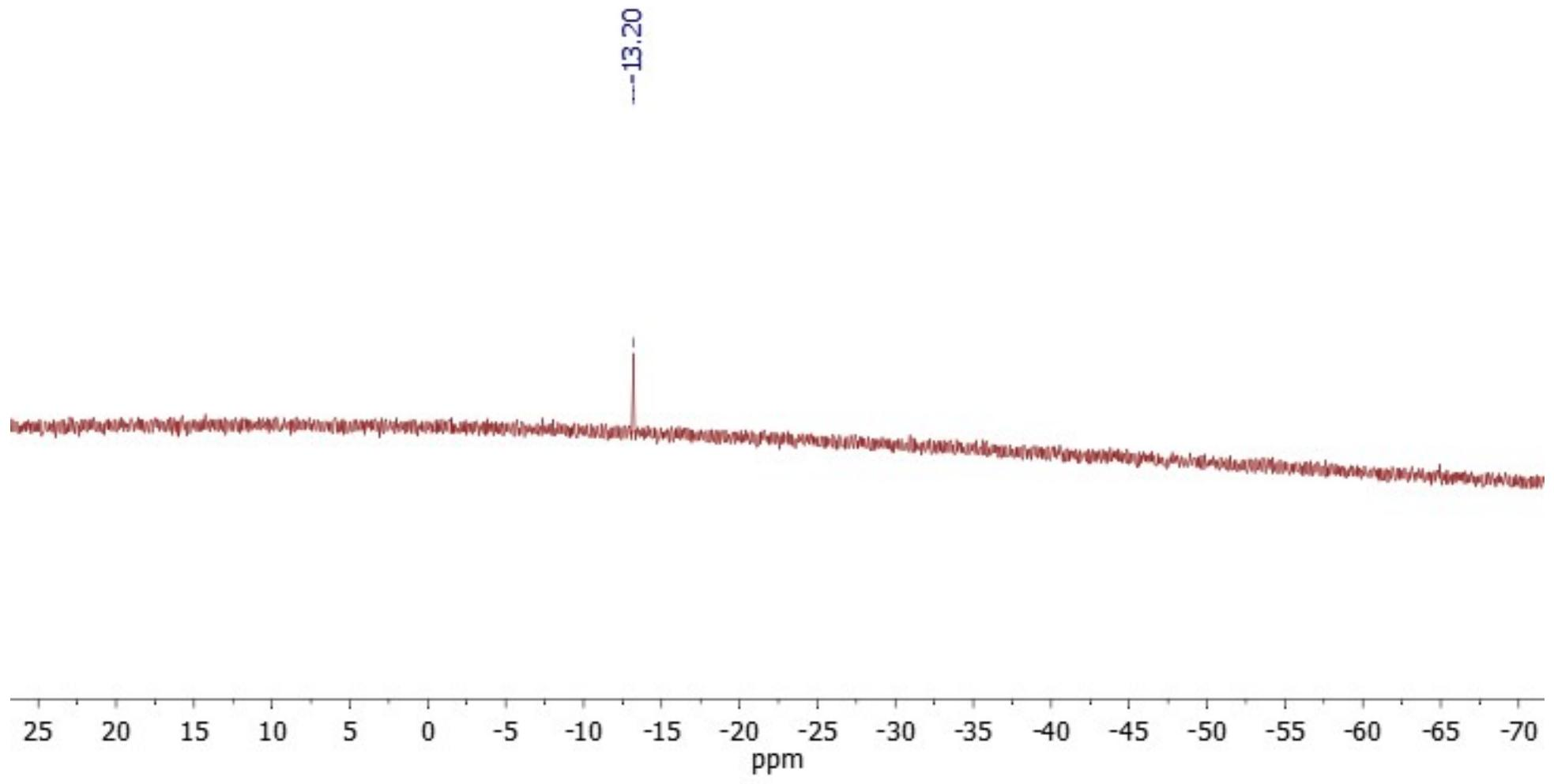
**Figure 9s.**  $^{29}\text{Si}$  NMR spectrum of compound  $\gamma\text{-Ph}$  (500 MHz, solvent –  $\text{CDCl}_3$ ).
