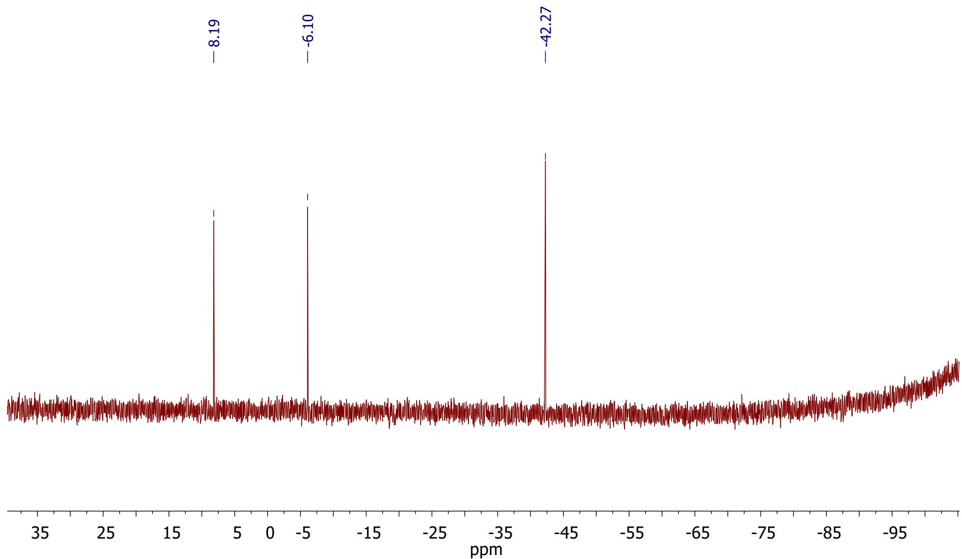
**Figure 67s.**  $^{29}\text{Si}$  NMR spectrum of compound **1.6** (400 MHz, solvent –  $\text{CDCl}_3$ ).
