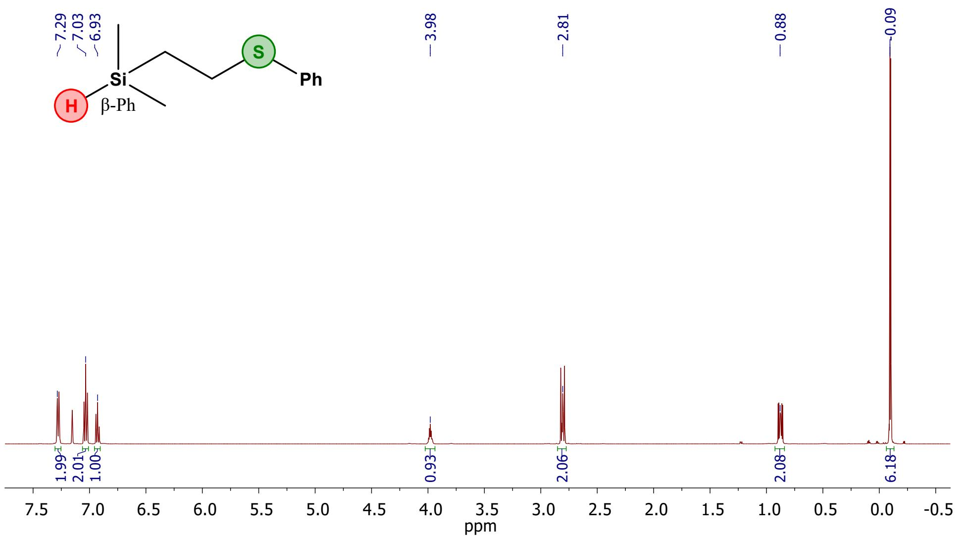
**Figure 2s.**  $^1\text{H}$  NMR spectrum of compound  $\beta\text{-Ph}$  (500 MHz, solvent – C<sub>6</sub>D<sub>6</sub>).
