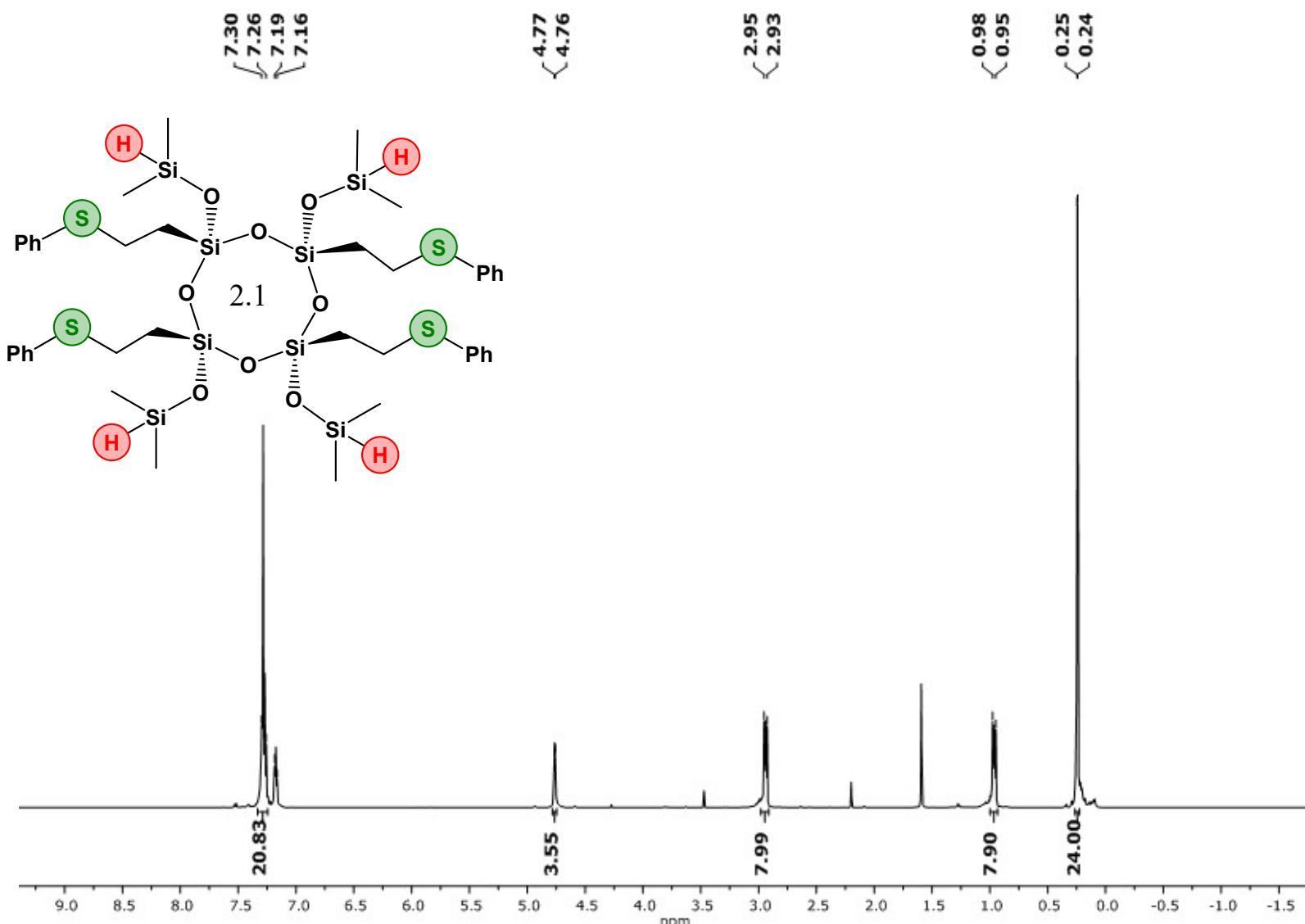
**Figure 80.**  $^1\text{H}$  NMR spectrum of compound **2.1** (400 MHz, solvent –  $\text{CDCl}_3$ ).
