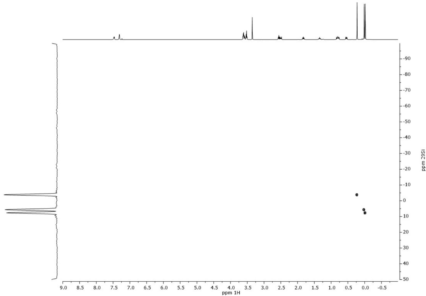
**Figure 117s.** HMBC  $^1\text{H}$ - $^{29}\text{Si}$  NMR spectrum of compound **1.2.2** (solvent – CDCl<sub>3</sub>).
