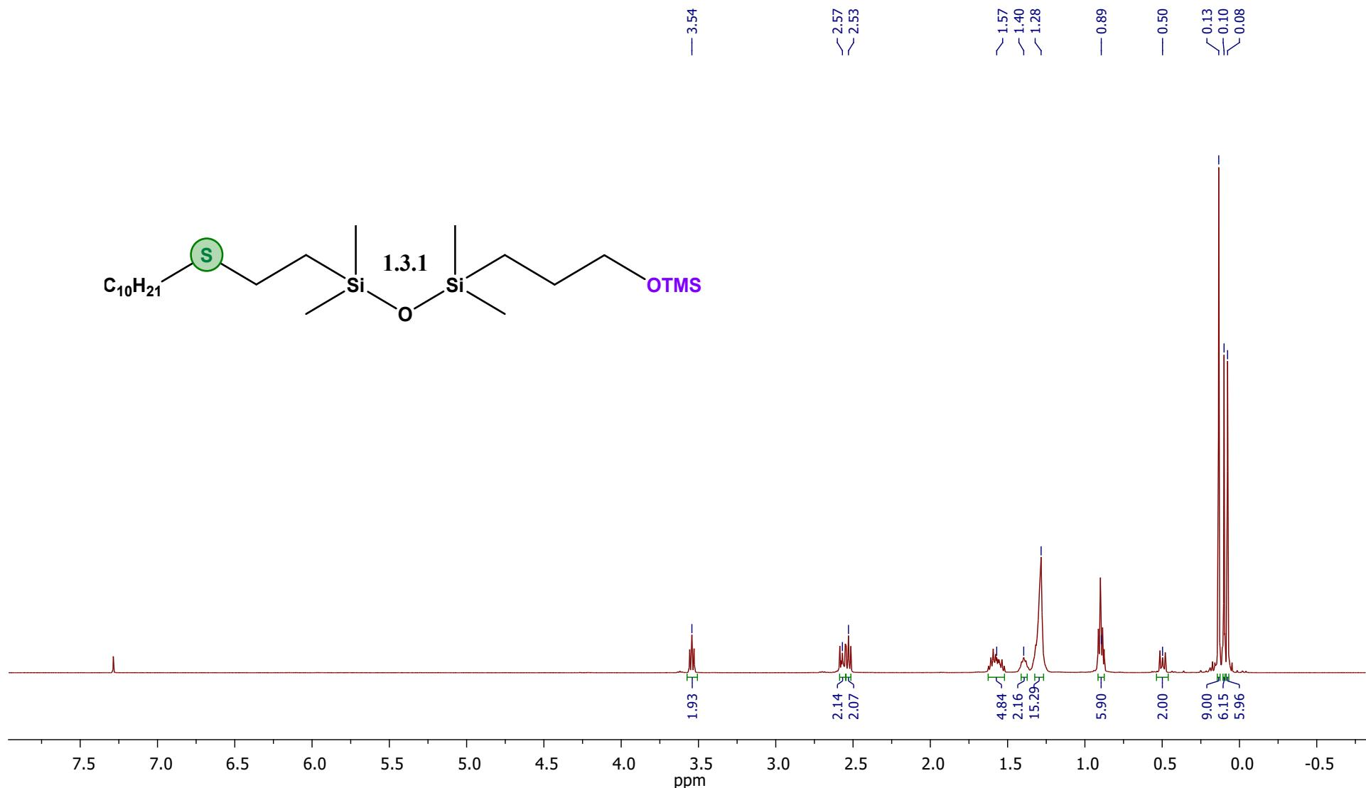
**Figure 120s.**  $^1\text{H}$  NMR spectrum of compound **1.3.1** (500 MHz, solvent –  $\text{CDCl}_3$ ).
