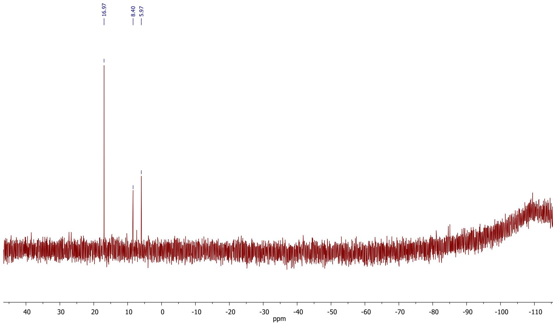
**Figure 122s.**  $^{29}\text{Si}$  NMR spectrum of compound **1.3.1** (500 MHz, solvent –  $\text{CDCl}_3$ ).
