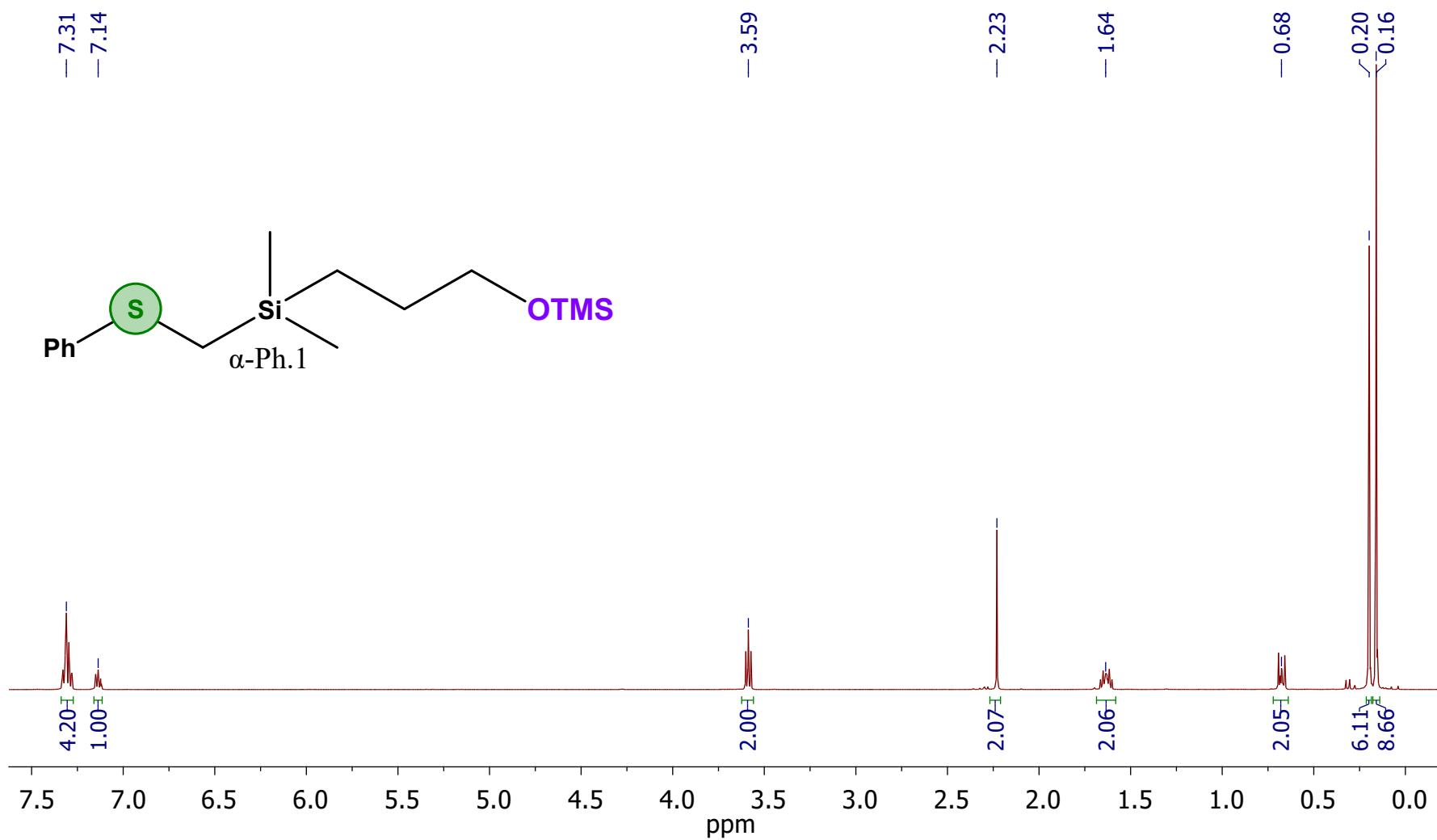
**Figure 96s.**  $^1\text{H}$  NMR spectrum of compound **α-Ph.1** (600 MHz, solvent –  $\text{CDCl}_3$ ).
