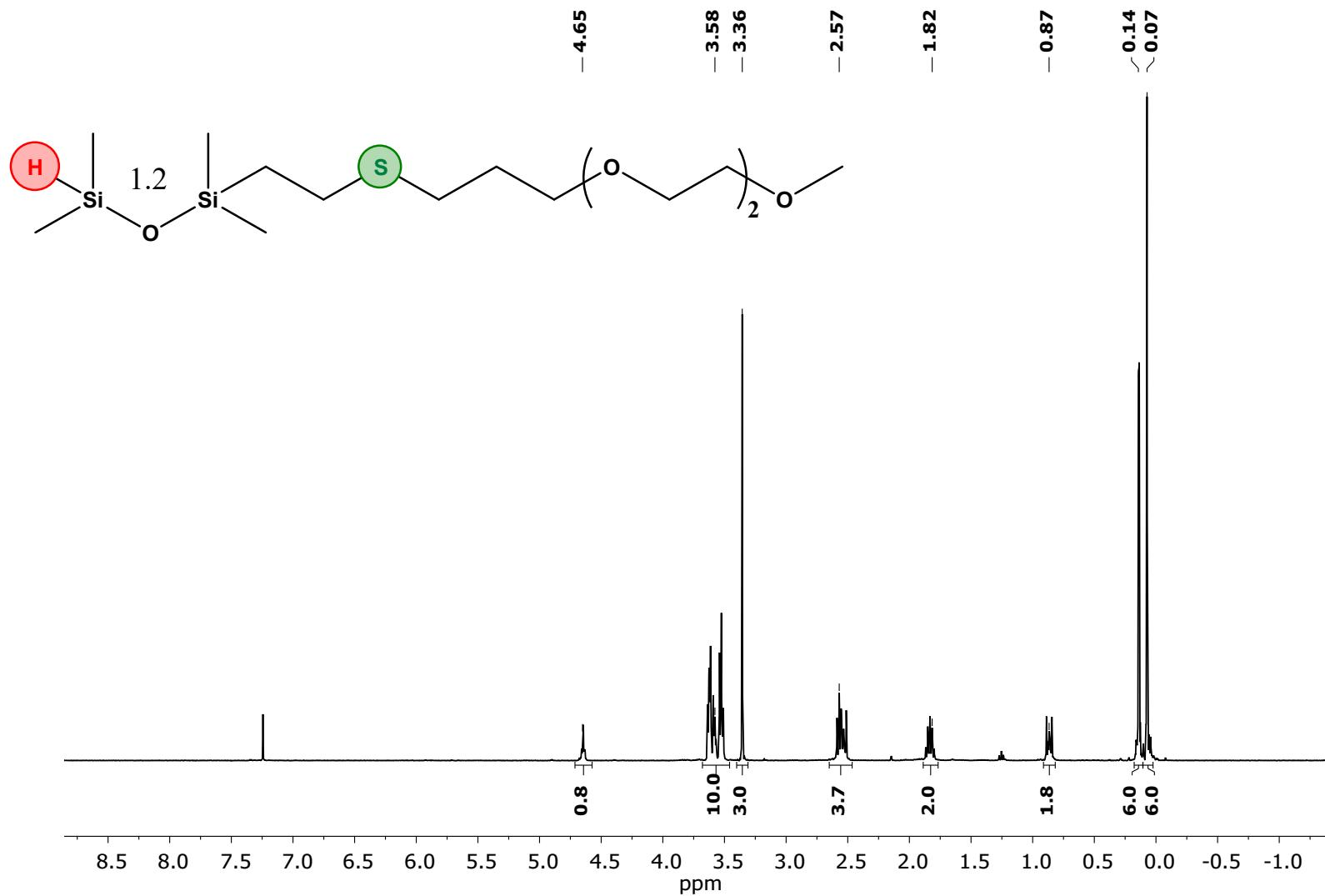
**Figure 33s.**  $^1\text{H}$  NMR spectrum of compound **1.2** (400 MHz, solvent –  $\text{CDCl}_3$ ).
