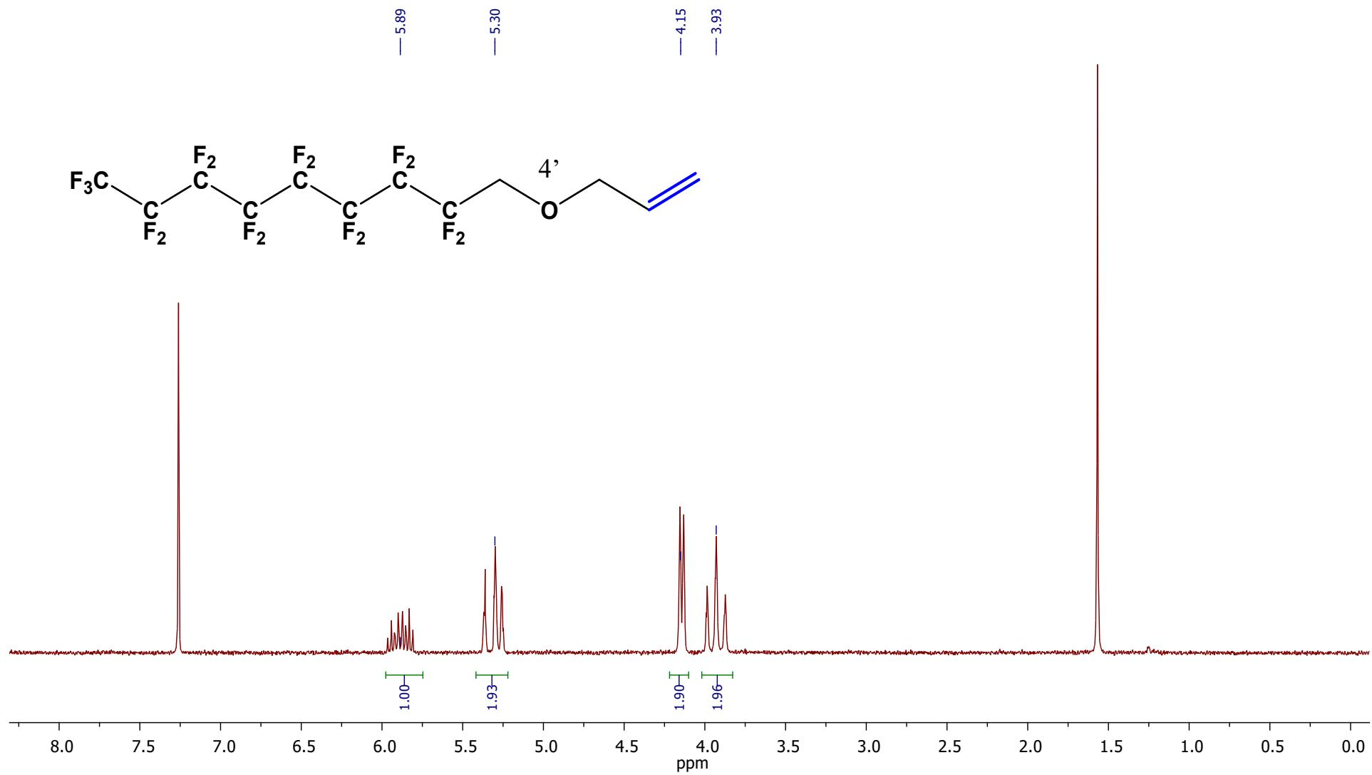
**Figure 43s.**  $^1\text{H}$  NMR spectrum of compound  $4'$  (400 MHz, solvent –  $\text{CDCl}_3$ ).
