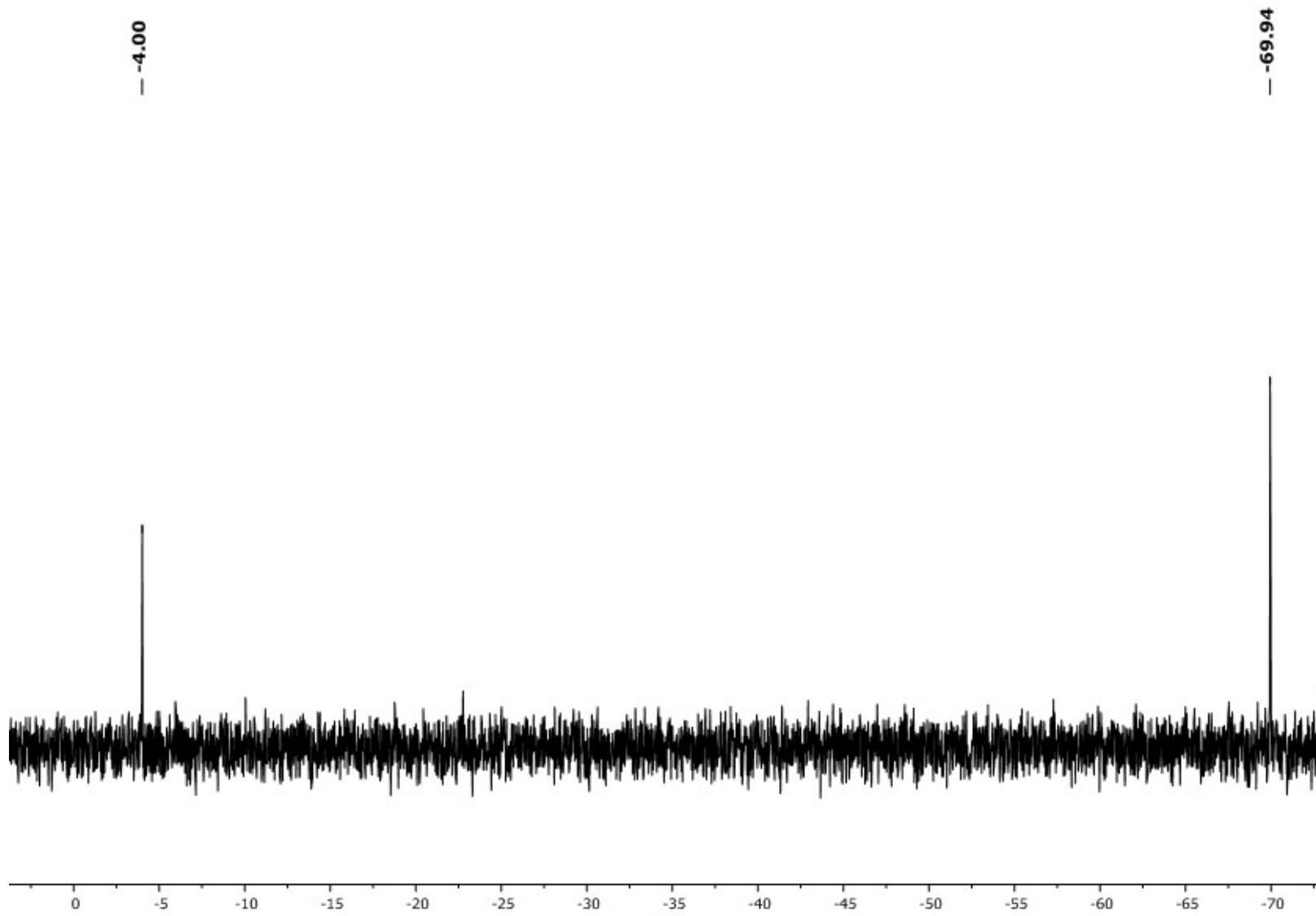
**Figure 82s.**  $^{29}\text{Si}$  NMR spectrum of compound **2.1** (80 MHz, solvent –  $\text{CDCl}_3$ ).
