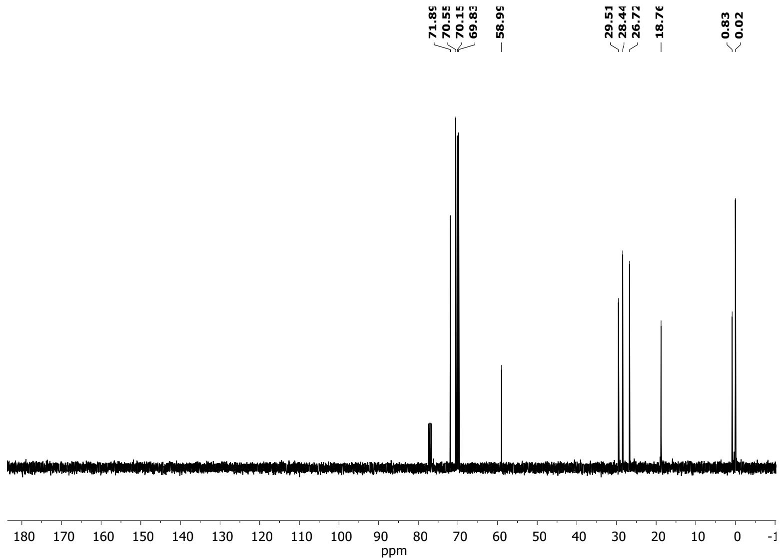
**Figure 34s.**  $^{13}\text{C}$  NMR spectrum of compound 1.2 (100 MHz, solvent –  $\text{CDCl}_3$ ).
