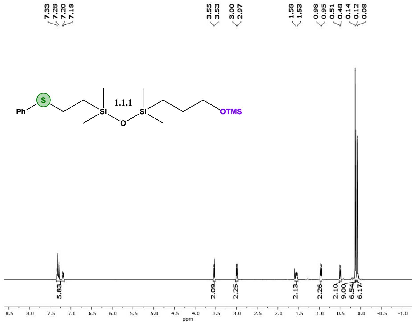
**Figure 101s.**  $^1\text{H}$  NMR spectrum of compound **1.1.1** (400 MHz, solvent –  $\text{CDCl}_3$ ).
