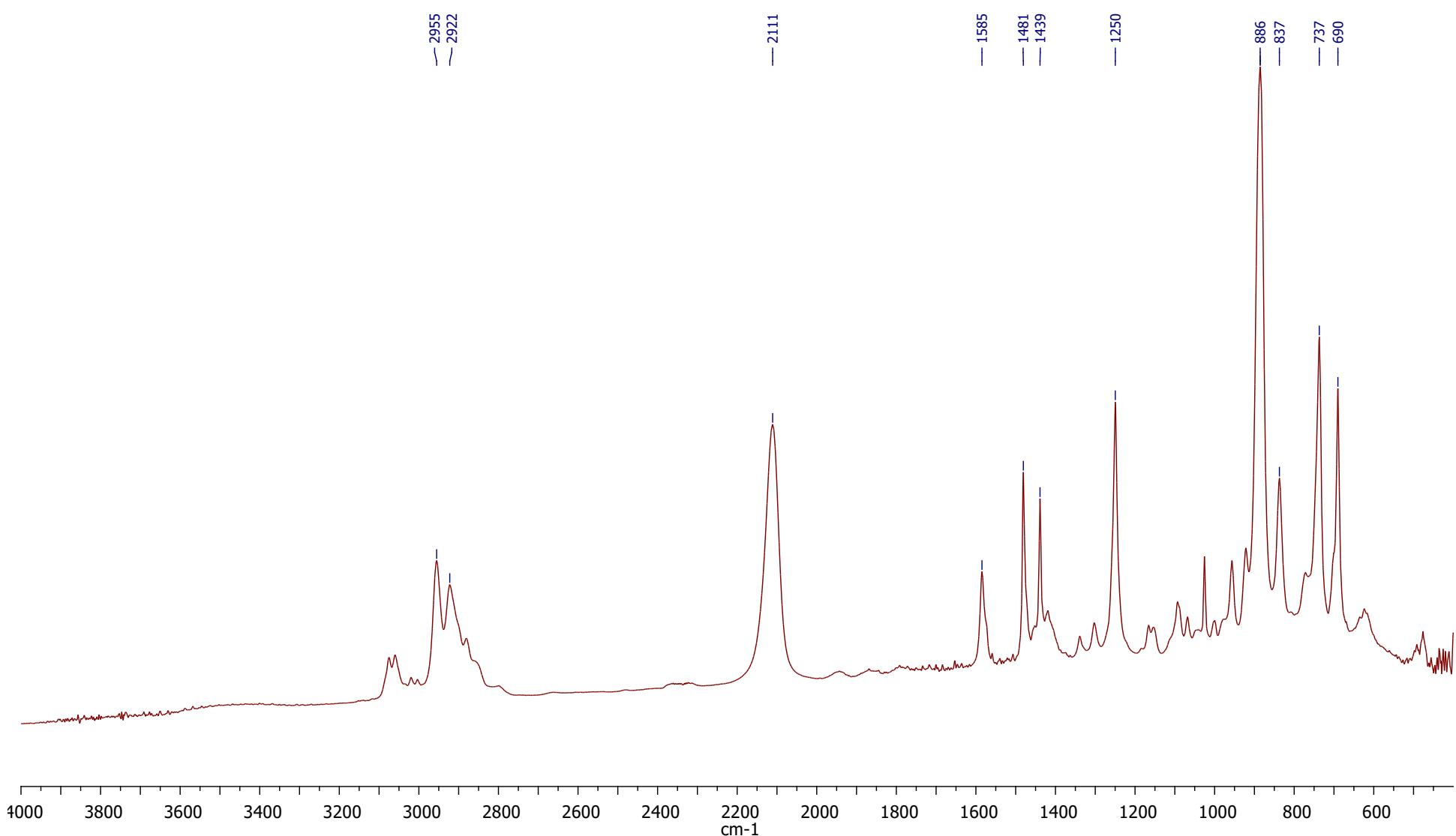
**Figure 10s.** IR-spectrum of compound  $\gamma$ -Ph.
