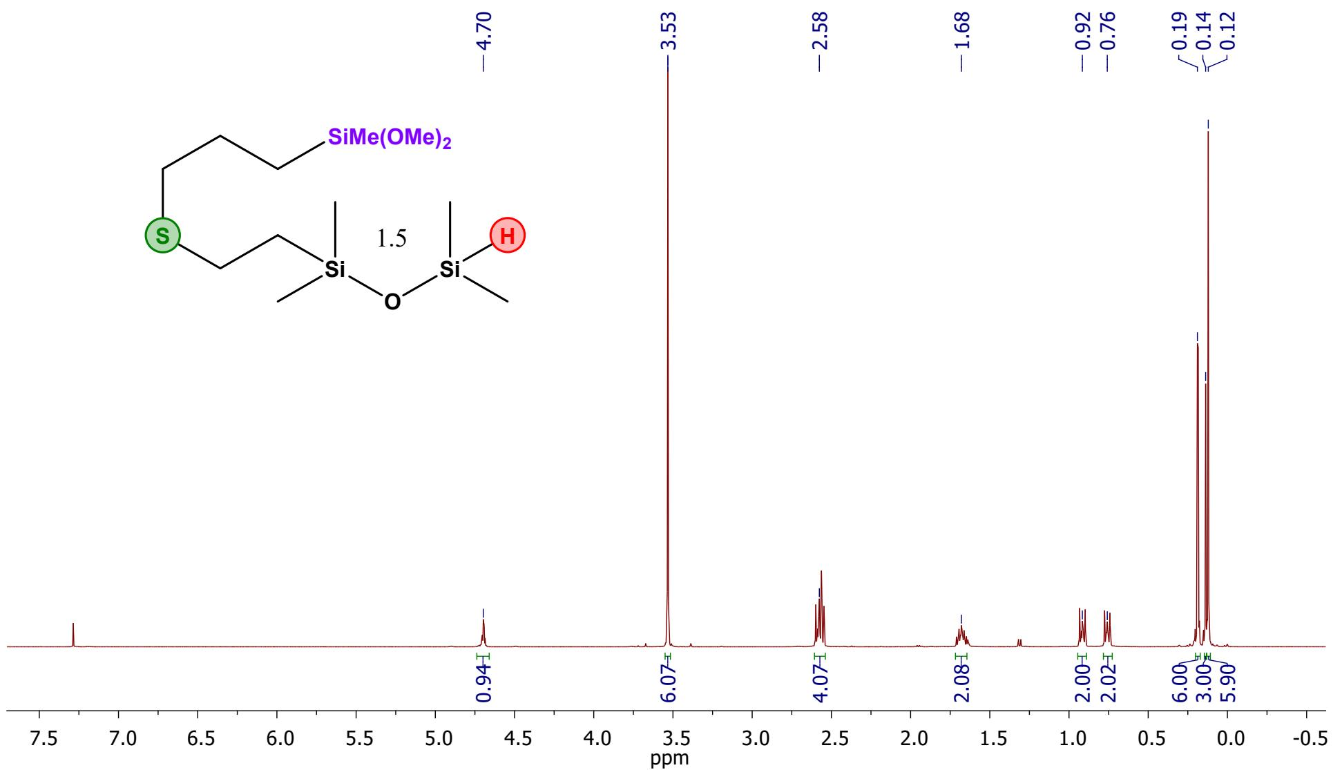
**Figure 60s.**  $^1\text{H}$  NMR spectrum of compound **1.5** (500 MHz, solvent –  $\text{CDCl}_3$ ).
