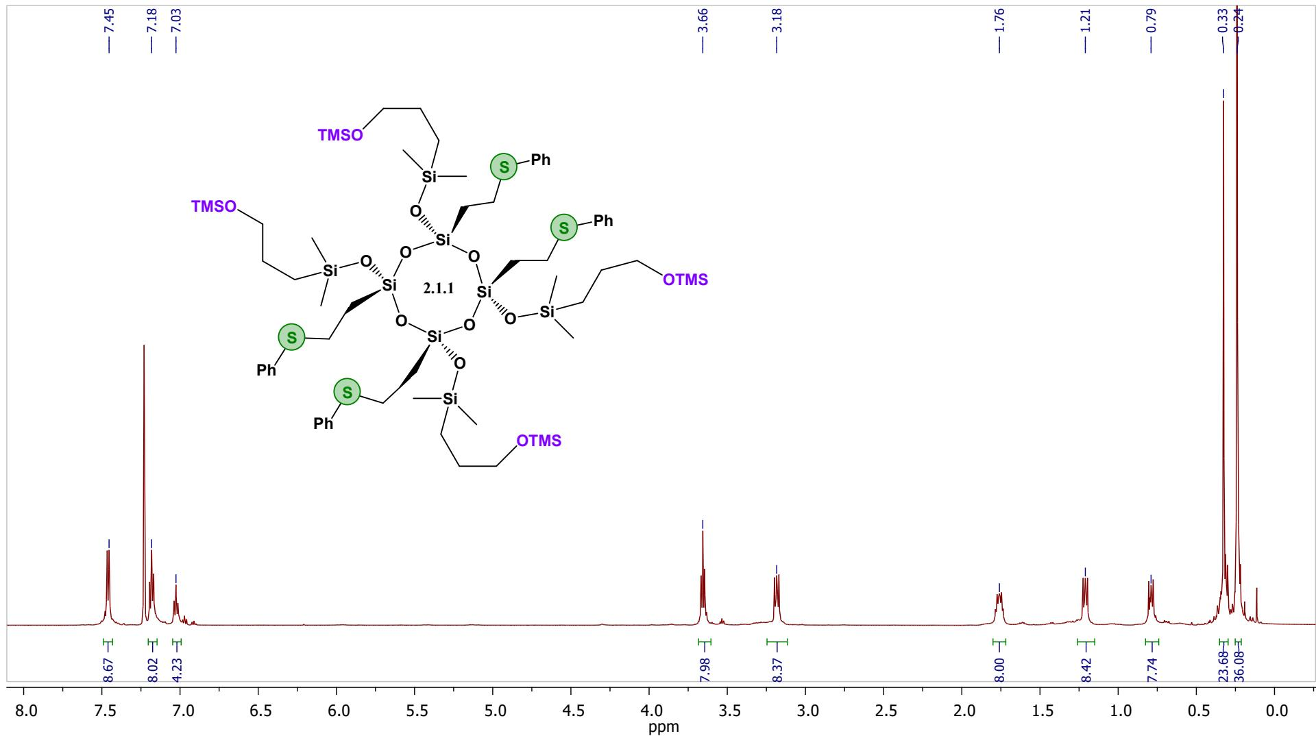
**Figure 131s.**  $^1\text{H}$  NMR spectrum of compound **2.1.1** (500 MHz, solvent –  $\text{CDCl}_3$ ).
