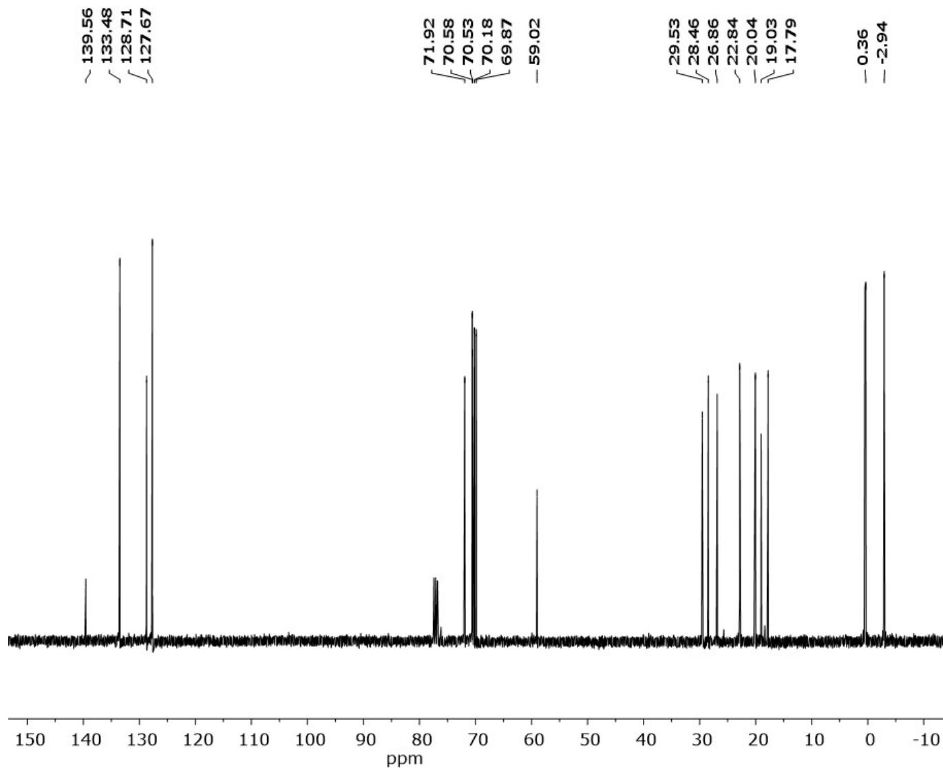
**Figure 116s.**  $^{13}\text{C}$  NMR spectrum of compound 1.2.2 (100 MHz, solvent –  $\text{CDCl}_3$ ).
