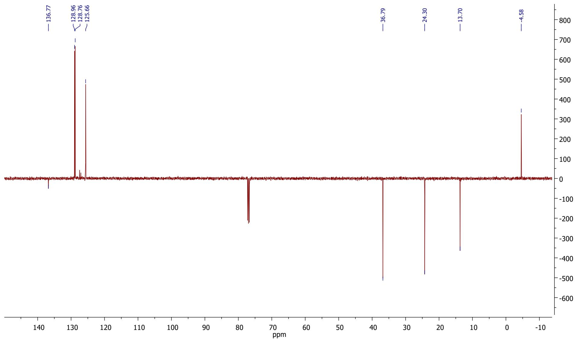
**Figure 8s.**  $^{13}\text{C}$  NMR spectrum of compound  $\gamma\text{-Ph}$  (500 MHz, solvent –  $\text{CDCl}_3$ , jmod).
