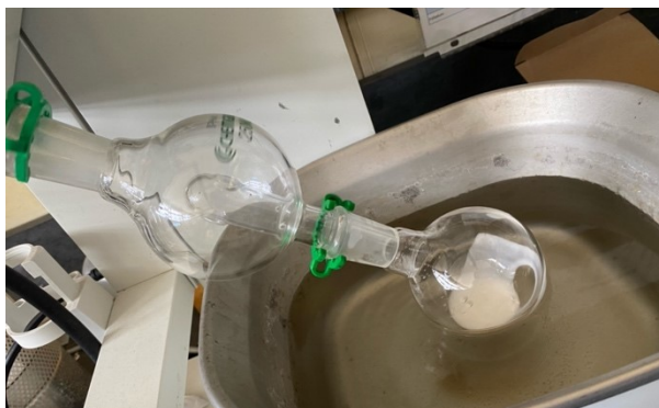
Figure S2. Reaction mixture in the round-bottom flask attached to the bump trap of the rotavap. The flask was submerged in a water bath set to 45°C. Initially the solution is milky white (shown in the picture) but is a clear brown solution after the 5-minute reaction time.
