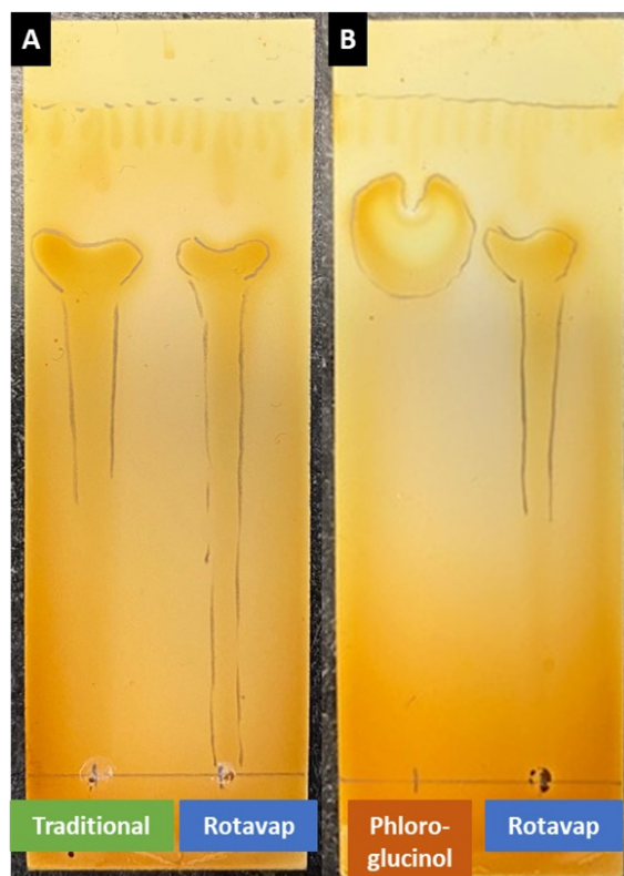
Figure S4. Picture of TLC plate results. (A) Traditionally prepared trioxime product (left) compared to the trioxime product formed in the rotavap (right). (B) Starting material, phloroglucinol (left), compared to the trioxime product formed in the rotavap (right).
