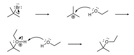
Consider the mechanism for the  $S_N1$  reaction between *t*-butyl iodide and ethanol to form ethyl *t*-butyl ether.
