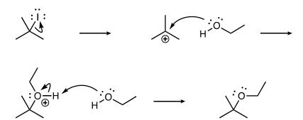
Consider the mechanism for the  $S_N1$  reaction between *t*-butyl chloride and ethanol to form ethyl *t*-butyl ether.
