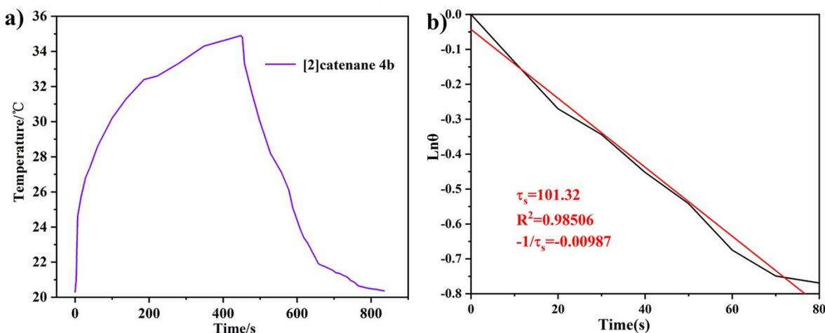
**Fig. S64.** (a) Heating and cooling curve of [2]catenane **4b** (with treble  $\pi$ - $\pi$  stacking interactions); (b) Fitting linear of  $\ln\theta$ -t.
