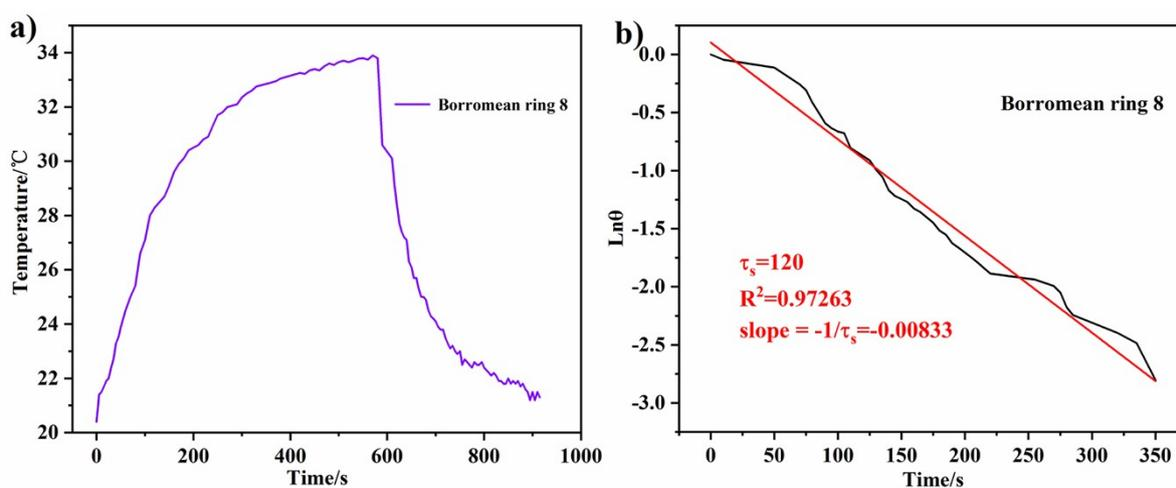
**Fig. S67.** (a) Heating and cooling curve of Borromean ring 8 (with six sets of  $\pi$ - $\pi$  stacking); (b) Fitting linear of  $\ln\theta$ -t.
