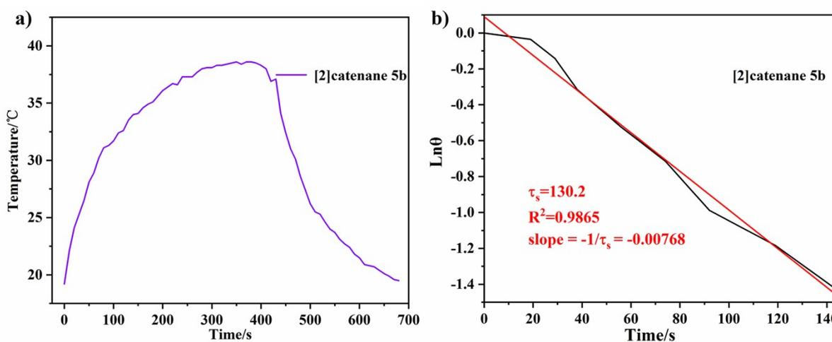
**Fig. S65.** (a) Heating and cooling curve of [2]catenane **5b** (with treble  $\pi$ - $\pi$  stacking interactions); (b) Fitting linear of  $\ln\theta$ -t.
