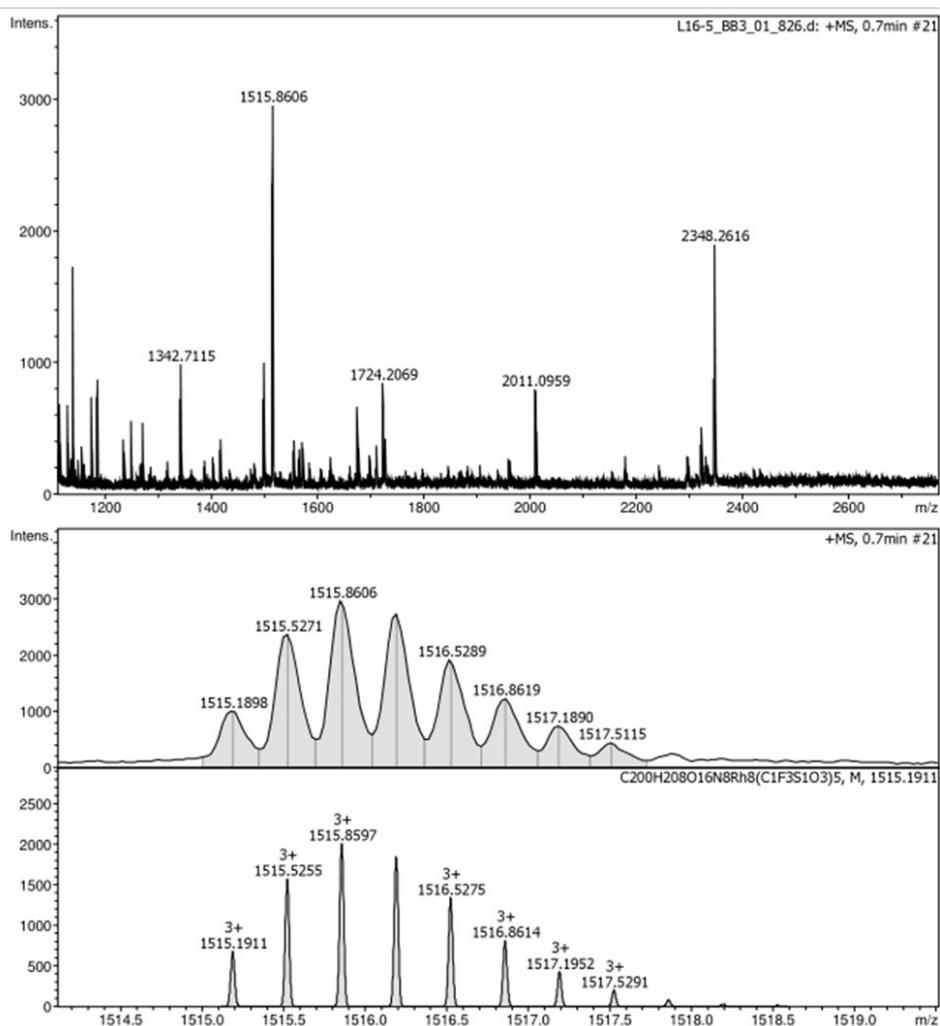
**Fig. S61.** Full ESI-MS spectra (a) of complex **3b**, experimental ESI-MS spectra of  $[\mathbf{3b-3OTf}]^{3+}$  in  $\text{CH}_3\text{OD}$  solvent.
