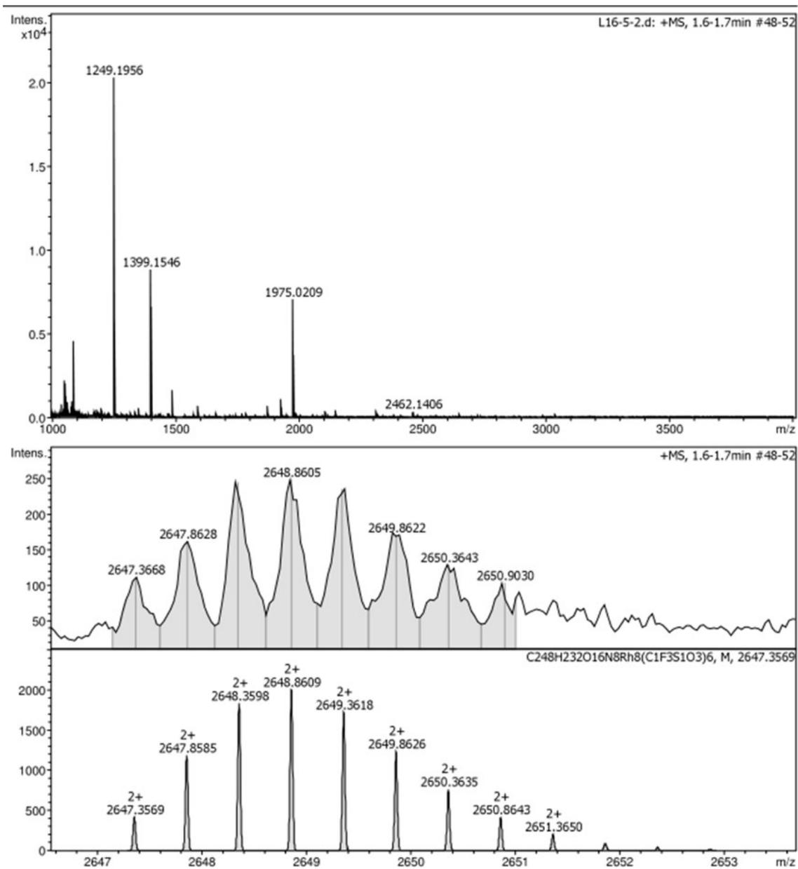
**Fig. S62.** Full ESI-MS spectra (a) of complex **5b**, experimental ESI-MS spectra of [5b-2OTf]<sup>3+</sup> in CH<sub>3</sub>OD solvent.
