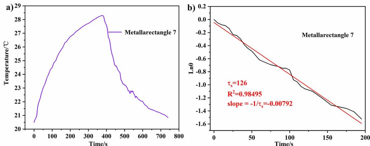
**Fig. S66.** (a) Heating and cooling curve of Metallarectangle 7 (with a single  $\pi$ - $\pi$  stacking); (b) Fitting linear of  $\ln\theta$ -t.
