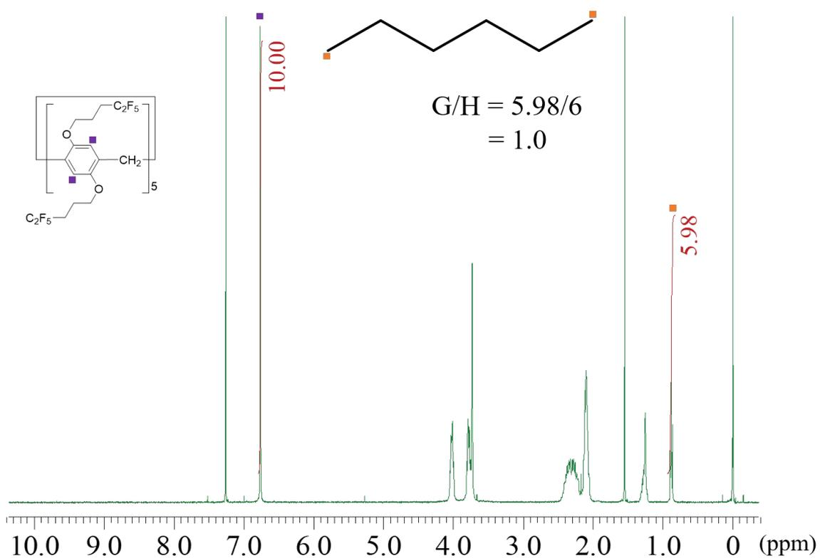
**Fig. S21**  $^1\text{H}$  NMR spectrum of *c*-(F5D)H ( $\text{CDCl}_3$ ,  $25\text{ }^\circ\text{C}$ ). The uptake ratio of *n*-hexane to F5 (G/H) calculated from the integration ratio was 1.0.
