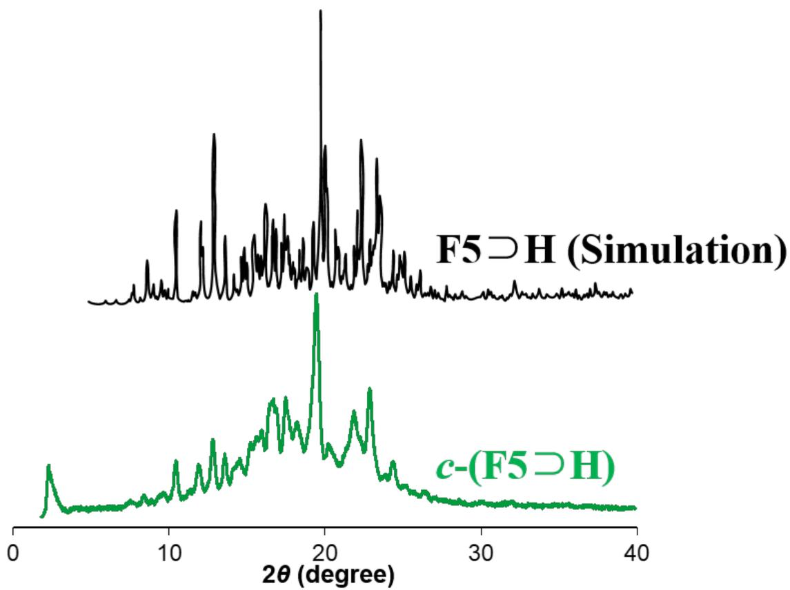
**Fig. S28** PXRD patterns of simulation from single crystal of **F5D H** (upper side) and **c-(F5D H)** (lower side).
