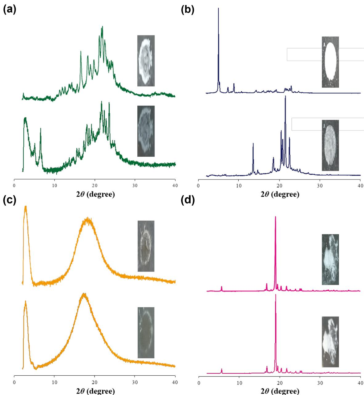
**Fig. S22** Photographs and PXRD patterns of (a) **F3**, (b) **C5**, (c) **F13** and (d) **Monomer Unit** before (lower side) and after (upper side) exposure to *n*-hexane vapor.
