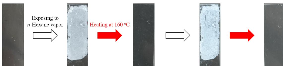
**Fig. S49** Photographs of **F5** by exposing *a*-**F5** to *n*-hexane vapor and heating *c*-(**F5**⇌**P**) at 160 °C repeatedly.
