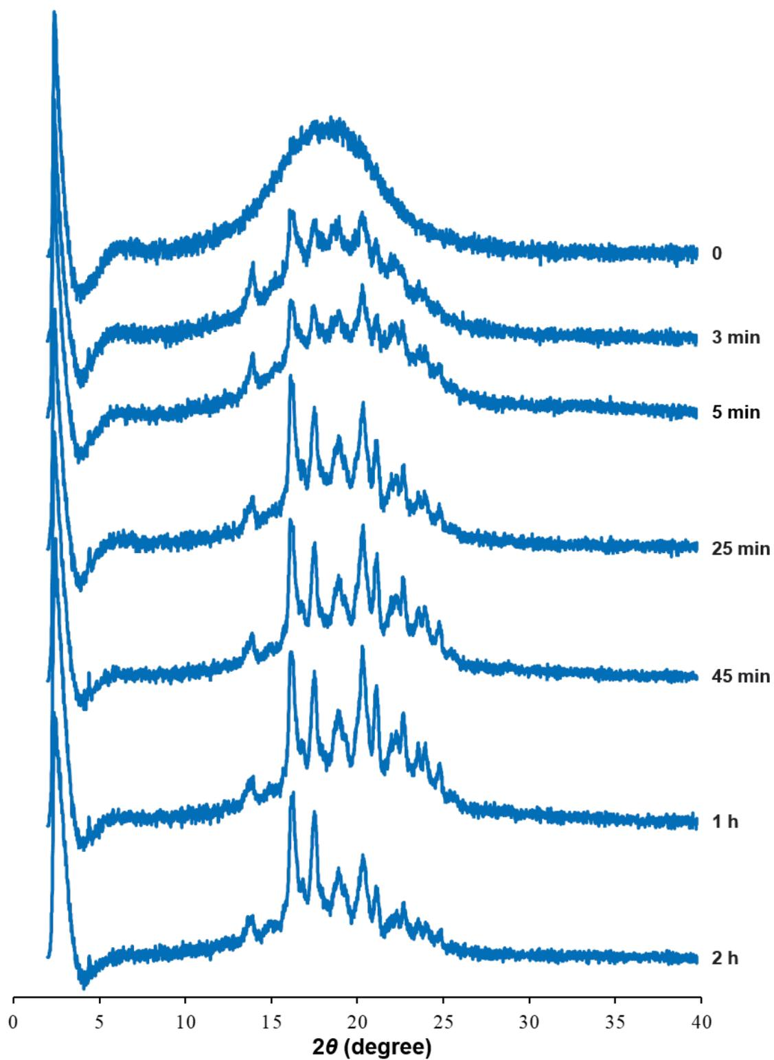
**Fig. S46** Time-dependent PXRD pattern changes of F5 by exposing  *$\alpha$* -F5 to *n*-pentane vapor.
