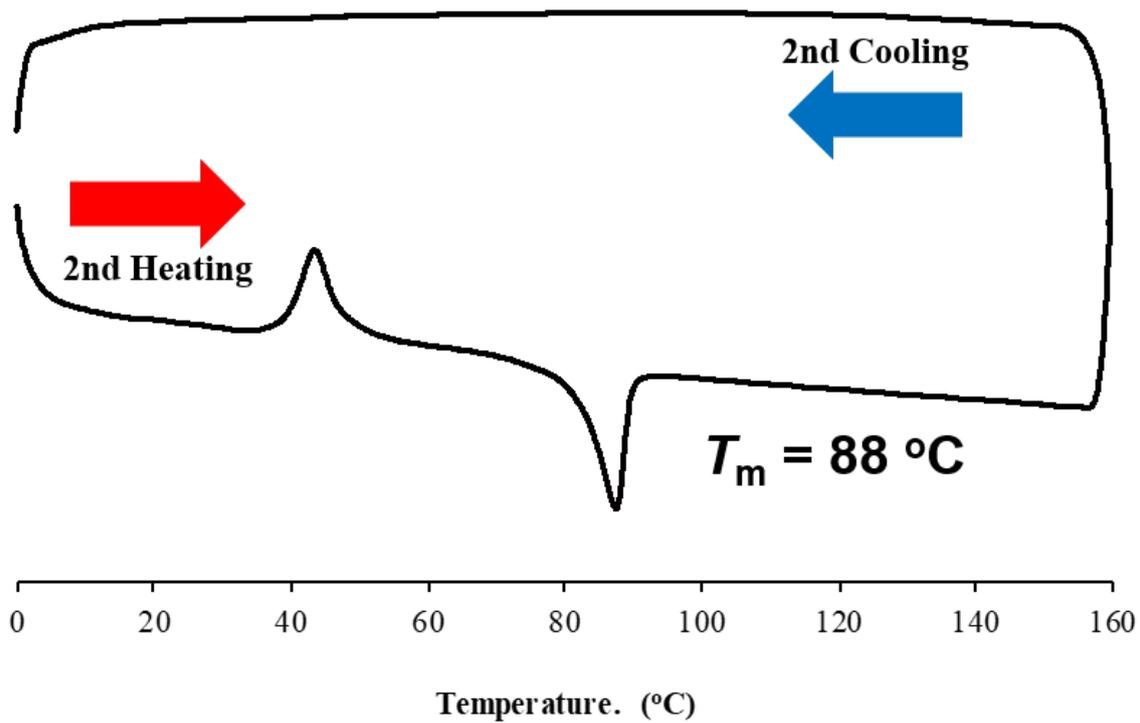
**Fig. S56** DSC second heating and cooling curve of [6]F5 (scanning rate: 10 °C/min).
