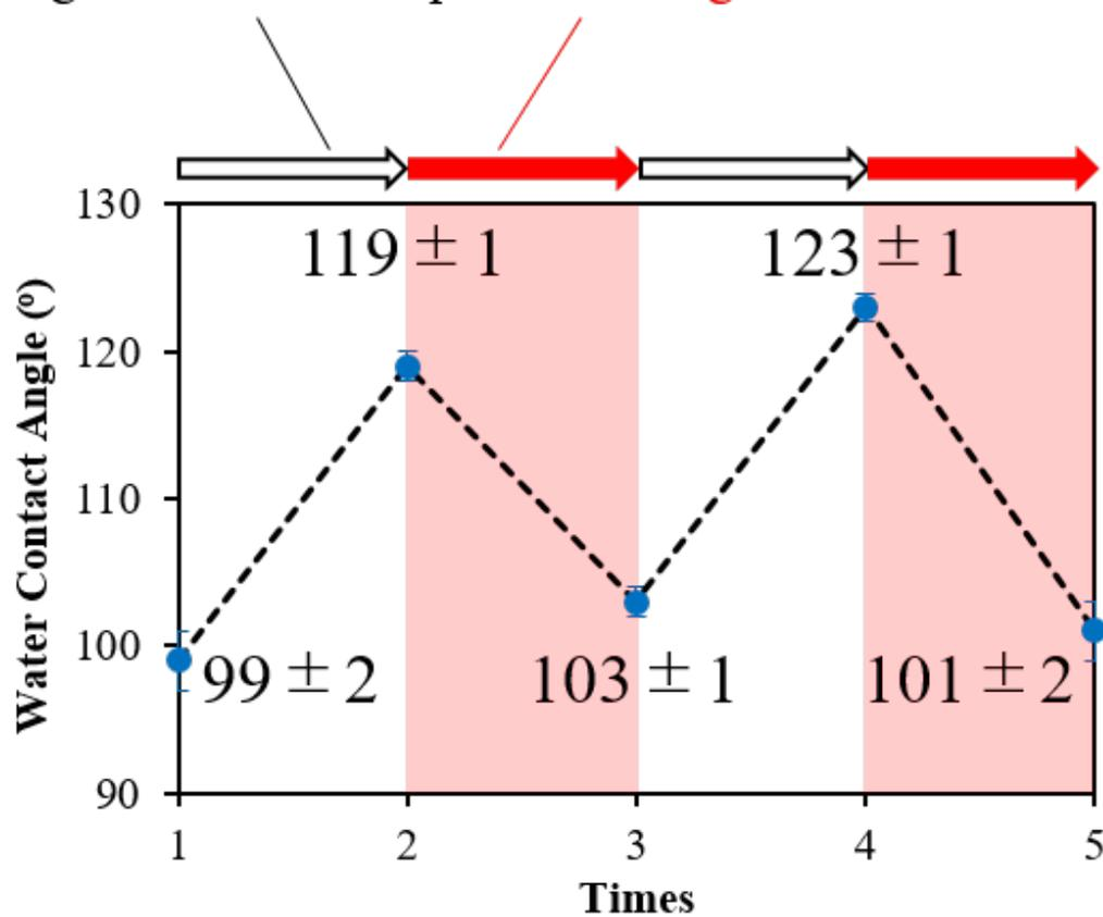
**Fig. S40** Water contact angle changes of F5 by exposing *a*-F5 to *n*-pentane vapor (odd times) and heating *c*-F5DP at 160 °C (even times). The error bars represent one standard error from five independent measurements.
