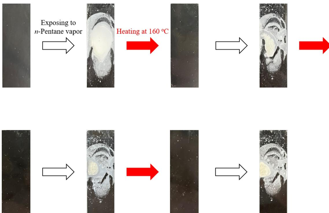
**Fig. S50** Photographs of **F5** by exposing  ***$\alpha$*** -**F5** to *n*-pentane vapor and heating  ***$c$*** -(**F5** $\supset$ **P**) at 160 °C repeatedly.
