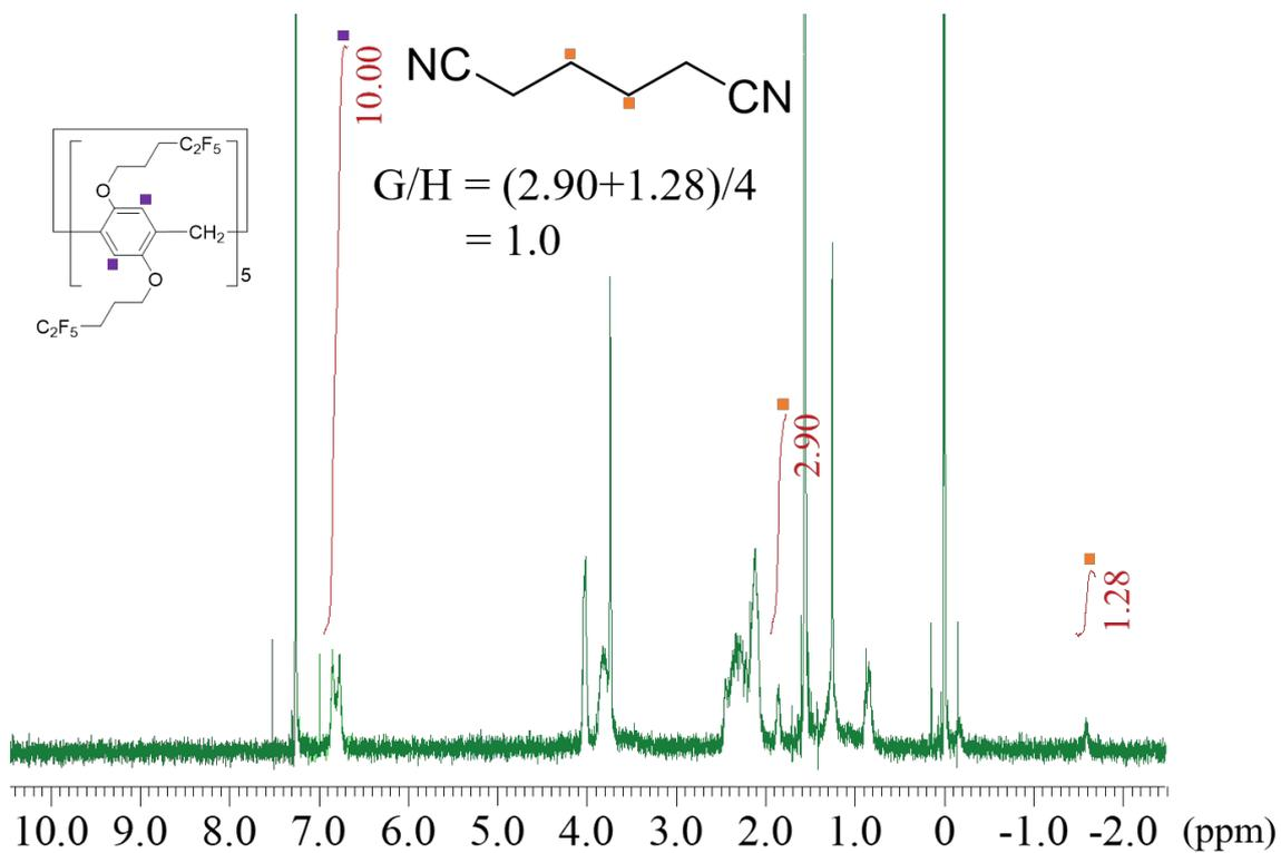
**Fig. S35**  $^1\text{H}$  NMR spectrum of *c*-(**F5-D1,4-Dicyanobutane**) ( $\text{CDCl}_3$ , 25 °C). The uptake ratio of 1,4-dicyanobutane to **F5** (G/H) calculated from the integration ratio was 1.0.
