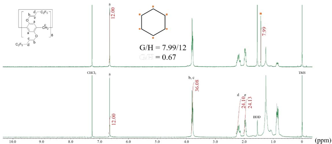
**Fig. S43**  $^1\text{H}$  NMR spectra of **[6]F5** ( $\text{CDCl}_3$ ,  $25\text{ }^\circ\text{C}$ ) before (lower side) and after (upper side) exposure to cyclohexane vapor. The uptake ratio of cyclohexane to **[6]F5** ( $G/H$ ) calculated from the integration ratio was 0.67.
