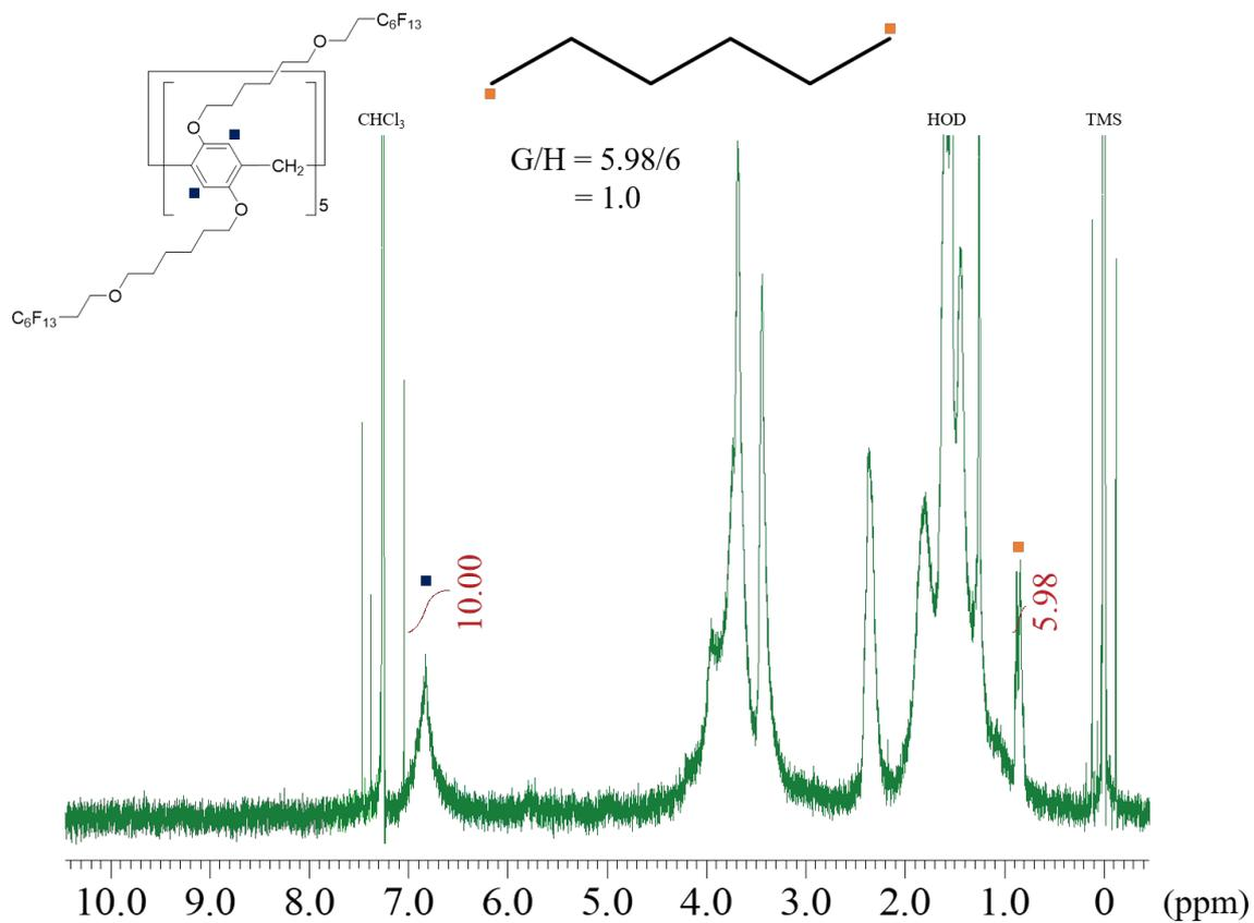
**Fig. S25** <sup>1</sup>H NMR spectrum of **F13** (CDCl<sub>3</sub>, 25 °C) before exposure to *n*-hexane vapor. The ratio of *n*-hexane to **F13** (G/H) calculated from the integration ratio was 1.0.
