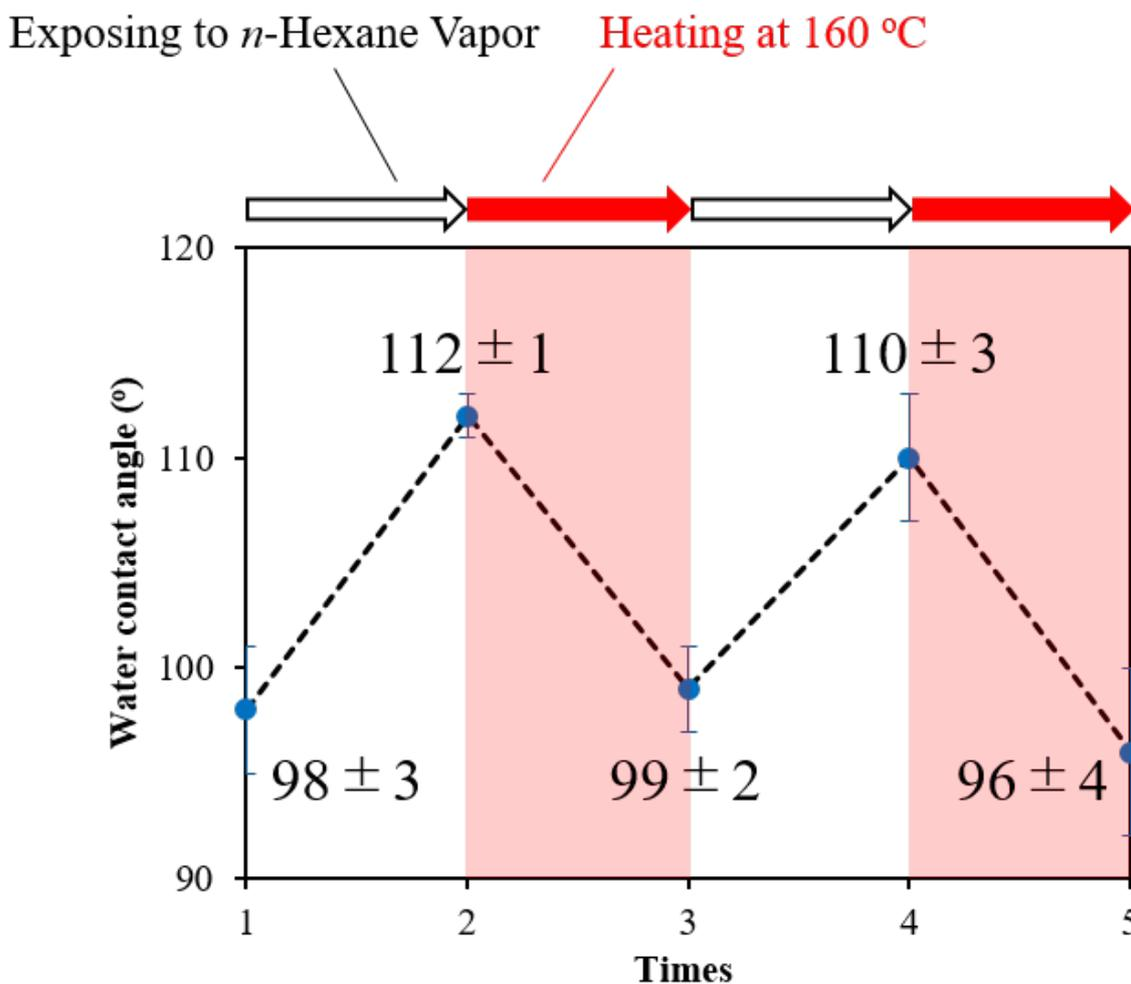
**Fig. S41** Water contact angle changes of **F5** by exposing *a*-**F5** to *n*-hexane vapor (odd times) and heating *c*-**(F5D)H** at 160 °C (even times). The error bars represent one standard error from five independent measurements.
