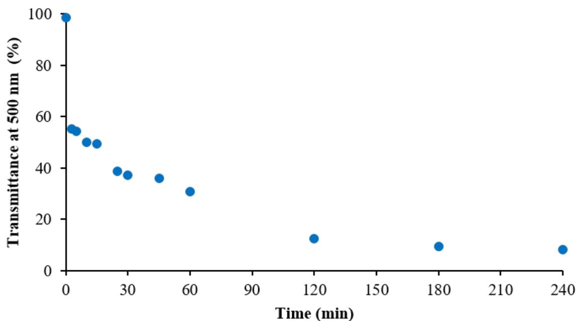
**Fig. S45** Time-dependent changes in transmittances at 500 nm of **F5** by exposing **a-F5** to *n*-pentane vapor.
