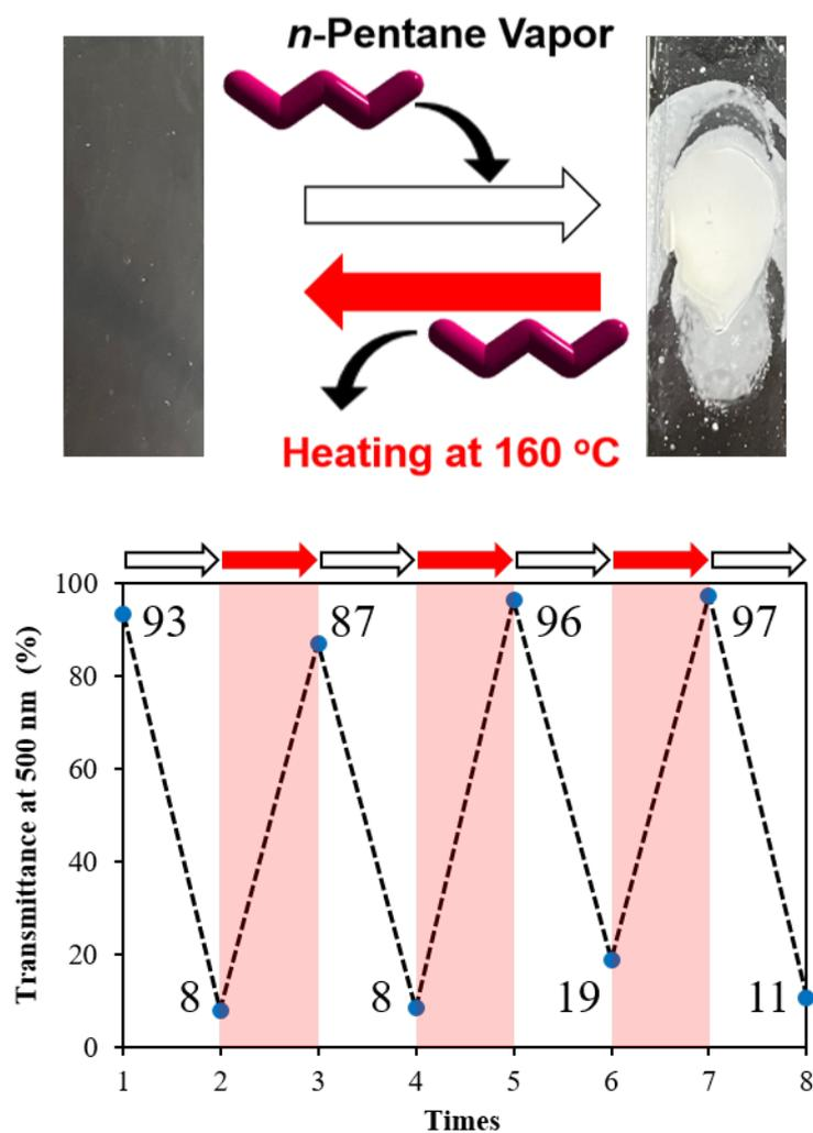
**Fig. S39** Photographs (upper side) and transmittance changes at 500 nm (lower side) of **F5** by exposing *a*-**F5** to *n*-pentane vapor (odd times) and heating *c*-(**F5**→**P**) at 160 °C (even times).
