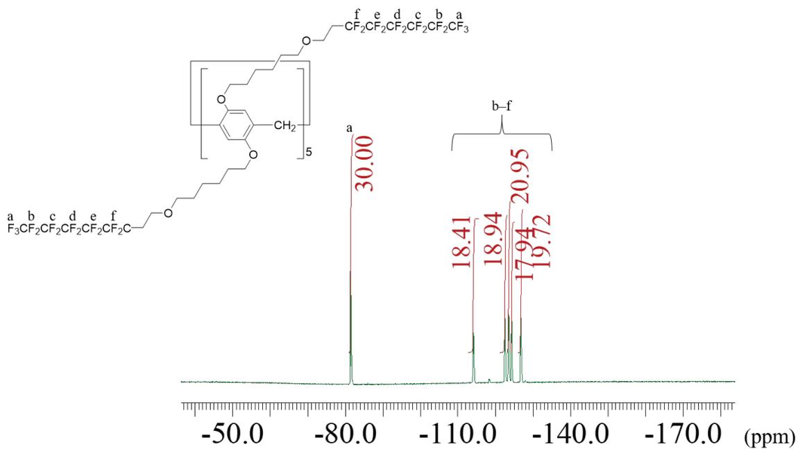
**Fig. S9**  $^{19}\text{F}$  NMR spectrum of F13 ( $\text{CDCl}_3$ , 25 °C).
