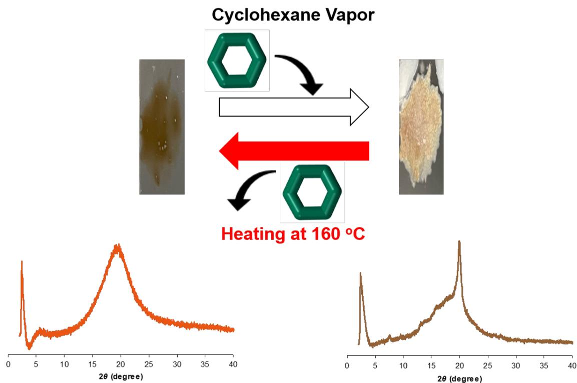
**Fig. S42** Photographs and PXR patterns of [6]F5 before (left) and after (right) exposure to cyclohexane vapor.
