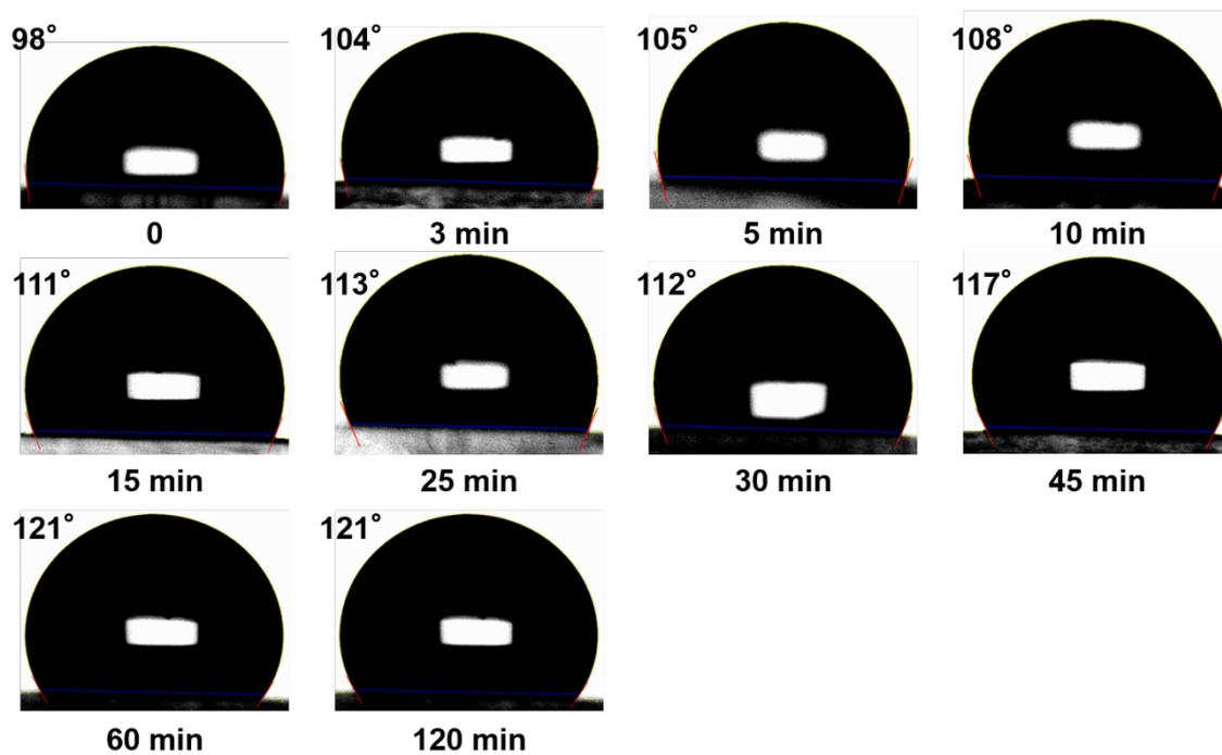
**Fig. S52** Photographs of time-dependent changes in water contact angles of **F5** by exposing  ***$\alpha$** -F5* to *n*-pentane vapor.
