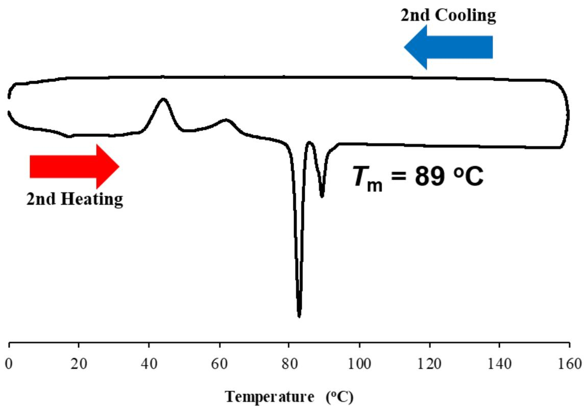
**Fig. S54** DSC second heating and cooling curve of C5 (scanning rate: 10 °C/min).
