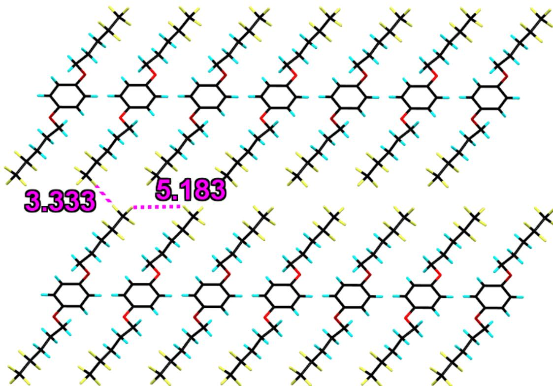
**Fig. S57** Single-crystal structures of (a) **F5D**H, (b) **F3D**H, (c) **C5D**H and (d) **Monomer Unit** (prepared from chloroform under *n*-hexane vapor); all labeled distances between intermolecular fluorine atoms are given in angstrom orders. F, O, C and H atoms are represented by yellow, red, black and light blue capped sticks, respectively. Guest molecules are omitted for clarity.
