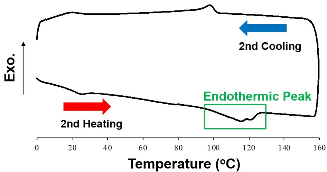
**Fig. S17** DSC second heating and cooling curve of *c*-F5 (scanning rate: 10 °C/min).
