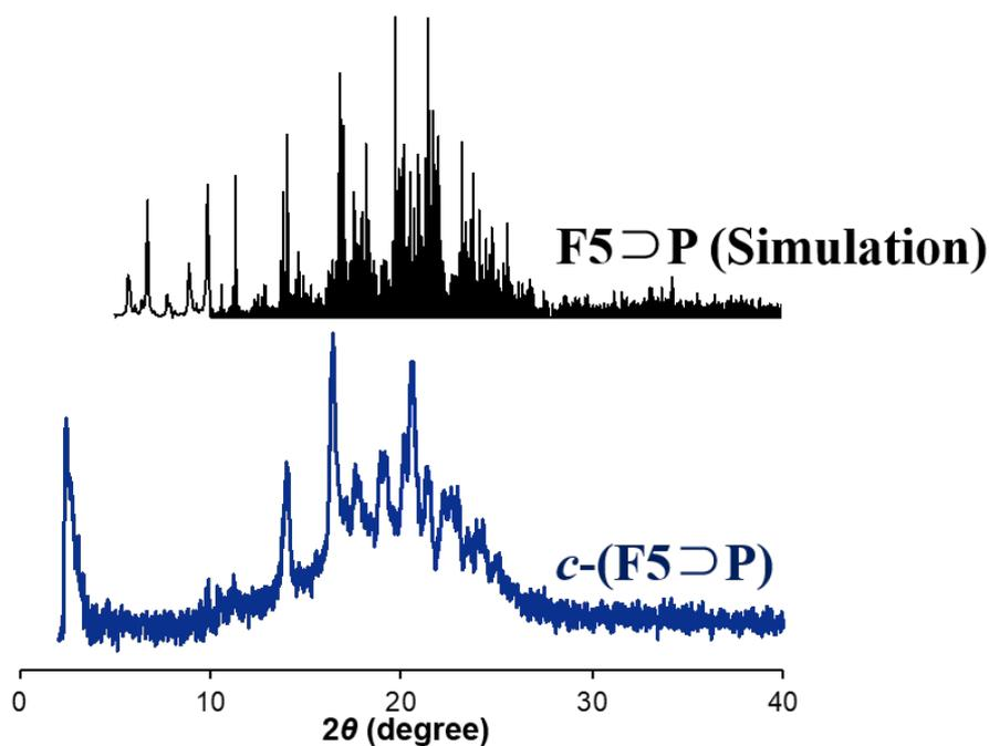
**Fig. S48** PXRD patterns of simulation from single crystal of  $F5\supset P$  (upper side) and  $c\text{-}(F5\supset P)$  (lower side).
