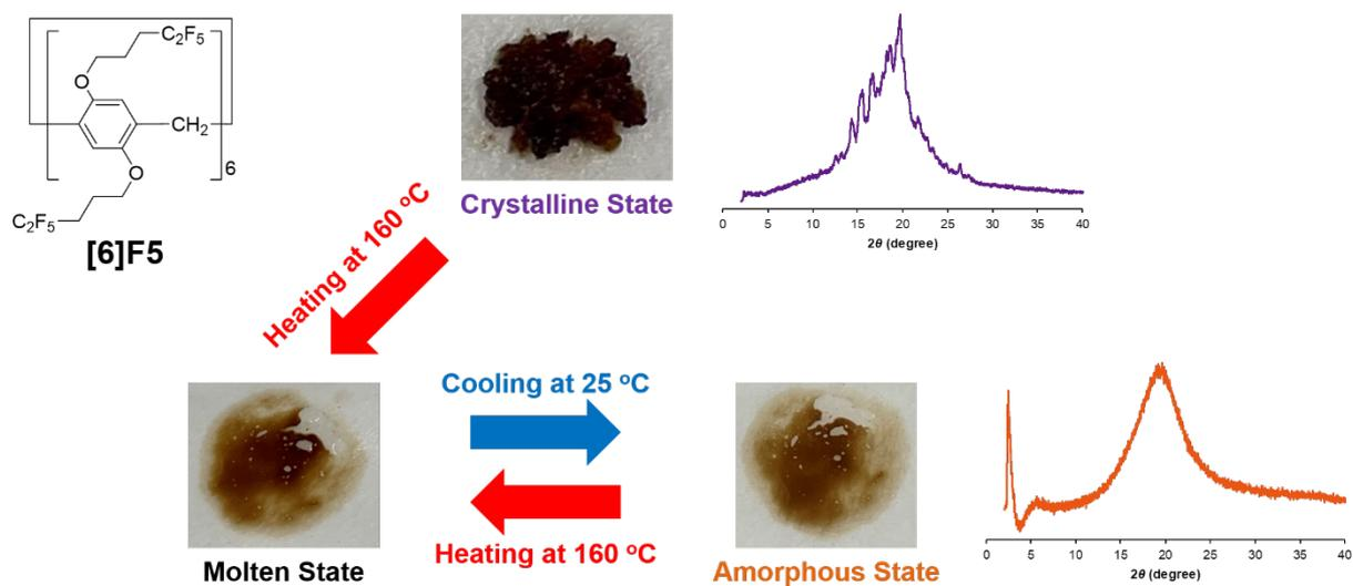
**Fig. S20** Photographs and PXRD patterns of [6]F5 before and after heating over melting points and then cooling at 25 °C.
