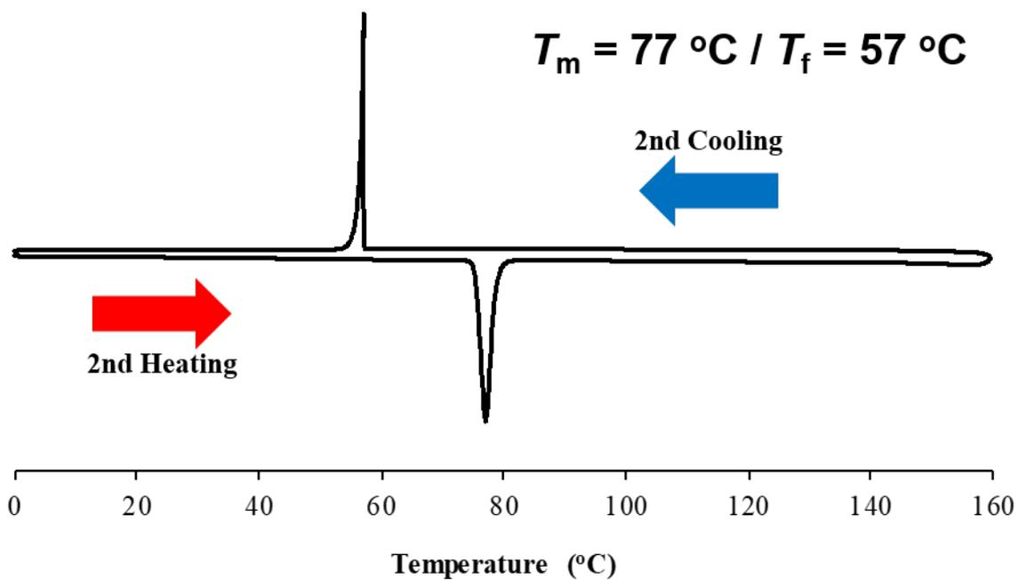
Fig. S55 DSC second heating and cooling curve of **Monomer Unit** (scanning rate: 10 °C/min).
