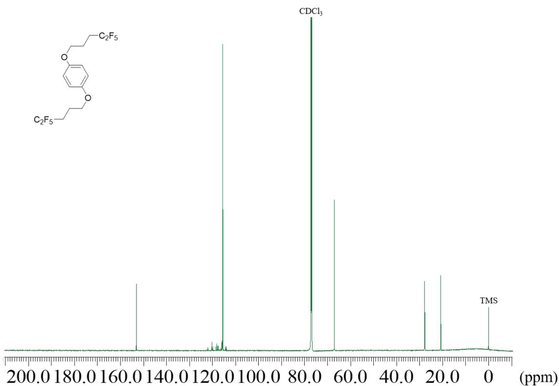
**Fig. S11**  $^{13}\text{C}$  NMR spectrum of **Monomer Unit** ( $\text{CDCl}_3$ ,  $25^\circ\text{C}$ ).
