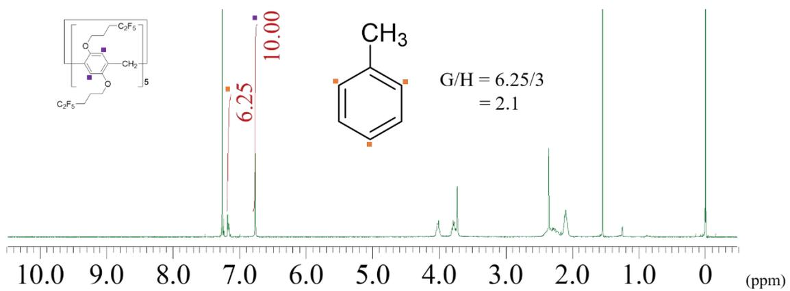
**Fig. S34**  $^1\text{H}$  NMR spectrum of *c*-(**F5**)Toluene) ( $\text{CDCl}_3$ , 25 °C). The uptake ratio of toluene to **F5** (G/H) calculated from the integration ratio was 2.1.
