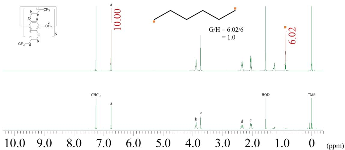
**Fig. S23**  $^1\text{H}$  NMR spectra of **F3** ( $\text{CDCl}_3$ , 25  $^\circ\text{C}$ ) before (lower side) and after (upper side) exposure to *n*-hexane vapor. The uptake ratio of *n*-hexane to **F3** (G/H) calculated from the integration ratio was 1.0.
