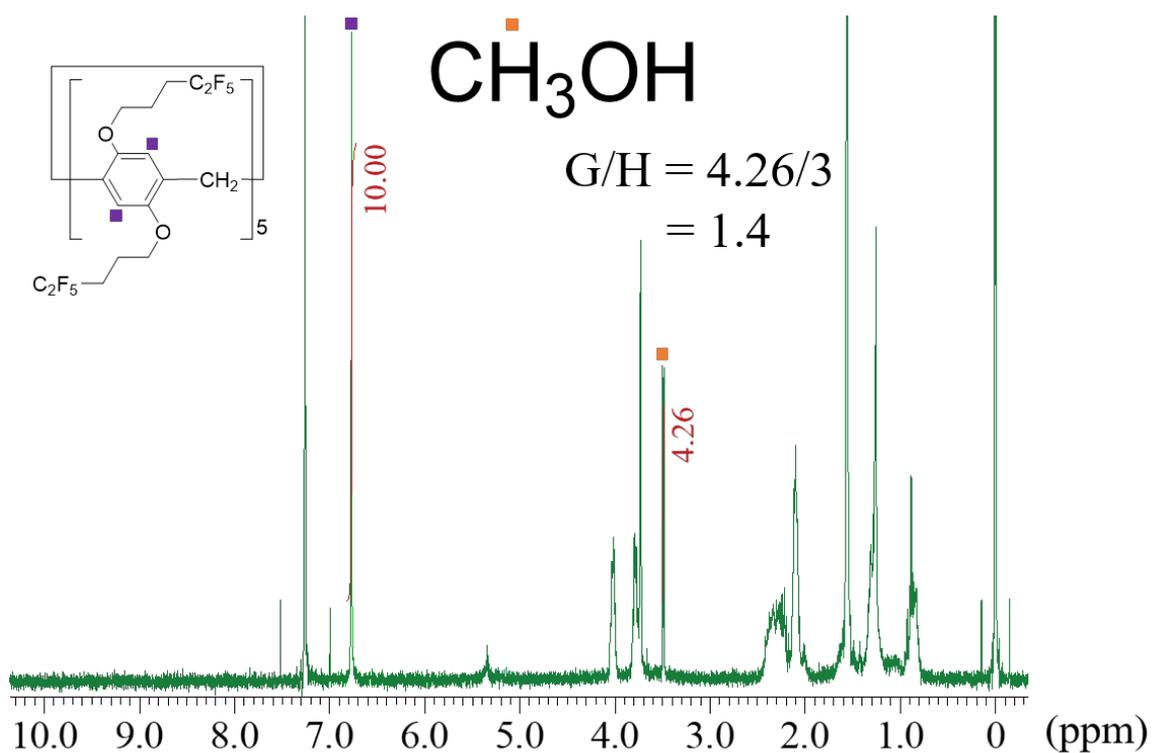
**Fig. S32** <sup>1</sup>H NMR spectrum of *c*-(F5)Methanol) (CDCl<sub>3</sub>, 25 °C). The uptake ratio of methanol to F5 (G/H) calculated from the integration ratio was 1.4.
