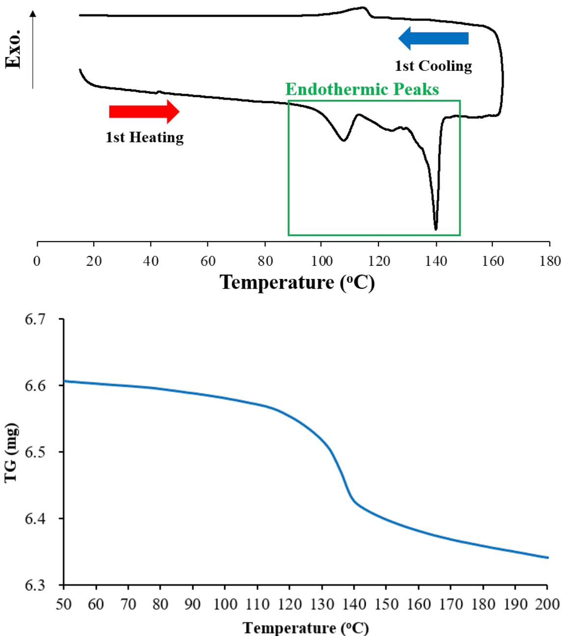
**Fig. S27** DSC first heating and cooling curve (upper side) and TG trace (lower side) of *c*-(F5D)H) (scanning rates of DSC and TDA: 10 °C/min).
