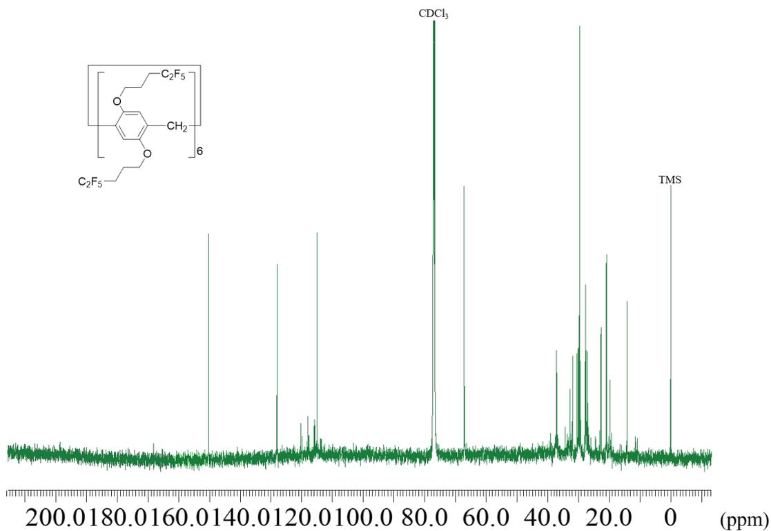
**Fig. S14**  $^{13}\text{C}$  NMR spectrum of [6]F5 ( $\text{CDCl}_3$ , 25 °C).
