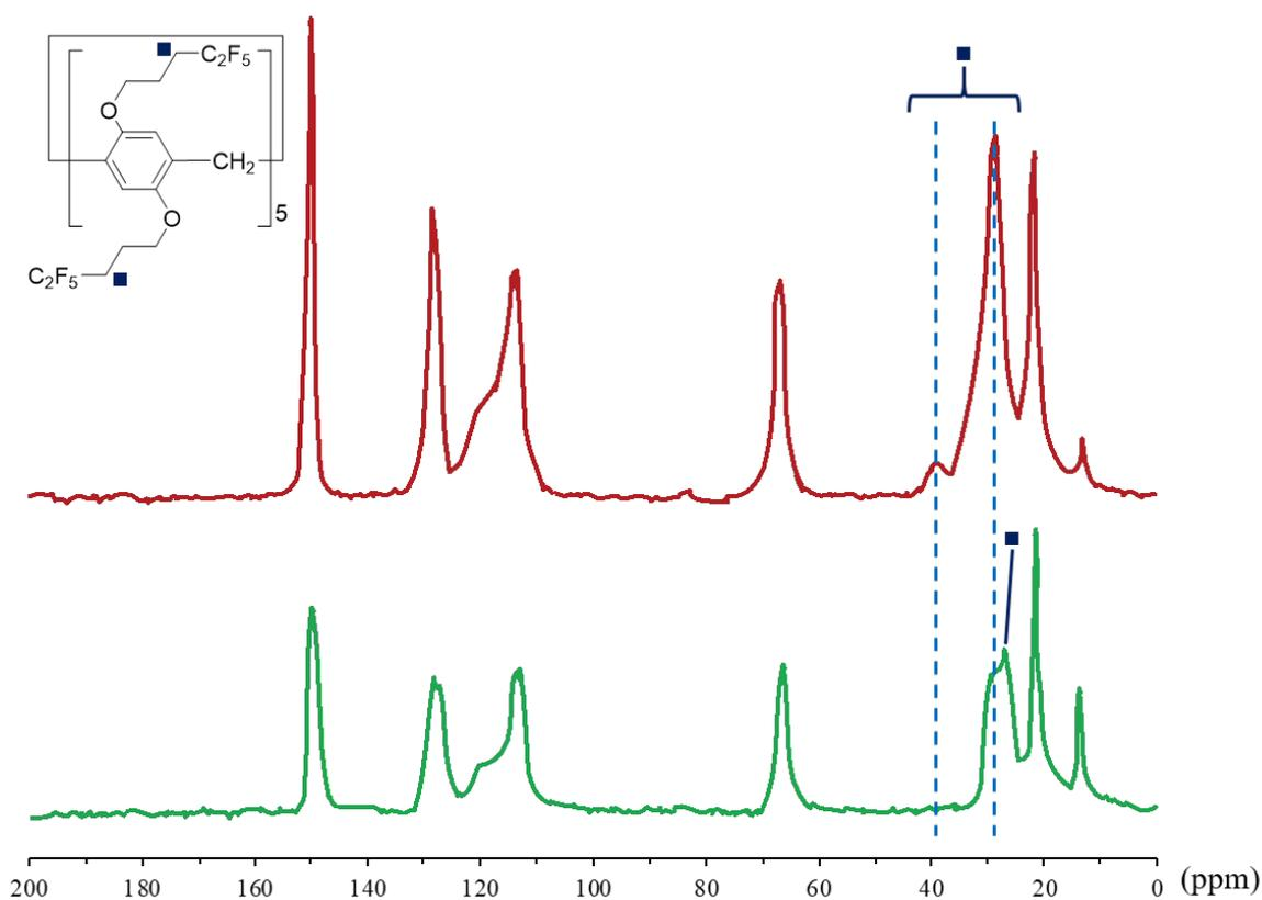
**Fig. S29** Solid-state  $^{13}\text{C}$  NMR spectra of *a*-F5 (upper side) and *c*-(F5D)H (lower side).
