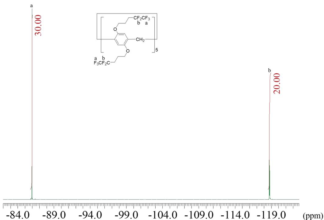
**Fig. S3**  $^{19}\text{F}$  NMR spectrum of **F5** ( $\text{CDCl}_3$ , 25 °C).
