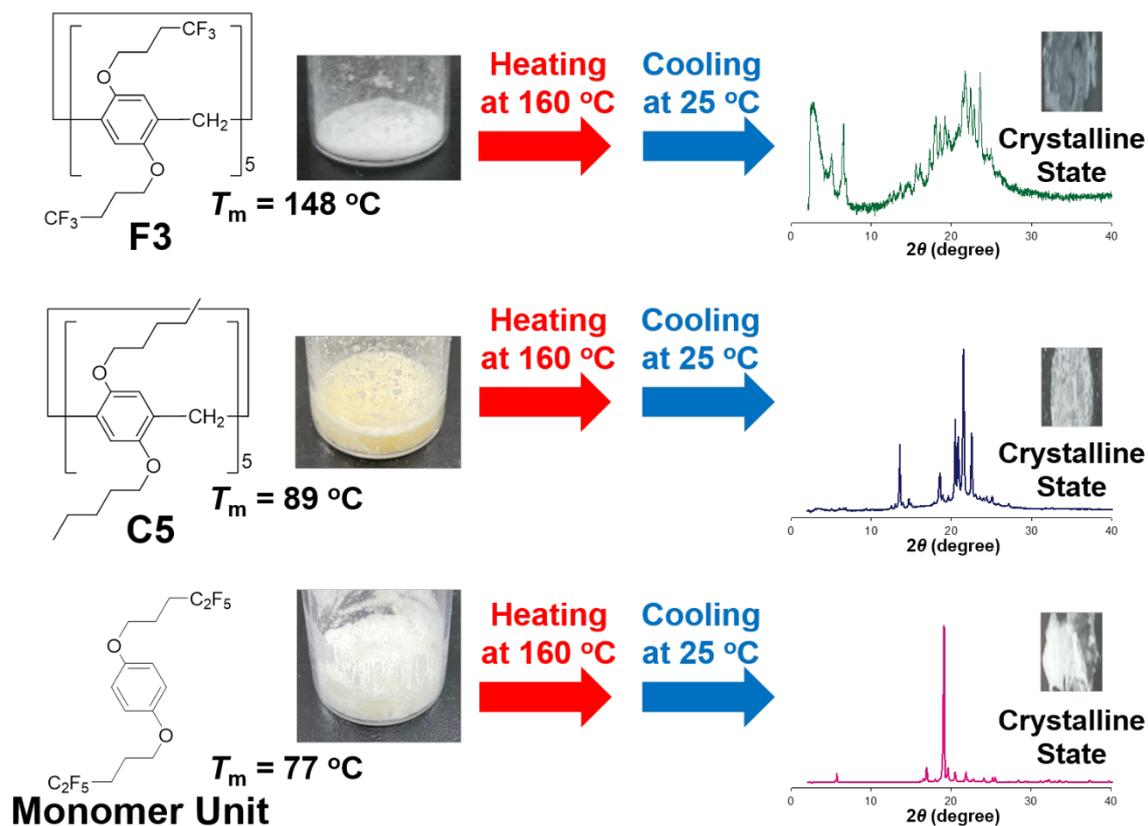
**Fig. S18** Photographs and PXRD patterns of **F3** (top), **C5** (middle) and **Monomer Unit** (bottom) before (left) and after (right) heating over melting points and then cooling at 25 °C.
