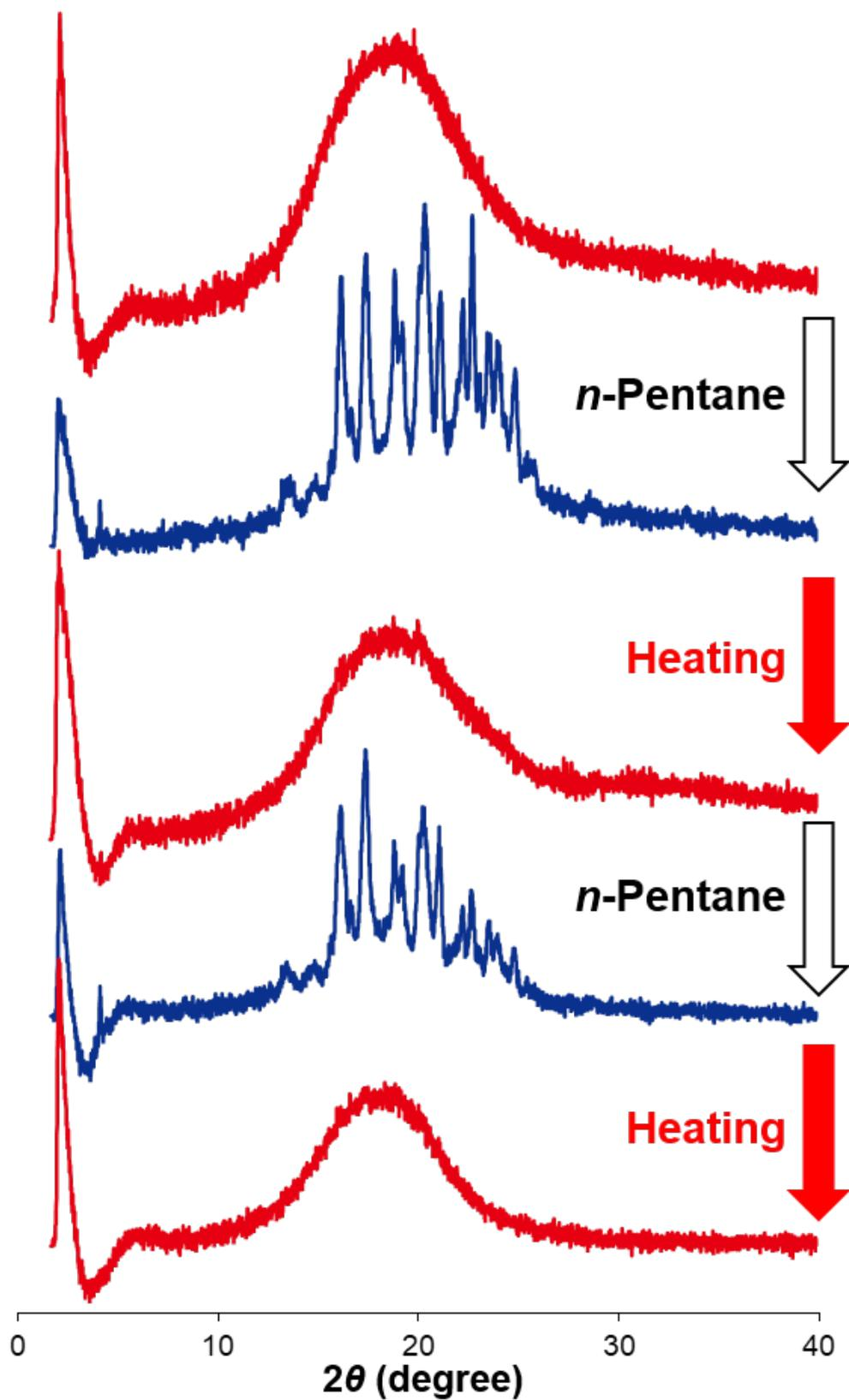
Fig. S38 PXRD patterns of F5 by exposing *a*-F5 to *n*-pentane vapor and heating *c*-(F5 $\Rightarrow$ P) at 160 °C.
