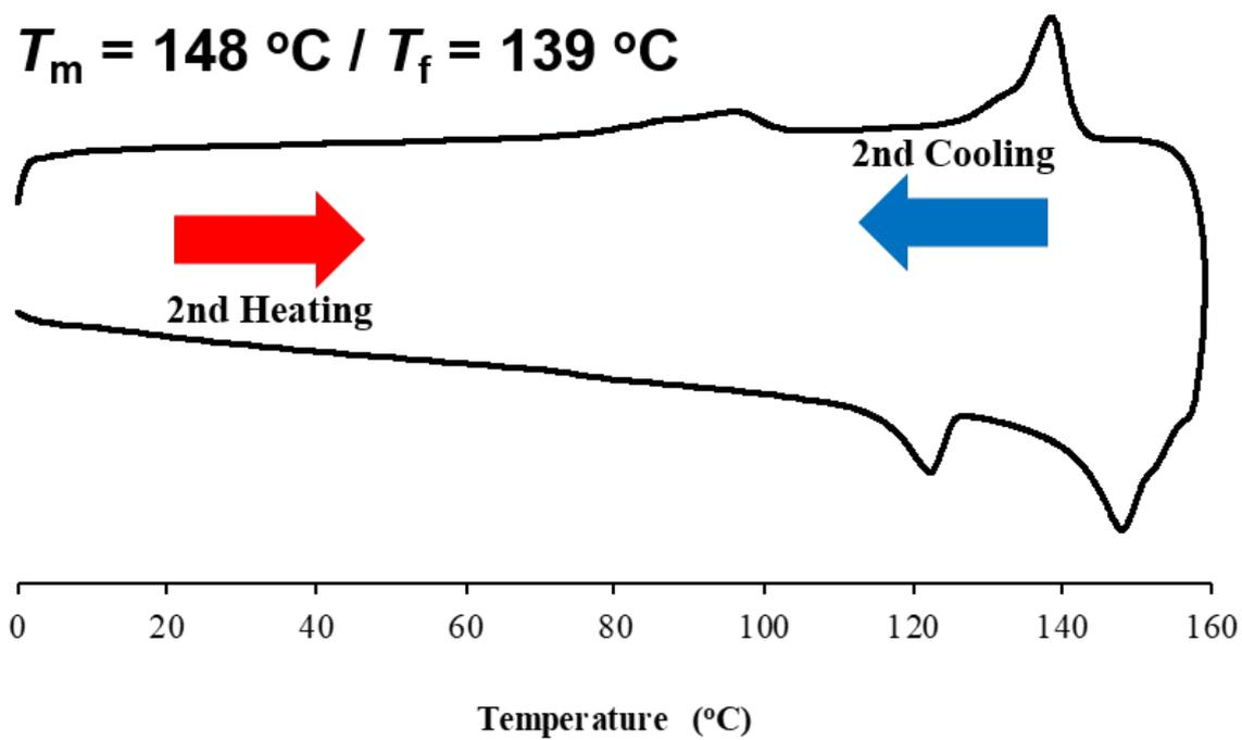
Fig. S53 DSC second heating and cooling curve of F3 (scanning rate: 10 °C/min).
