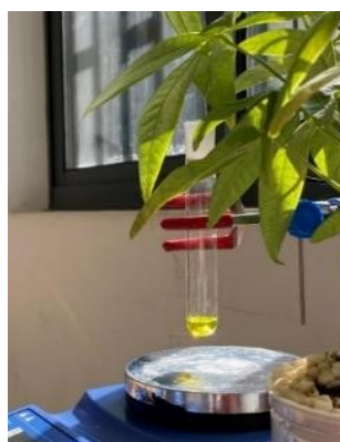
Figure S27. Efficient conversion of amines to imines under sunlight in an air atmosphere.
