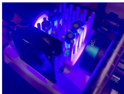
Figure S1. Reaction setup for the photoinduced two-component Minisci alkylation reaction
