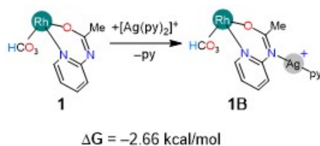
Figure S4. Thermodynamic change with coordination of \text{Ag}(\text{pyridine})_2 to complex 1 .
