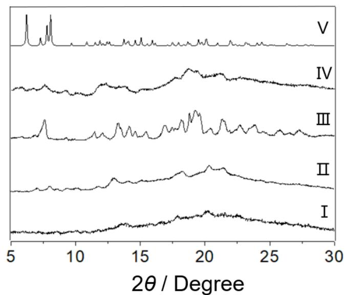
**Fig. S31** The PXRD patterns of I) original **cagearene-1**; II) after adsorption of Cy vapour; III) after adsorption of Bz vapour; IV) after adsorption of Bz/Cy (50:50 v/v) mixture vapour; V) simulated pattern from the single-crystal structure of **Bz@cagearene-1**.
