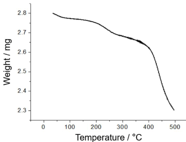
**Fig. S26** TGA of the activated **cagearene-1** solid.
