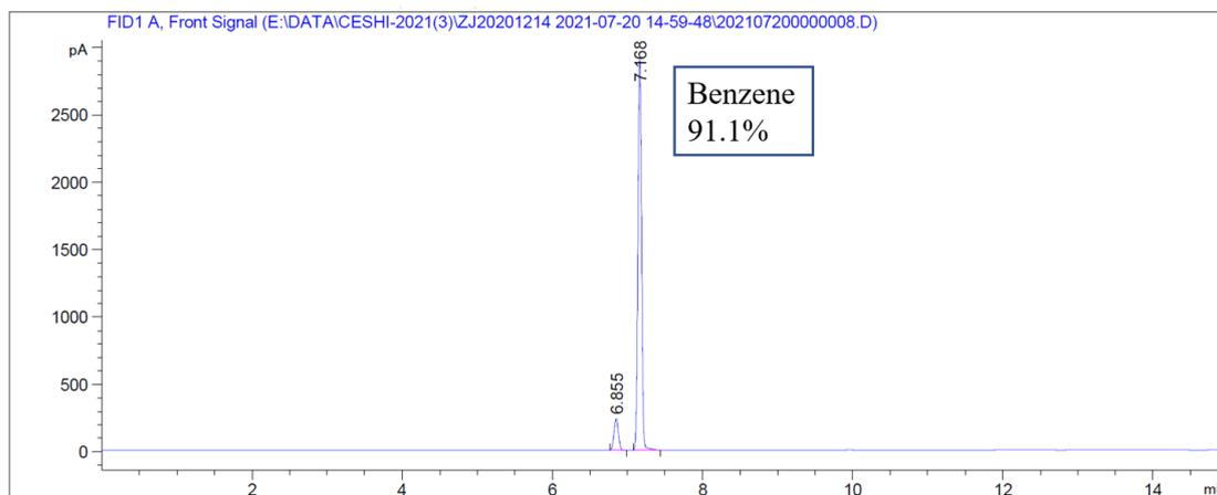
**Fig. S29** Percentage of Bz measured by gas chromatography after absorbing a Bz/Cy mixture (50:50 v/v) by **cagearene-1** solid for 12 hours.
