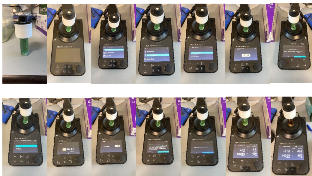
Fig S14. Example of the ElectroSyn interface used to set the reaction parameters. Here a potentiostatic reaction at E_{app} = -0.16 \text{ V} is demonstrated. The observed colour change from green to brown is attributed to electrochemical reduction of Cu II (NPPI) 2 (green) to Cu I (NPPI) 2 (brown).
