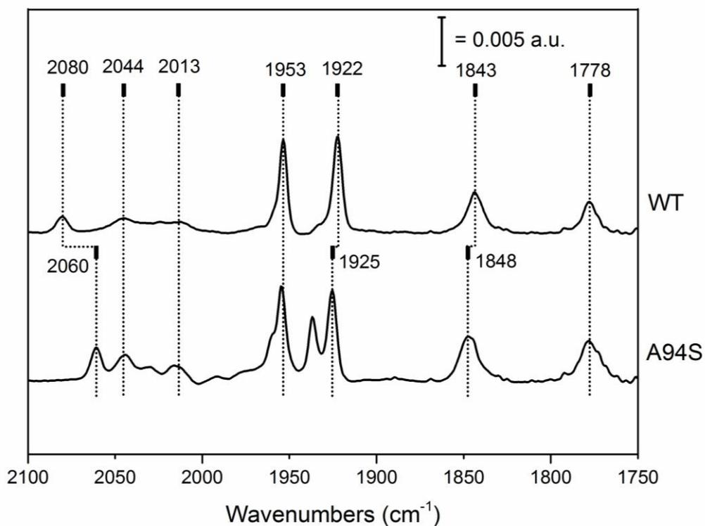
Fig. S3 Effect of the A94S mutation on the FTIR spectrum of 2-HydA1. Room temperature ATR-FTIR spectra obtained for 2-HydA1 (WT) and for the A94S mutant. The frequencies of the most prominent bands are given and their shifts can be followed through dotted lines. Spectra are recorded on semi-dry films on an ATR-FTIR crystal, at room temperature and with  $2 \text{ cm}^{-1}$  spectral resolution.
