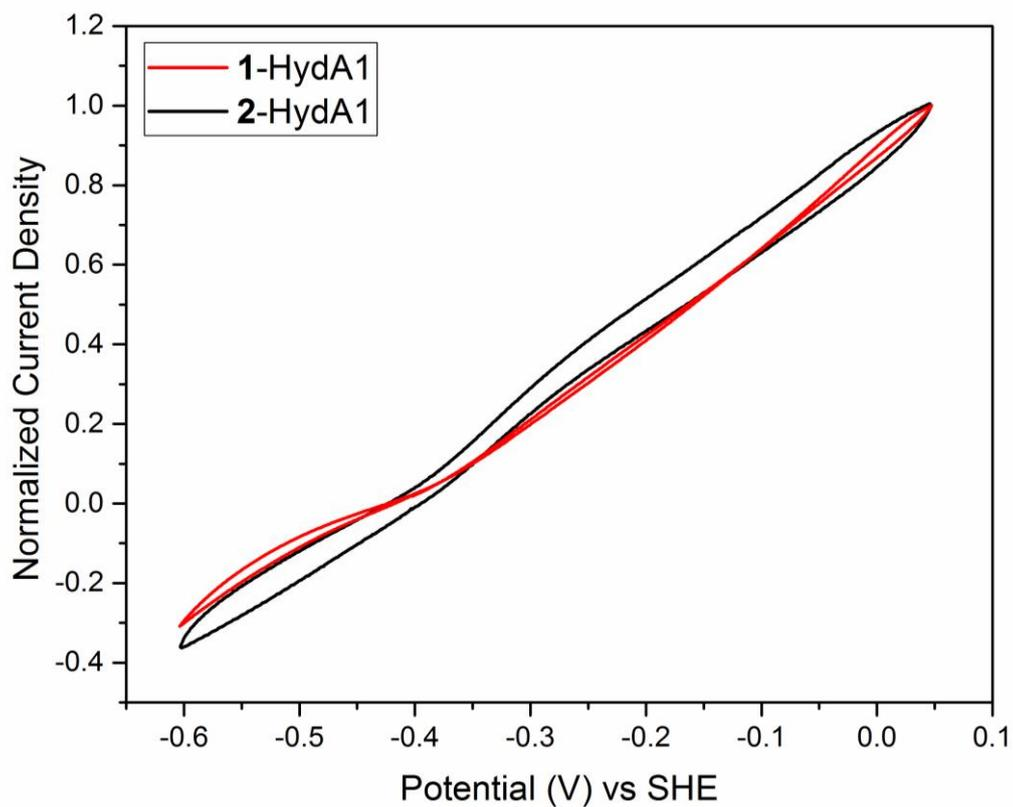
Fig. S7 Cyclic voltammograms with normalized currents for 1-HydA1 and 2-HydA1. Cyclic voltammograms of 2-HydA1 (black trace) and 1-HydA1 (red trace) films absorbed on a rotating-disk PGE electrode, measured in pH 7 Buffer Mix under 1 atm H<sub>2</sub> gas, scan rate: 10mV/s, temperature: 30°C and rotation rate: 3000 rpm. Current were normalized at their maximum positive value, at 0.05 mV vs SHE.
