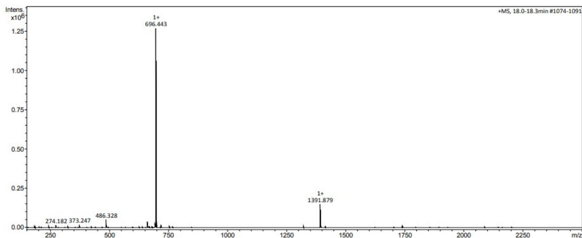
**Figure S2.** Deconvoluted mass spectrum of  $N_3$ -ILVAGK-NH<sub>2</sub>. Calculated for C<sub>31</sub>H<sub>57</sub>N<sub>11</sub>O<sub>7</sub> 695.452, found 696.443 [M + H]<sup>+</sup>.
