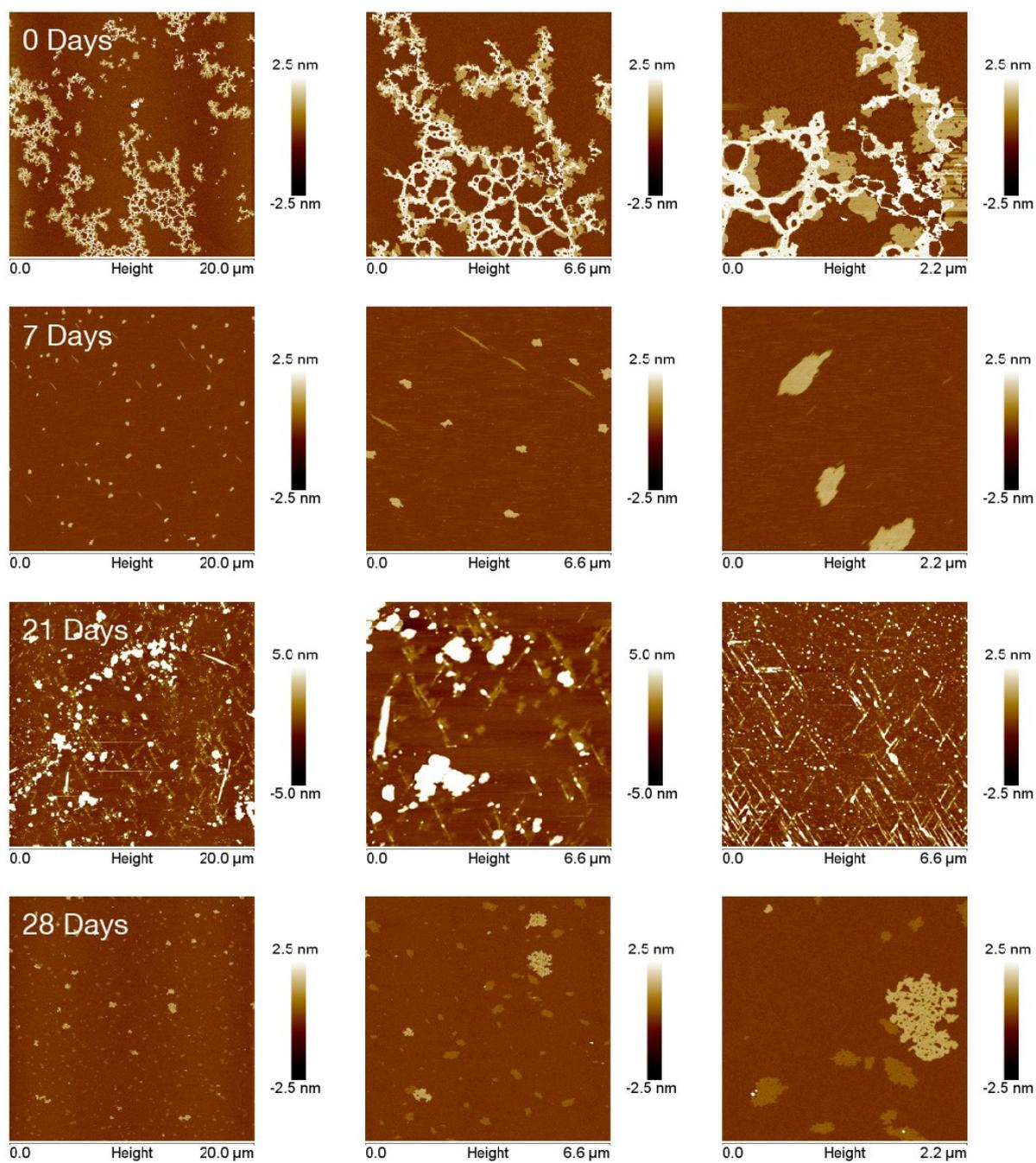
**Figure S23.** AFM images of ILVAGK over 28 days of aging, deposited from 1% SDS.
