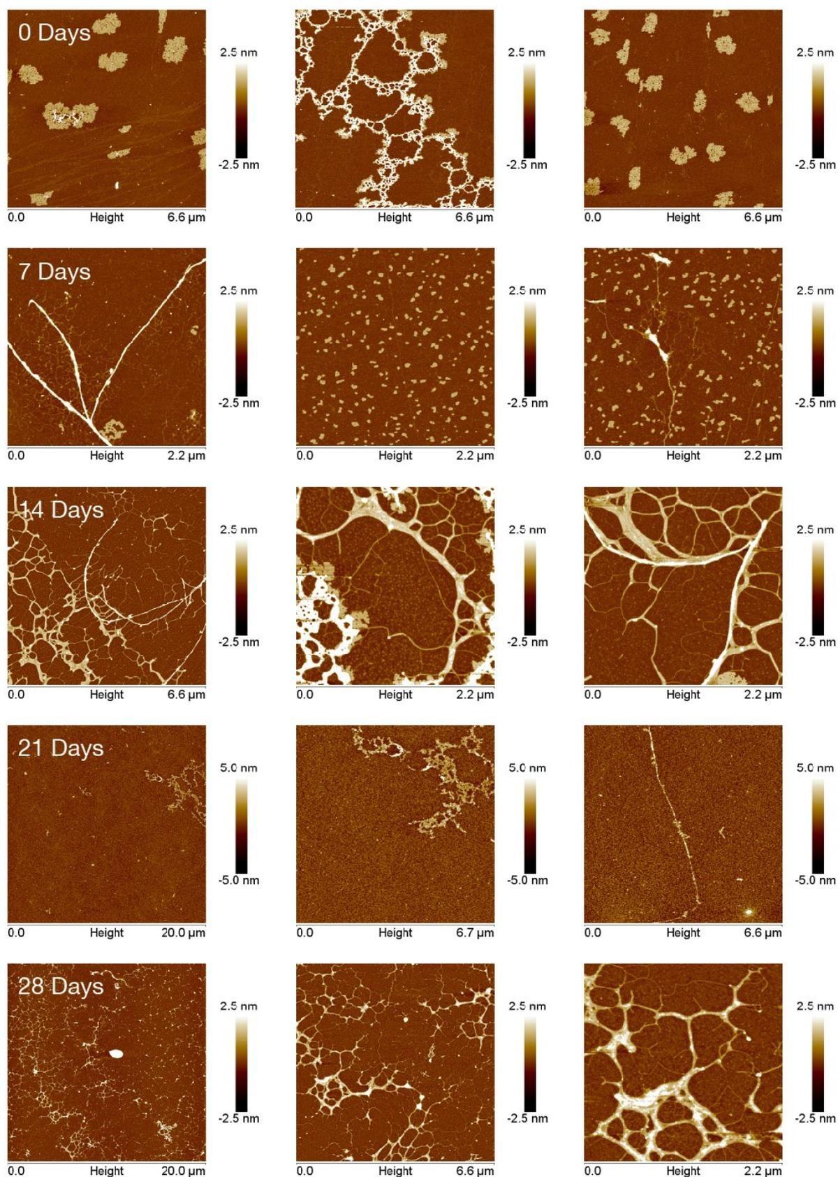
**Figure S19.** AFM images of 1:1 mixture of DNA A and IVLAGK in 1x TAMg buffer over 28 days of aging after thermocycling.
