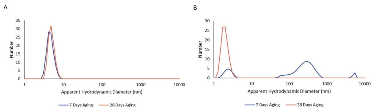
**Figure S20.** DLS data for study 3. A: **A'-ILVAGK + A**, B: **ILVAGK**. All measured in 1 % SDS buffer and at a concentration of 10  $\mu\text{M}$ .
