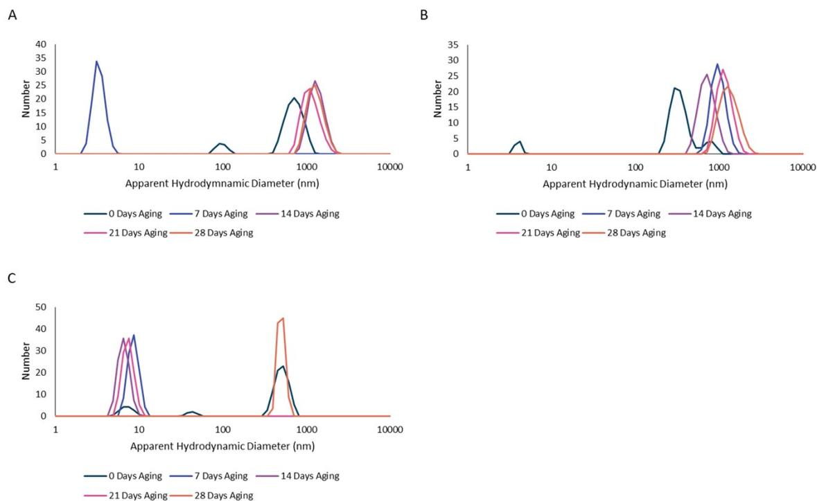
**Figure S14.** DLS data for Study 2. A: **A-ILVAGK + A'**, B: **A-ILVAGK + 2A'**, and C: **A-ILVAGK + 3A'**. All measured in TAMg buffer and at a concentration of 10  $\mu\text{M}$ .
