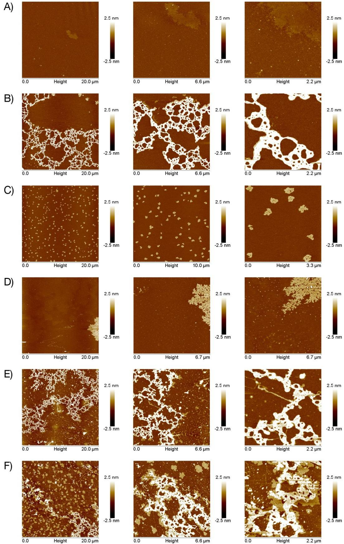
**Figure S26.** AFM images of DNA controls in 1x TAMg buffer over 28 days of aging. A: 1x TAMg, B: A, C: A', D: A+A', E: 2A' and F: 3A'.
