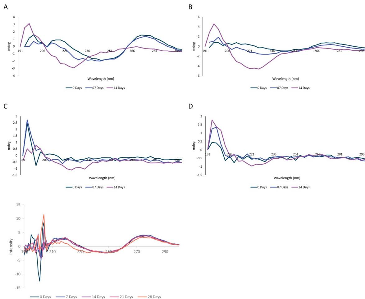
**Figure S7.** CD spectra for Study 1, A: 1:1, B: 1:0.5, C: 1:0.1, D: 1:0.01, E: 0:1 ratios of **ILVAGK:A'-ILVAGK**. All measured in TAMg buffer and at a concentration of 10  $\mu$ M. Missing time points occurred due to Covid-19 related lab closures. Excessive absorption was observed with the pure **A'-ILVAGK** sample, leading to noise in the CD spectrum below 210 nm which occludes any real signal in that range.
