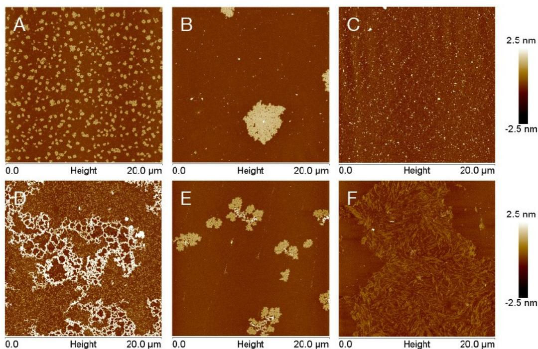
**Figure S1.** Morphologies within this paper. A: Small flakes, B: large flakes, C: dot-like, D: network-like, E: fractal-like and F: fibre-like.
