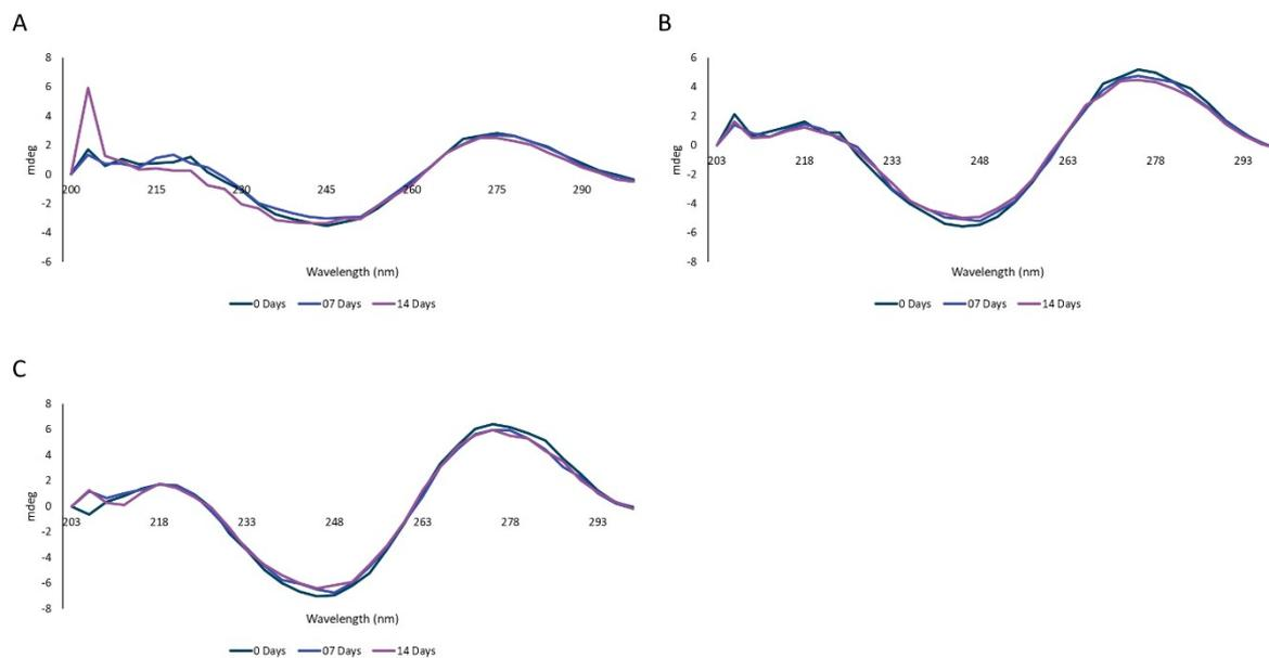
**Figure S15.** CD spectra for Study 1, A: **A-ILVAGK + A'**; B: **A-ILVAGK + 2A'**; and C: **A-ILVAGK + 3A'** All measured in TAMg buffer and at a concentration of 10  $\mu$ M.
