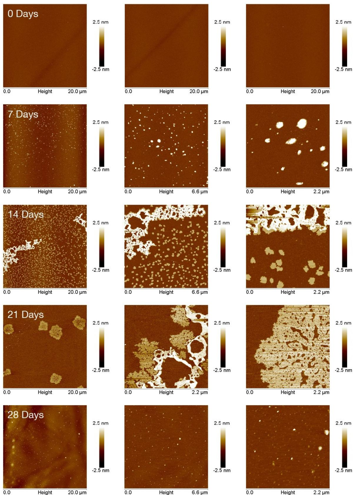
**Figure S13.** AFM images of ILVAGK in 1x TAMg buffer over 28 days of aging (no thermocycling).
