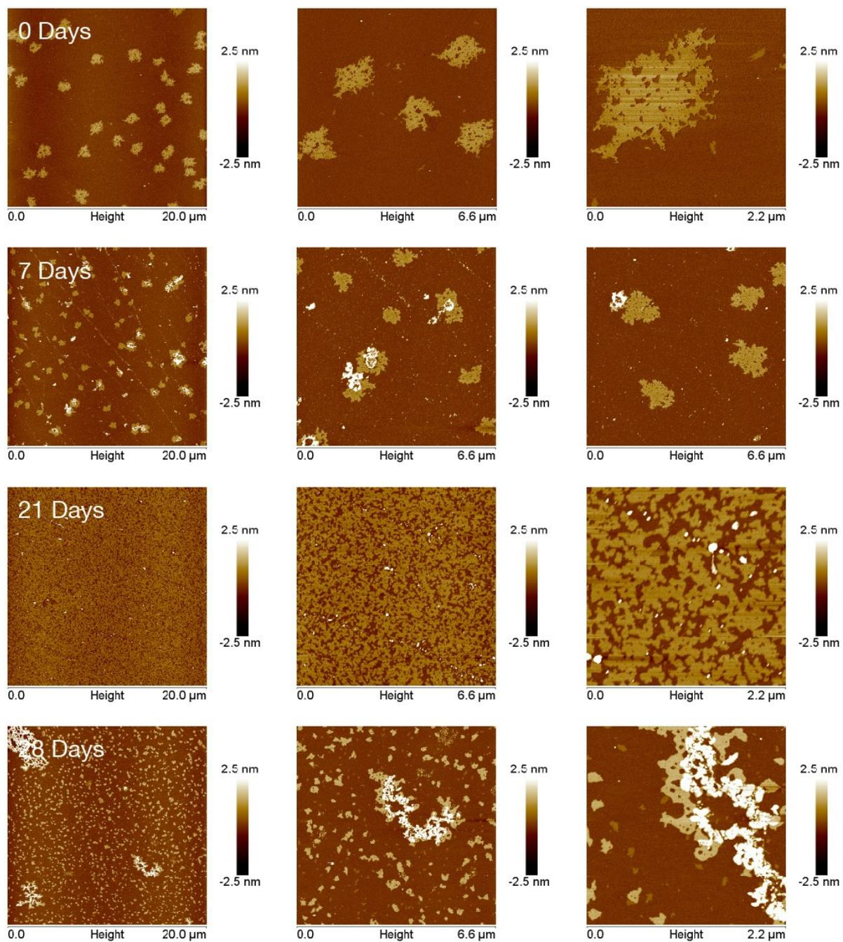
Figure S22. AFM images of sample A'-ILVAGK + A over 28 days of aging, deposited from 1% SDS.
