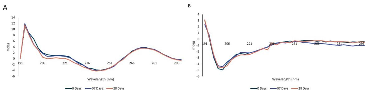
**Figure S21.** CD spectra for A: **A'-ILVAGK + A**, B: **ILVAGK**. All measured in 1 % SDS buffer and at a concentration of 10  $\mu\text{M}$ .
