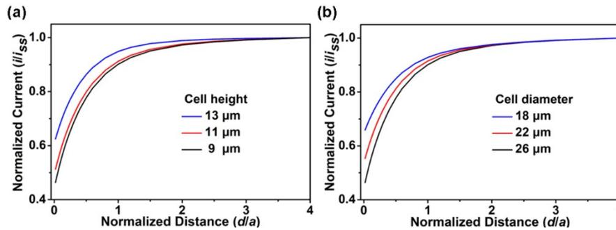
**Fig. S4** Simulated SECM approach curves towards cells with (a) different heights (diameter = 13  $\mu\text{m}$ ) and (b) different widths (height = 9  $\mu\text{m}$ ).
