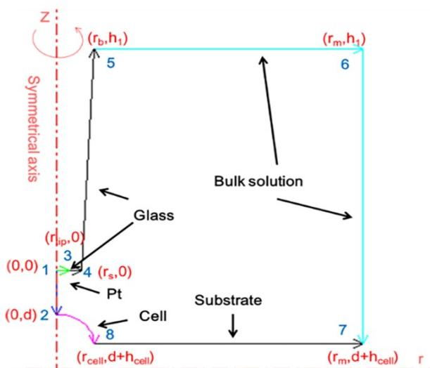
**Fig. S2** An illustration of the 2D axial SECM geometry simulation for the cell.
