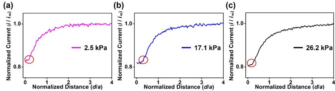
**Fig. S3** SECM approach curves to the PA gels with the stiffnesses of (a) 2.5, (b) 17.1 and (c) 26.2 kPa, respectively.
