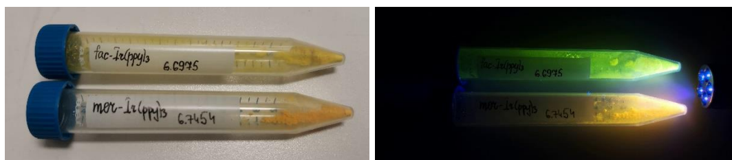
Figure S56. Photo images of starting material fac -Ir(ppy) 3 and the product mer -Ir(ppy) 3 under daylight (left) and under irradiation at 365 nm (right).
