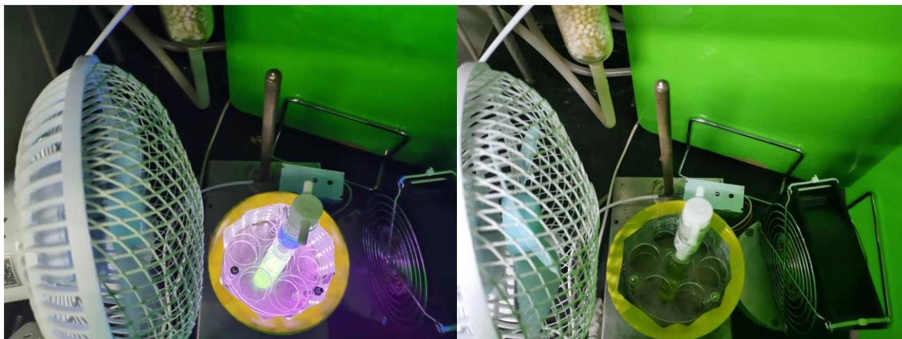
Photoreactor scaled as 100 W BLUE LED.
