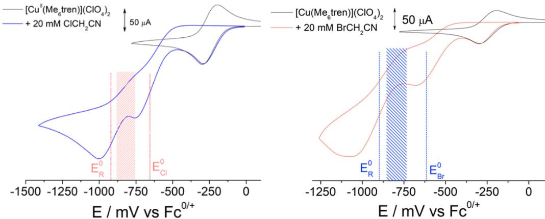
**Figure S2.** Cyclic voltammetry of  $[\text{Cu}(\text{Me}_6\text{tren})(\text{NCCH}_3)]^{2+}$  in the absence and presence of  $\text{XCH}_2\text{CN}$  ( $\text{X} = \text{Cl}$  (**1a**) or  $\text{Br}$  (**1b**)). The electrolysis potential ( $E_{\text{app}}$ ) lies within the shaded band shown on each voltammogram ( $E_{\text{R}} < E_{\text{app}} < E_{\text{X}}$ ,  $\text{X} = \text{Cl}, \text{Br}$ ).
