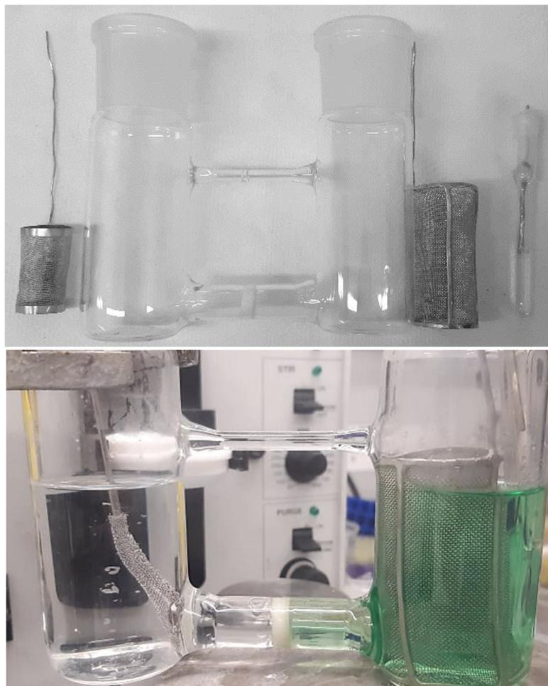
**Figure S1.** H-cell electrolysis before set-up (top) and during electrolysis (bottom). The green colour of  $[\text{Cu}(\text{Me}_6\text{tren})(\text{CH}_2\text{CN})]^+$  is apparent in the working electrode chamber (right).
