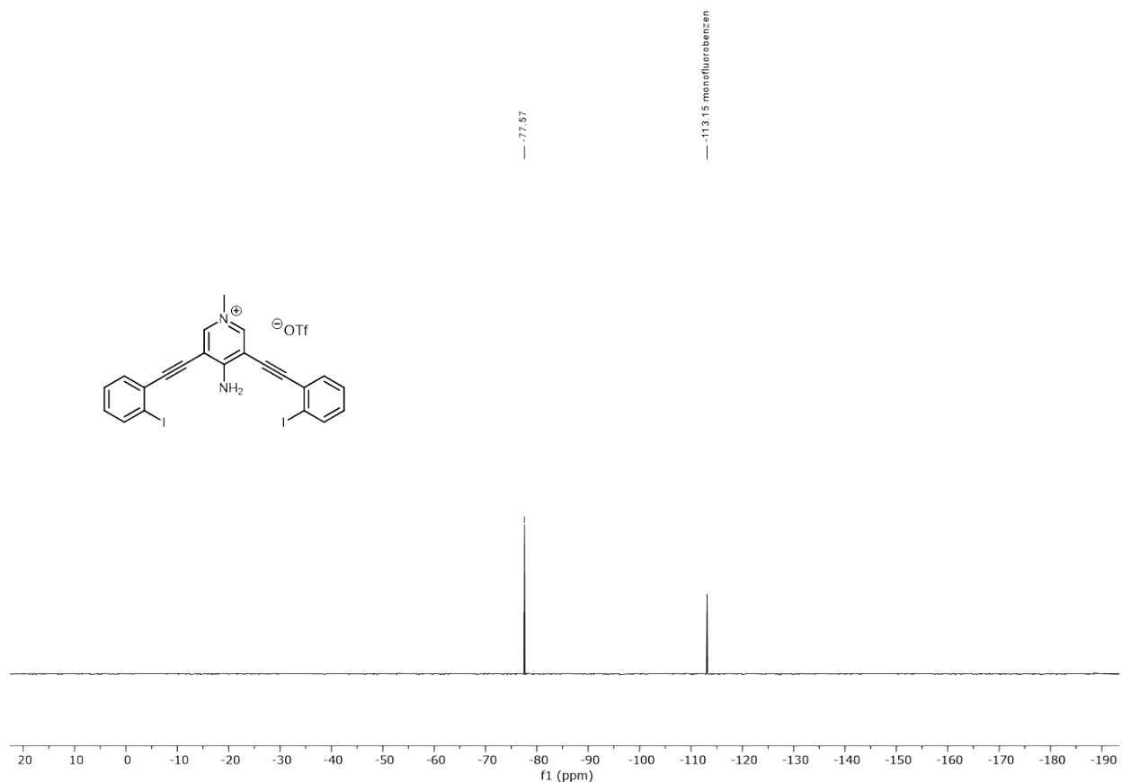
Figure 33S ^{19}\text{F} NMR spectrum of 4 (470 MHz, \text{CD}_3\text{CN} ). \text{C}_6\text{H}_5\text{F} (monofluorobenzene) internal reference.
