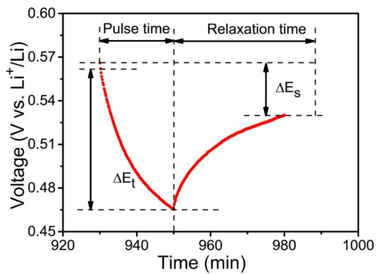
**Fig. S5** E vs. t profiles for the GITT measurement.
