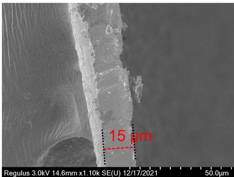
**Fig. S6** SEM cross-section image of the VB4/rGO electrode.
