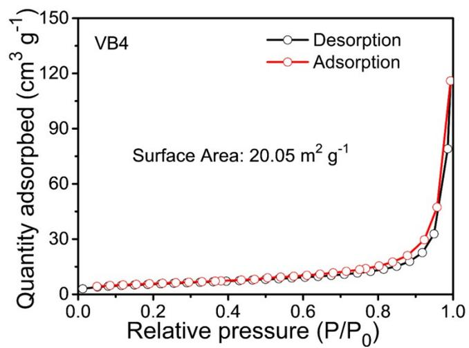
**Fig. S3** N<sub>2</sub> adsorption/desorption isotherms of the pristine VB4.
