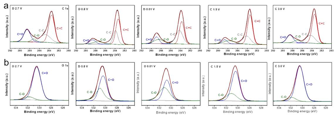
**Fig. S7** The ex-situ XPS spectra of VB4/rGO anode under different charge/discharge states: (a) C 1s and (b) O 1s.
