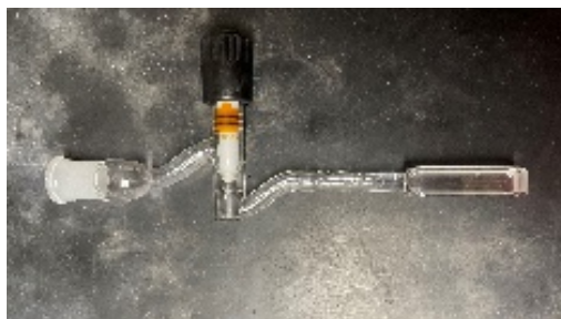
Figure S2. 10 mm pathlength quartz cell fused with a J-Young valve used for collecting photophysical data of all air sensitive compounds.
