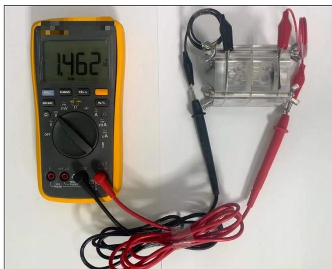
**Fig. S9.** The open circuit voltage of the Pt/C-IrO<sub>2</sub>-catalyzed battery.
