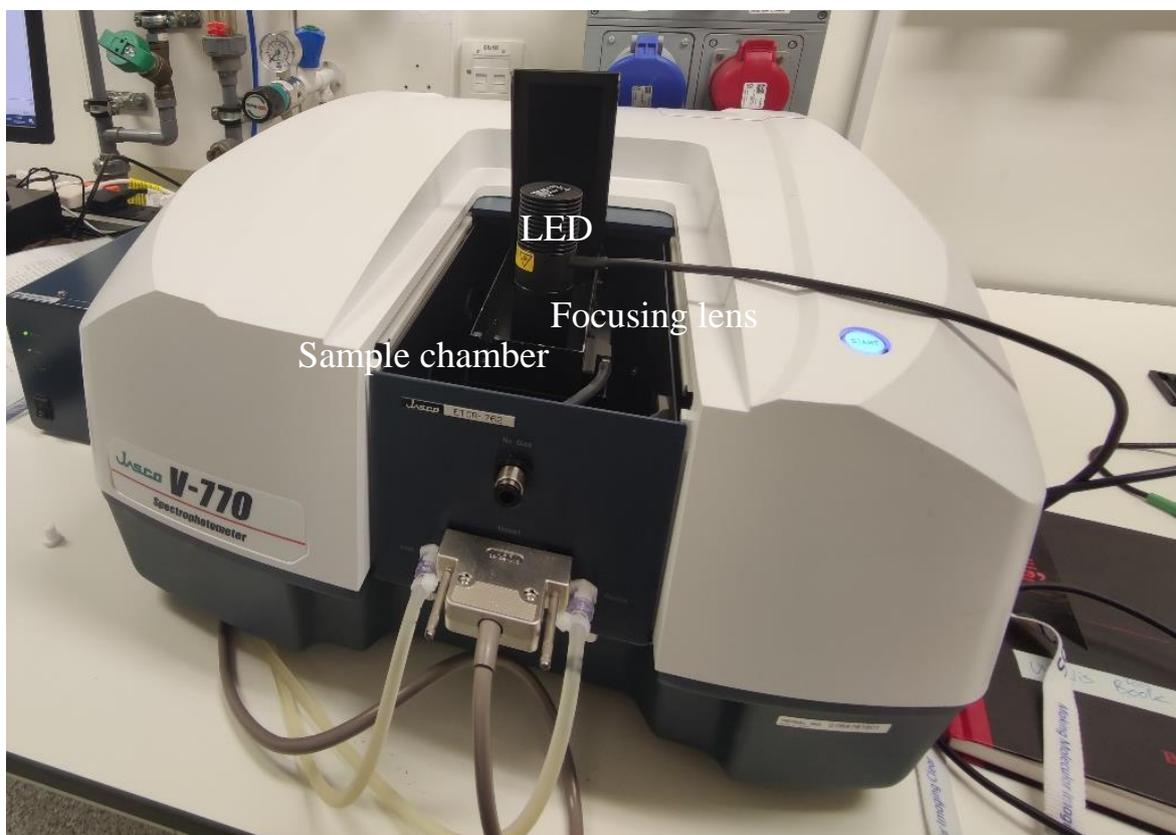
**Figure 307:** Experimental setup for in-situ switching
