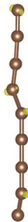
Figure S6. The charge densities distribution of a kinked carbyne chain. The charge densities distribution: the charge density is nonuniform. The kink bonds induce the nonuniform distribution of charge density and it is mainly concentrated at the twisted carbon atoms.
