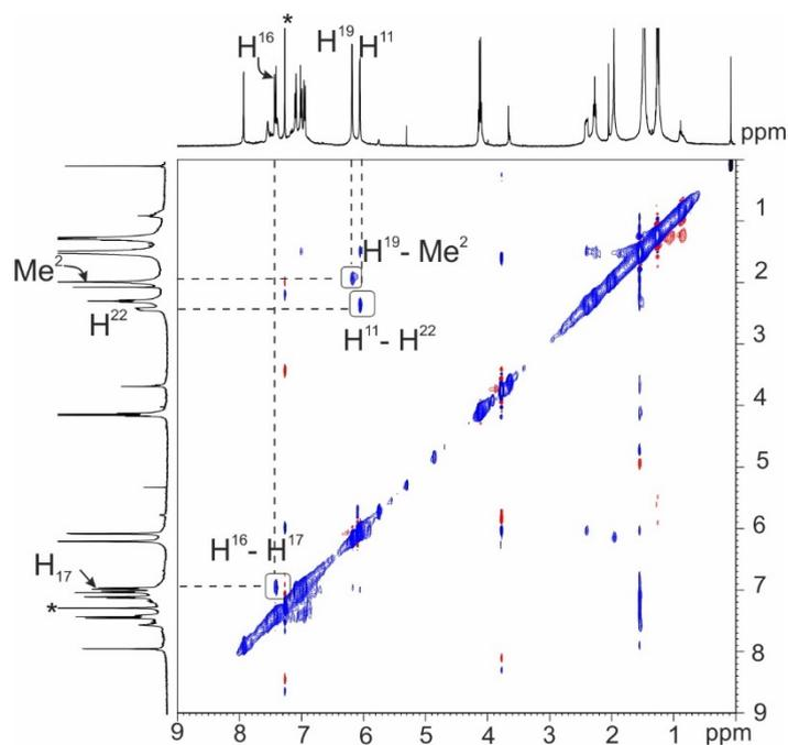
**Figure S 22.** 2D NOESY NMR (400 MHz, at 298 K, CDCl<sub>3</sub>, mixing time = 0.3 s) of a solution containing tetra-imine cage (CDCl<sub>3</sub>)<sub>2</sub>·**1b**. See **Scheme S 1** for protons assignment. (\*) Indicates residual solvents.
