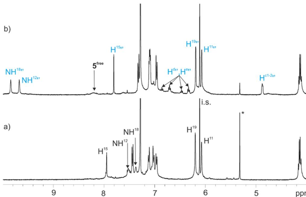
**Figure S 32.** Selected  $^1\text{H}$  NMR region of spectra (400 MHz, at 298 K,  $\text{CDCl}_3$ ) of a solution containing tetra-imine cage solvate  $(\text{CDCl}_3)_2$  before (a) and immediately after addition of **5** (3 equiv.) (b). Primed and blue letters indicate the bound host and guest in a 2:1 stoichiometry. See **Scheme S 2** for protons assignment. (\*) Indicates residual solvents. i.s. internal standard.
