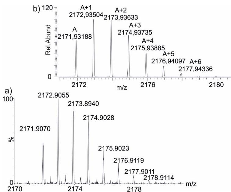
**Figure S 39.** Experimental (a) and calculated (b) isotopic distributions of cage complex  $[4c-1b + Cl]^-$ . The exact mass for the monoisotopic peak is indicated as A in (b).
