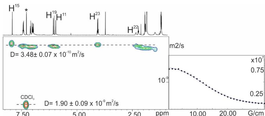
**Figure S 17.**  $^1\text{H}$  pseudo-2D plot of the DOSY NMR (400 MHz, at 298 K,  $\text{CDCl}_3$ : $\text{CD}_3\text{CN}$  9:1 mixture,  $D_{20} = 0.1$  s,  $P_{30} = 0.002$  s) of tetra-imine cage  $(\text{CD}_3\text{CN})_2\text{1b}$ . See **Scheme S 1** for protons assignment (\*) Indicates residual solvents.
