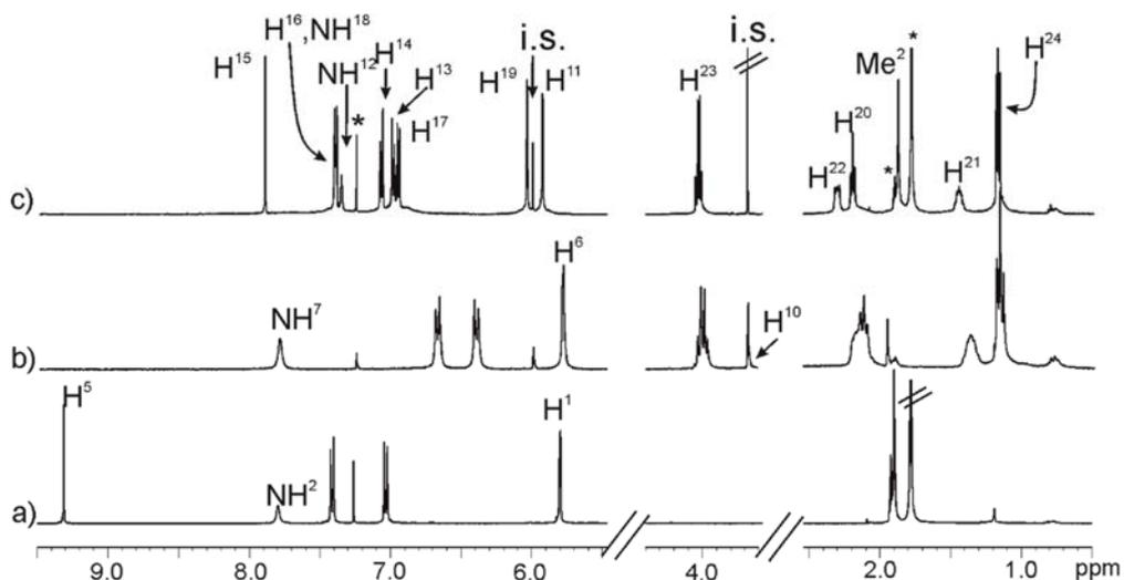
**Figure S 12.** Selected regions of  $^1\text{H}$  NMR spectra (400 MHz, at 298 K,  $\text{CDCl}_3:\text{CD}_3\text{CN } 9:1$  mixture) of (a) **3**, (b) **2b**, (c) an equimolar mixture of **3** and **2b** after 3h at r.t. (tetra-imine cage  $(\text{CD}_3\text{CN})_2<1\text{b}$ ). See **Scheme S 1** for protons assignment. (\*) Indicates the residual solvents.
