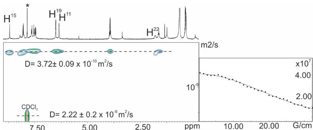
**Figure S 23.** <sup>1</sup>H pseudo-2D plot of the DOSY NMR (400 MHz, at 298 K, CDCl<sub>3</sub>, D20 = 0.15 s, P30 = 0.001 s) of a solution containing tetra-imine capsule (CDCl<sub>3</sub>)<sub>2</sub>·**1b**. See **Scheme S 1** for protons assignment. (\*) Indicates residual solvents.
