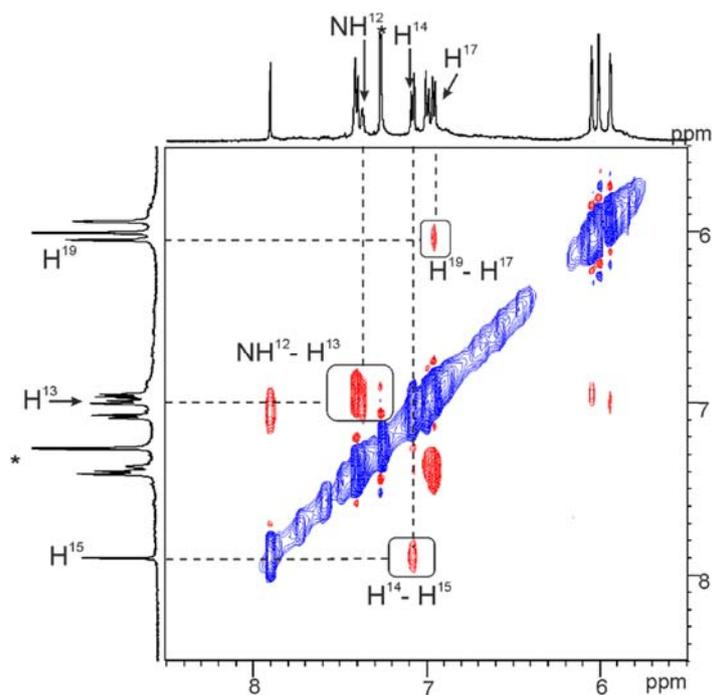
**Figure S 16.** Selected region of 2D ROESY NMR (400 MHz, at 298 K,  $\text{CDCl}_3$ : $\text{CD}_3\text{CN}$  9:1 mixture, mixing time = 0.3 s) of tetra-imine cage  $(\text{CD}_3\text{CN})_2\text{1b}$ . See **Scheme S 1** for protons assignment. (\*) Indicates residual solvents.
