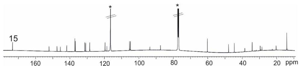
**Figure S 13.**  $^{13}\text{C}$  NMR (120 MHz with cryoprobe, 298 K,  $\text{CDCl}_3:\text{CD}_3\text{CN}$  9:1 mixture) of a solution containing tetra-imine cage  $(\text{CD}_3\text{CN})_2\text{-1b}$ . Imine carbon is indicated as 15. (\*) Indicates residual solvents.
