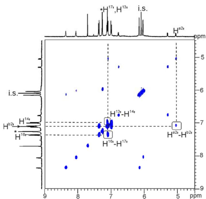
**Figure S 7.** Selected region of the 2D COSY NMR (400 MHz, at 298 K, CDCl<sub>3</sub>) of a solution containing tetra-imine cage complex **4c1b**. See **Figure S 5** for protons assignment. (\*) Indicates the residual solvents.
