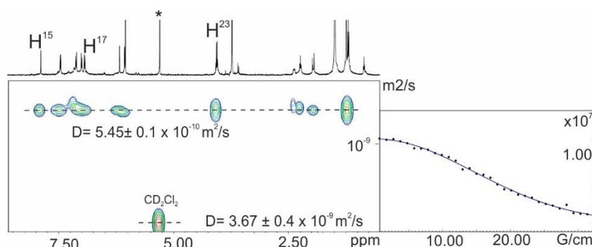
**Figure S 28.**  $^1\text{H}$  pseudo-2D plot of the DOSY NMR (400 MHz, at 298 K,  $\text{CD}_2\text{Cl}_2$ ,  $D_{20} = 0.15$  s,  $P_{30} = 0.001$  s) of a solution containing tetra-imine cage  $(\text{CD}_2\text{Cl}_2)_2\text{c1b}$ . See **Scheme S 1** for protons assignment. (\*) Indicates residual solvents.
