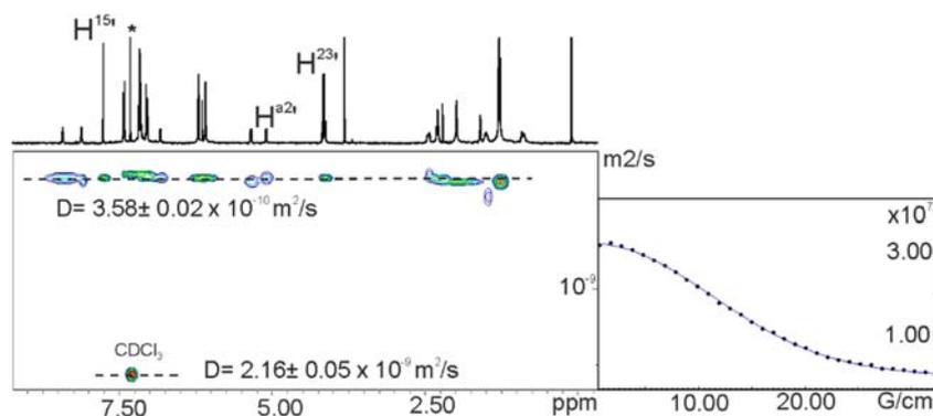
**Figure S 10.**  $^1\text{H}$  pseudo-2D plot of the DOSY NMR (400 MHz, at 298 K,  $\text{CDCl}_3$ ,  $D_{20} = 0.1$  s,  $P_{30} = 0.002$  s) of a solution containing tetra-imine cage complex **4c1b**. See **Figure S 5** for protons assignment. (\*) Indicates the residual solvents.
