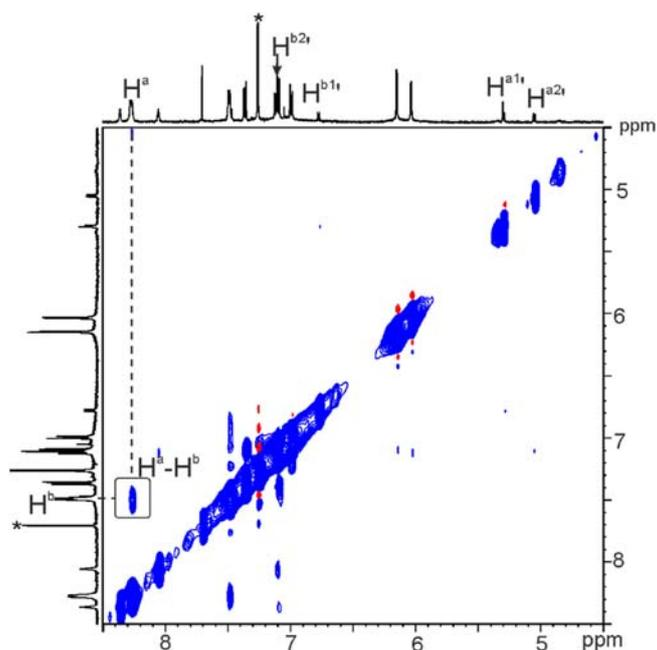
**Figure S 31.** Selected region of the  $^1\text{H}$ - $^1\text{H}$ -EXSY NMR (400 MHz,  $\text{CDCl}_3$ , 298 K, mixing time = 0.3 s) of a solution containing tetra-imine cage complex **4** in the presence of an excess of **4** (2 equiv.). The spectrum does not show cross-peaks between free and bound guest. This is indicative of a slow chemical exchange process between free and bound guest on the EXSY NMR timescale. See **Scheme S 2** for protons assignment. (\*) Indicates residual solvents.
