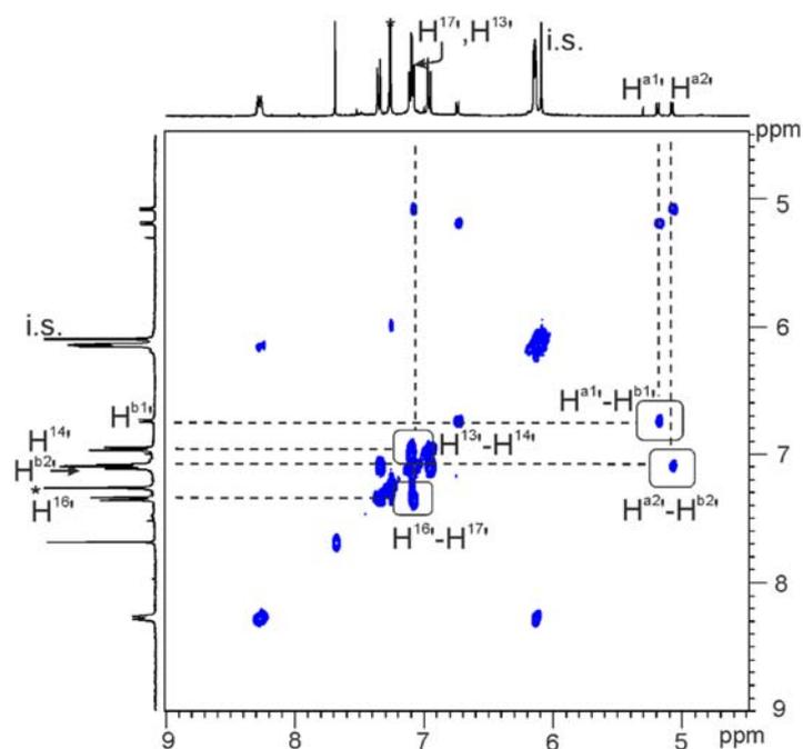
**Figure S 2.** Selected region of 2D COSY NMR (400 MHz, at 298 K, CDCl<sub>3</sub>) of a solution containing tetra-imine cage complex **4c1a**. See Figure S 1 for protons assignment. (\*) Indicates residual solvents.
