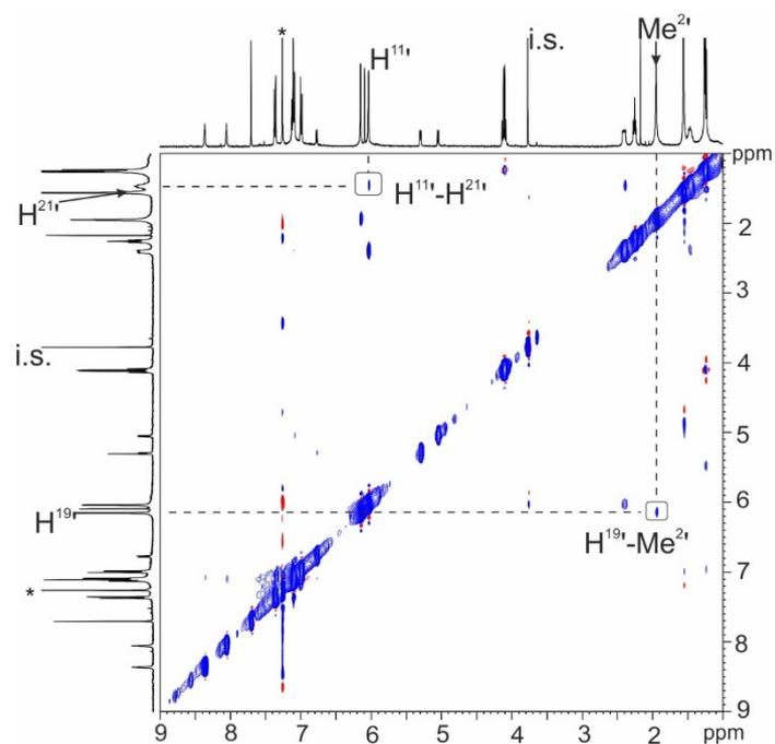
**Figure S 8.** 2D NOESY NMR (400 MHz, at 298 K,  $\text{CDCl}_3$ , mixing time = 0.3 s) of a solution containing tetra-imine cage complex **4c1b**. See **Figure S 5** for protons assignment. (\*) Indicates the residual solvents.
