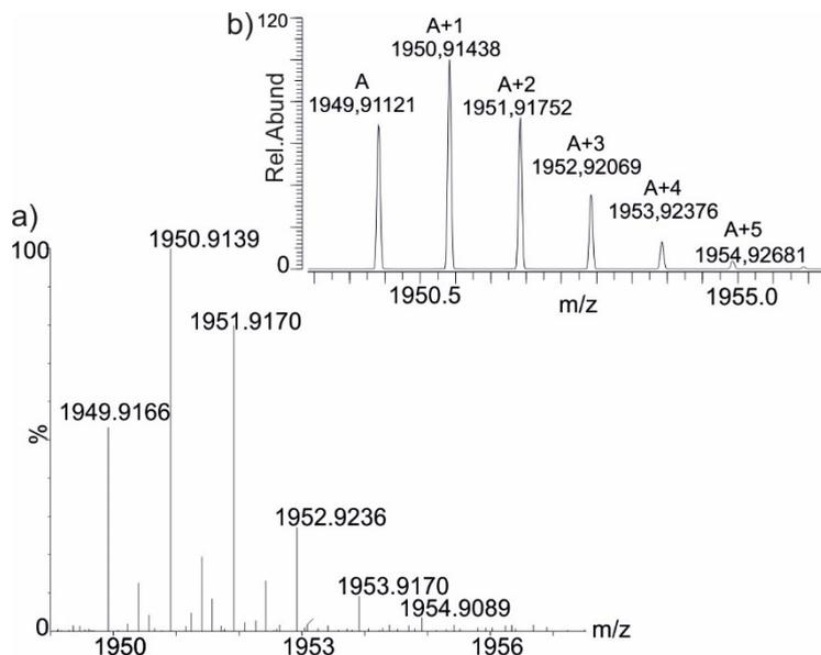
**Figure S 38.** Experimental (a) and calculated (b) isotopic distributions of cage  $[1b+H]^+$ . The exact mass for the monoisotopic peak is indicated as A in (b).
