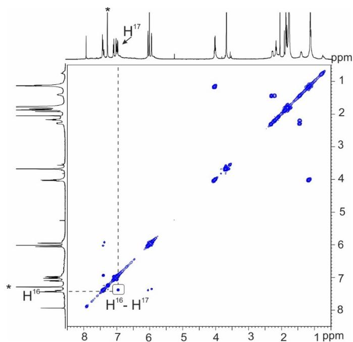
**Figure S 14.** 2D COSY NMR (400 MHz, at 298 K,  $\text{CDCl}_3:\text{CD}_3\text{CN}$  9:1 mixture) of a solution containing tetra-imine cage  $(\text{CD}_3\text{CN})_2\text{-1b}$ . See for **Scheme S 1** protons assignment. (\*) Indicates residual solvents.
