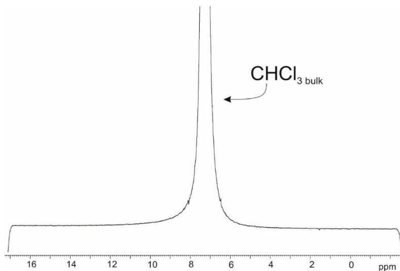
**Figure S 24.** GOESY NMR experiment (500 MHz, at 298 K) using a 95:5  $\text{CHCl}_3$ : $\text{CDCl}_3$  solution of cage **1b** with selective excitation of the signal of chloroform at 7.28 ppm. The absence of exchange peaks suggests that most likely, the chemical exchange between the free and bound  $\text{CHCl}_3$  was fast on the chemical shift timescale.
