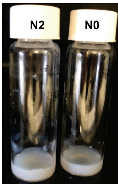
Figure S11. Picture of PI and P(I-co-DOT) nanoparticles obtained by nanoprecipitation from N0 and N2 , respectively (see Table 2).
